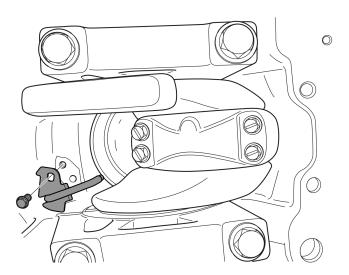
3 Remove the piston cooling nozzle.
