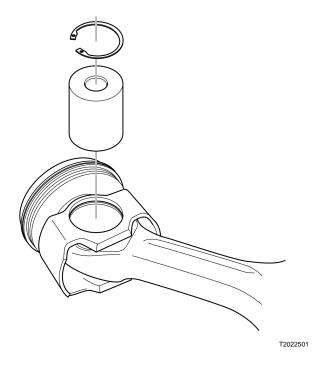
Remove the snap ring from the piston and push out the piston pin. Remove the piston from the connecting rod.
