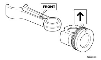
Install the connecting rod in the piston with the marking "FRONT" on the connecting rod and the arrow on the piston facing the same direction.
