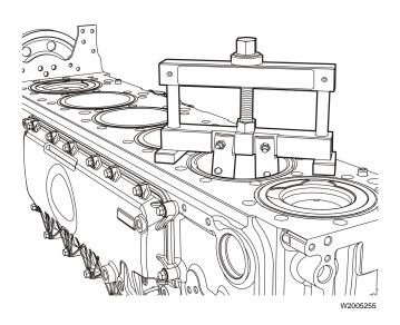
Pull the cylinder liner out of the block.
