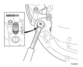
Remove the plug from the flywheel housing and install tool 88800014. Turn the crankshaft until it is possible to get at the bolts on the connecting rod that is to be removed.
