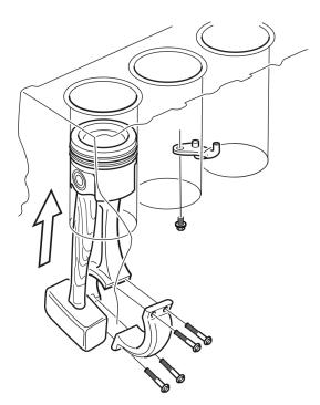
Remove the piston and the connecting rod.
