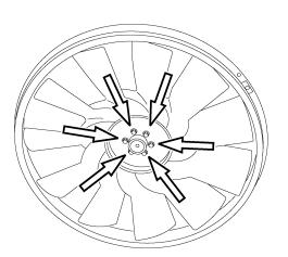
Position the engine fan blade on the front of the fan hub and install the fan blade fasteners. Tighten all fasteners to specification.
