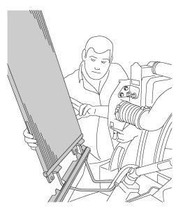
Remove upper hose clamps on the left side of the cooler. Remove the upper coolant hoses from the thermostat housing (including pipe). Remove bracket bolts from the cylinder head.
