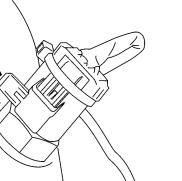
Install the air temperature sensor connector to the sensor. Insert the connector lock tab, push in place and secure with a tie strap. Install the P-clamp to secure the harness to the main fresh air pipe. Torque-tighten the P-clamp bolt to  $8 \pm 1.2 \text{ Nm } (6 \pm 1 \text{ ft-lb}).$
