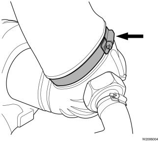
17 Install the main fresh air pipe to the turbocharger inlet elbow. Tighten the clamps to secure the pipe and then connect the air compressor hose to the pipe.
