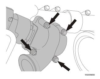
21 Remove all the EGR valve mounting bolts and remove the valve from the exhaust manifold. Discard the mounting bolts.
