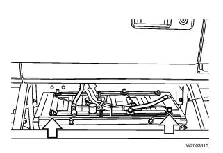
3 Remove inner splash guard as an assembly.
