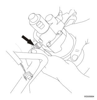
Remove the return oil line from the bottom of the EGR valve.
