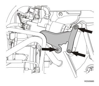
Remove the nuts and bolts securing the EGR valve heat shield and remove the shield.
