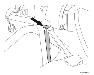
6 Tighten the return oil line to specification.
