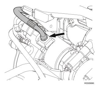
20 Remove the inlet oil line from the EGR valve.
