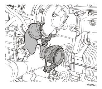
Remove the EGR hot pipe from between the EGR valve and the EGR cooler.
