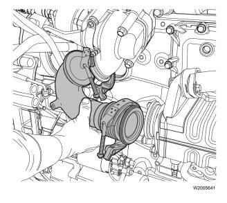
Inspect and lubricate the V-clamps. Hook the upper V-clamp over the EGR valve flange. Place the lower V-clamp over the bellows on the hot pipe.
