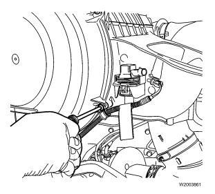
Install the filter restriction gauge wiring harness to the air filter housing and tighten the clamps.
