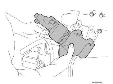
1 Position the EGR valve near the exhaust manifold EGR ports.
