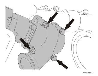
4 Install the other two new EGR valve bolts. Torque-tighten all EGR valve bolts to 61 Nm (45 ft-lb).
