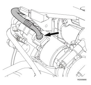
**5** Install the inlet oil line to the EGR valve and tighten to specification.
