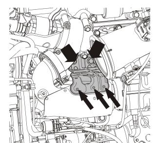
Position the upper EGR hot pipe heat shield and install the fasteners and bolts. Tighten the fasteners to specification.
