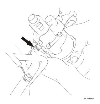
2 Install the return oil line to the bottom of the EGR valve. Allow the fitting to remain only finger tight at this time.
