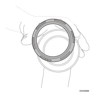
Remove the high temperature gaskets from the EGR valve end of the hot pipe and the EGR cooler end of the hot pipe. Discard the gaskets.
