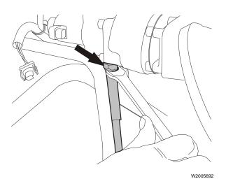
Loosen both the inlet and the return oil line fittings on the valve.
