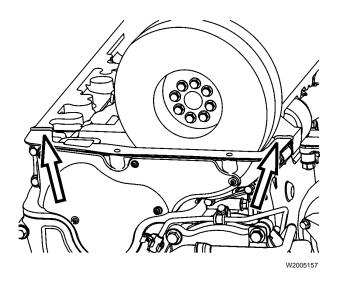
Apply a two mm (0.08 inch) bead of Volvo sealant across the parting line on the valve cover sealing surface between the timing gear cover and the cylinder head.
