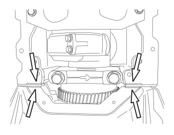
Apply a two mm (0.08 inch) bead of Volvo sealant to the seams between the flywheel housing and timing gear mounting plate and between the timing gear mounting plate and the cylinder block.
