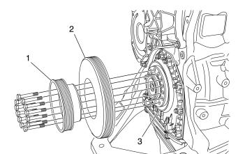
Attach the vibration damper (2), belt pulley (1) and bolts to the crankshaft hub and torque-tighten according to "Specifications", see Group 20.
