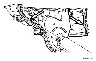
Apply Volvo sealant to the mating surfaces of the timing gear cover; see "Specifications", Group 20.
