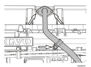
Remove the fasteners securing the valve cover to the cylinder head. Also remove the engine wiring harness support bracket from the front of the valve cover.
