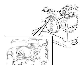
Make sure that the camshaft and flywheel are positioned at top dead center (TDC).
