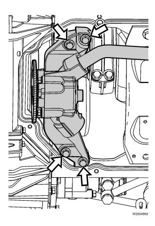
Remove the oil strainer and suction pipe from the oil pump.
