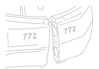
When installing connecting rod bearing caps, align the markings on the connecting rod and bearing cap.
