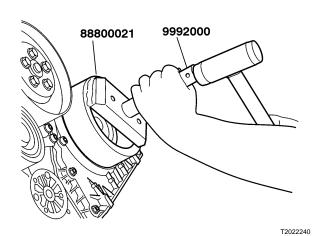
Place the crankshaft cover with the spacer 9998170 in the center on a flat surface. Install a new crankshaft seal with plastic ring in the crankshaft cover. The spacer ring prevents the plastic ring from sliding off. Carefully tap the crankshaft seal into the crankshaft cover with drift 88800021 and handle 9992000 until the crankshaft seal is level with the crankshaft cover outer surface.
