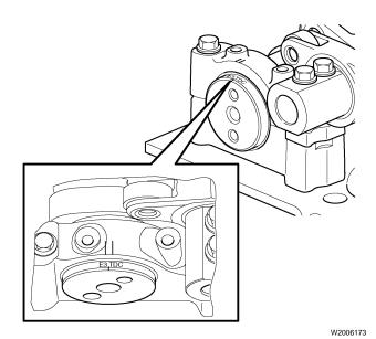
Apply a film of oil to the crankshaft gear inner surface and to the crankshaft rear journal. Install the crankshaft gear and bolts. Torque-tighten as specified in "Specifications", see Group 20.
