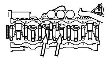
Rotate the crankshaft so that the No. 3 and No. 4 pistons are near bottom dead center (BDC) so that the connecting rod bearing cap bolts can be accessed. Remove the connecting rod bearing cap bolts and caps. Remove the connecting rod bearings from the connecting rods and bearing caps.
