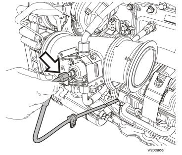
Connect the aftertreatment injector fuel supply line. Tighten the fuel line fitting to  $15 \pm 0.5$  Nm  $(135 \pm 5 \text{ in-lb})$ .
