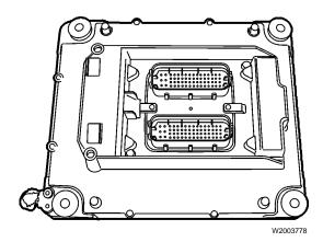
This information covers the proper procedure for replacement of the Engine Electronic Control Unit (EECU) on the Volvo D13F engine.
