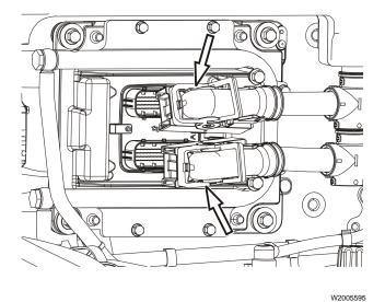
Push the connector locks inward and rotate outward to disconnect both wiring harnesses from the EECU.
