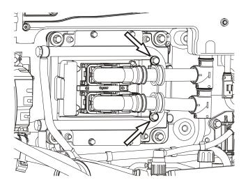
Install the bolts to secure the wiring harness clamps to the EECU.
