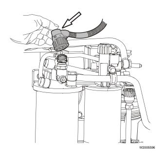
4 Disengage the fuel sensor harness connector from the fuel filter housing.
