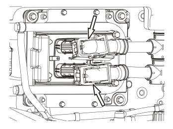
5 Carefully engage the upper and lower wiring harness connectors to the EECU. Verify that the connectors are latched and properly locked in position.
