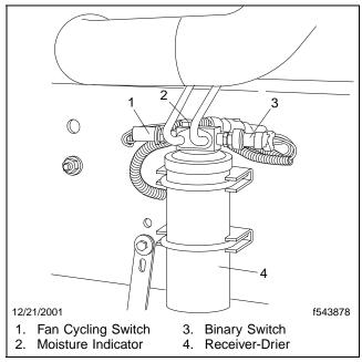
Fig. 1, Receiver-Drier
