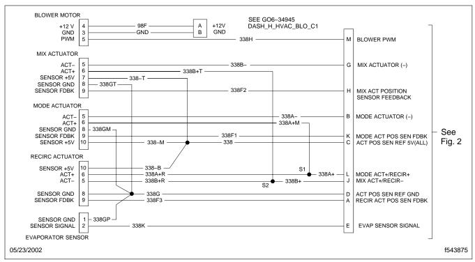
Fig. 1, HVAC Wiring Diagram, Part 1
