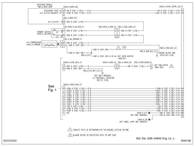
Fig. 2, HVAC Wiring Diagram, Part 2
