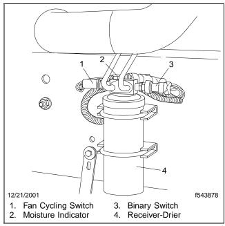
Fig. 1, Receiver-Drier
