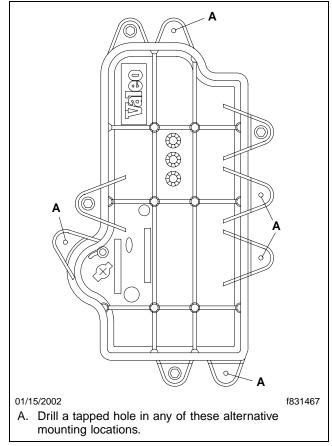
Fig. 3, Evaporator Service Cover
