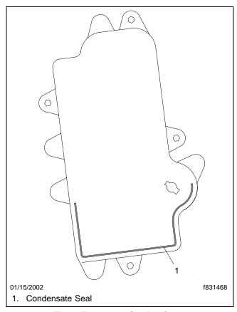
Fig. 2, Evaporator Service Cover
