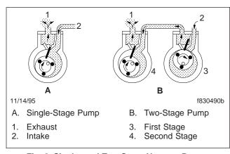
Fig. 2, Single- and Two-Stage Vacuum Pumps
