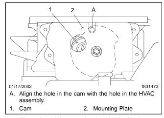
Fig. 2, Cam Alignment for the Air Distribution Actuator
