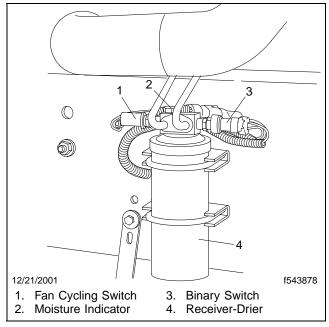
Fig. 1, Receiver-Drier
