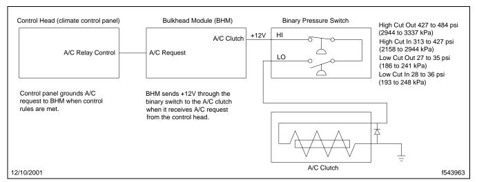
Fig. 3, A/C Clutch Control Circuit
