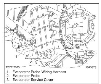
Fig. 1, Evaporator Probe and Service Cover
