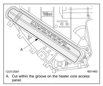
Fig. 3, Heater Core Access Panel
