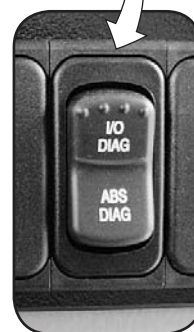
Diagnostic Mode Switch Cycles the MBC's display through Ports, Inputs, Outputs, and Feedbacks. (3-position momentary)
