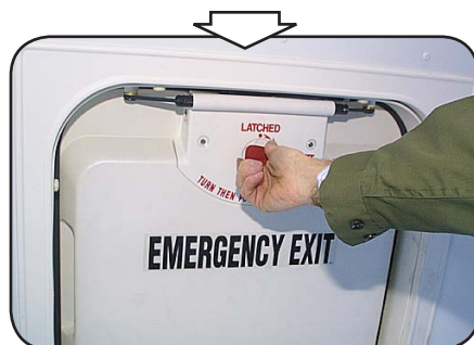
Rotate the red knob from the position marked "LATCHED" to the position marked "TO EXIT."
