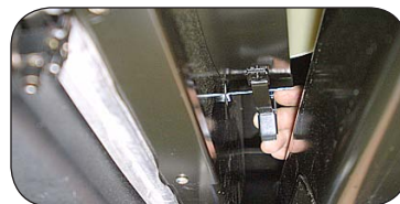
(Viewed from under the radiator.) On buses with pivoting radiators, a clasp on the right side of the fan shroud allows it to expand to provide clearance from the fan blades when the radiator is pivoted.
