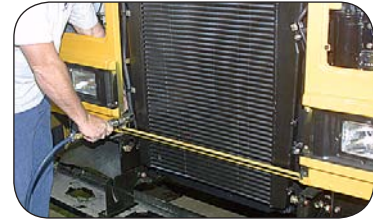
Remove 4 bolts, washers, nuts from crossbar.
