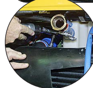
Disconnect radiator hoses after draining. Not necessary on buses equipped with pivot radiator feature.
