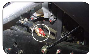
Rear Engine heater return cutoff valve. Accessible from under the bus, forward of the radiator.
