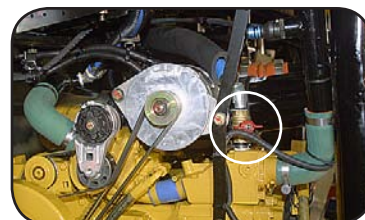
Rear Engine (Cat C7 shown) heater supply cutoff valve. Accessible from engine compartment.
