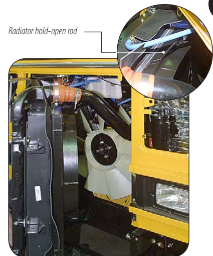
Pivoted radiator provides engine front access without draining coolant.
