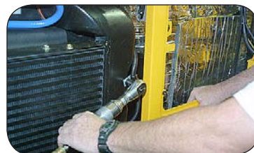
Remove the harness clamps from the radiator and push the harness out of the way.
