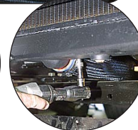
Disconnect radiator hoses after draining. Not necessary on buses equipped with pivot radiator feature.
