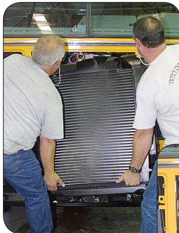
Obtain assistance in lifting out non-pivoting radiator.
