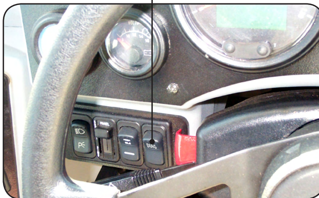
Diagnostic Mode Switch Cycles the MBC's display through Ports, Inputs, Outputs, and Feedbacks.
