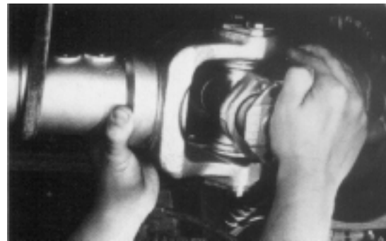
Figure 46—Bearing Assembly Flush to Face of Yoke
