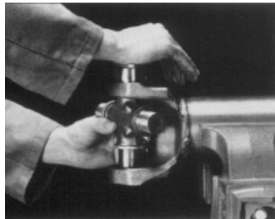
Figure 37—Bearing Assembly Flush With Face of Yoke
