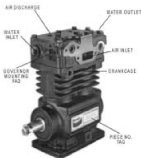
Figure 15B—Air Compressor Major Assemblies
