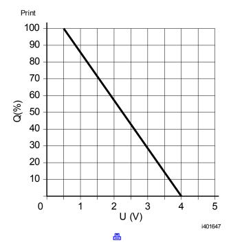
Q Tank volumeV Signal voltage
