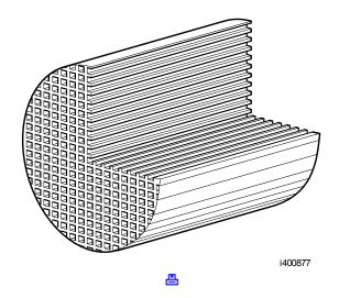
A carrier material (2) that holds the active catalytic agent (3) is applied to the element (1). The catalytic agent for the DOC is platinum. The surface of the carrier material is very rough and porous, so the effective area through which the exhaust gas flows is very large.
