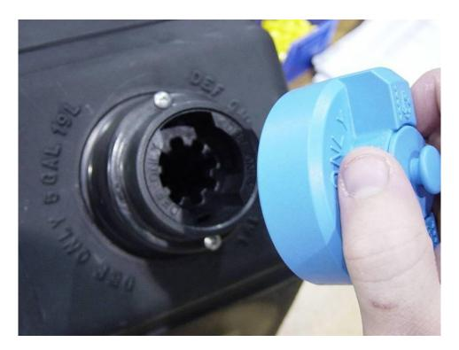
8) Wipe down the fill port adapter with a damp cloth before replacement of the cap. Take the cap and replace with the grooves on the cap fitting into the notches on the fill port adapter.
