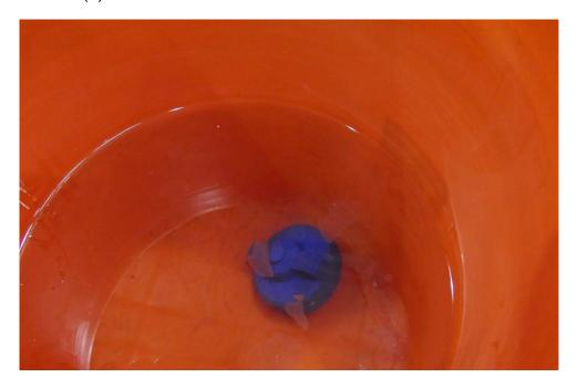
5) After soaking, grip the cap and shake vigorously while underwater to break up and loose and/or remaining DEF within the cap assembly.
