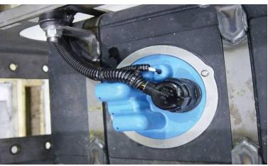
Using a 1/8" Allen wrench/hex key, unscrew the Allen screws holding the retaining ring to the reservoir from the unit and place safely aside to be used at a later time.
