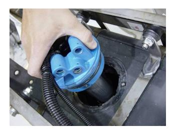
4. Once loosened from the DEF reservoir, pull the head unit out of the tank, angling the head unit towards the flange at the end so that it will fit through the opening, and drain the head unit of any coolant still inside. Place the head unit upside-down on a soft, clean surface, this helps prevent against the introduction of contaminants upon re-installation.
