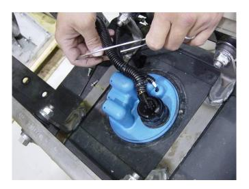
17. Using the Allen Wrench/Hex Key, screw the Allen screws back into place and installation is complete. Recommended torque installation is 20-30 in-lbs.
