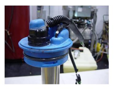
7. Snip off the zip ties to remove the split wire loom from the wires connected to the sensor.
