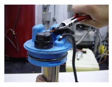
8. Remove split wire loom from around the wires connected to the sensor unit.
