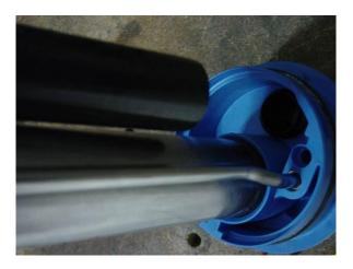
6. Place the head unit upright on a clean surface, so as to help prevent contaminants from being introduced into the reservoir upon re-installation.
