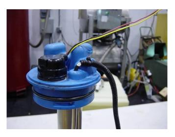
9. Use groove lock pliers or a wrench to firmly grip the base of the sensor and turn it counter clockwise to loosen it from the head unit.
