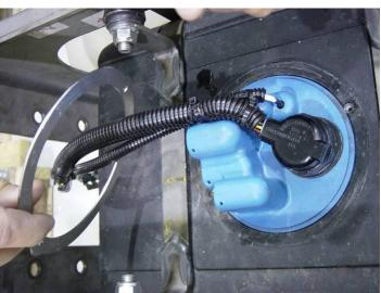
3. Using a flathead screwdriver, gently pry around where the head unit is connected to the reservoir while pulling on the top of the unit to remove. Do NOT pull on the wires or fittings for removal.
