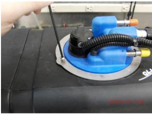
2. Remove the stainless steel retaining ring from the unit.
