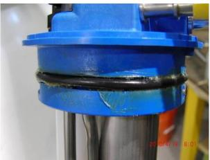
7. Utilizing the same caution as earlier, position the new DEF Multifunction Head Unit over the reservoir. Angle the head units so that it will fit through the opening, then straighten the head unit and slide it into the reservoir.
