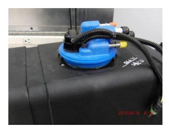
8. Orient the head unit to the desired position or as required so that the fittings are aligned correctly with the hose routing in the DEF system and push the head unit back into place. Add a few drops of Loctite 242 to the threaded screw holes on the reservoir.
