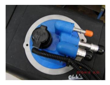
10. Using the Allen Wrench/Hex Key, screw the Allen screws back into place clockwise with a max torque of 20-30 in-lbs and installation is complete.
