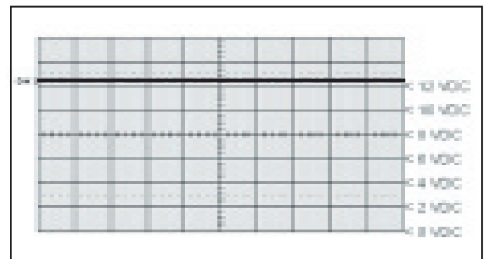
FIGURE 6 - POWER LINE WITHOUT PLC SIGNAL
