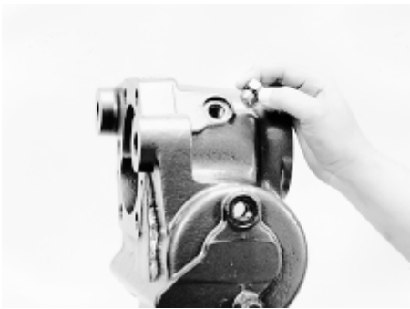
Replace automatic bleed screw, and aux. port plugs
