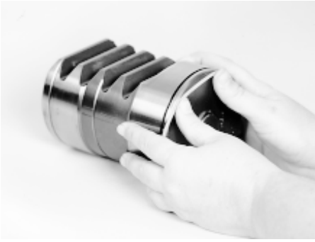
Install rack piston o-ring and seal ring
