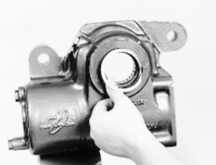
Install retaining ring
