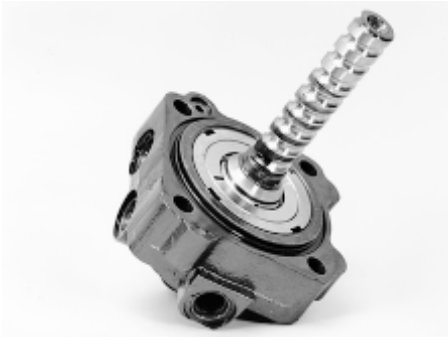
Inspect input shaft, valve/worm assembly sealing areas
