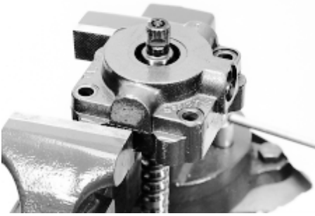
Reposition subassembly in vise
