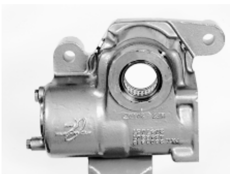
Inspect housing screws, and plugs
