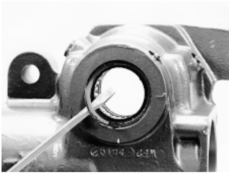
Remove retaining ring (if equipped)
