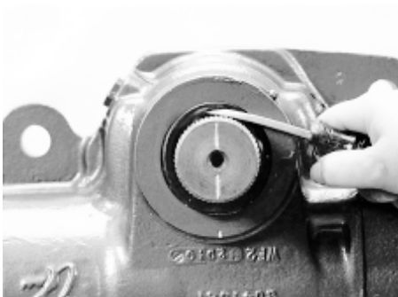
Remove dirt & water seal
