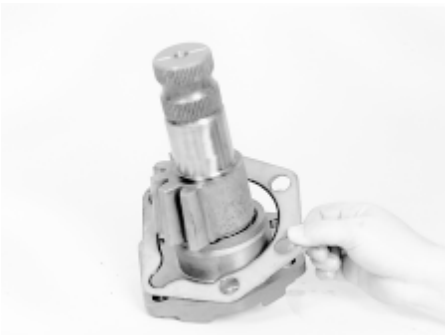
Install side cover gasket
