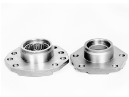
Inspect side cover bushing/bearing
