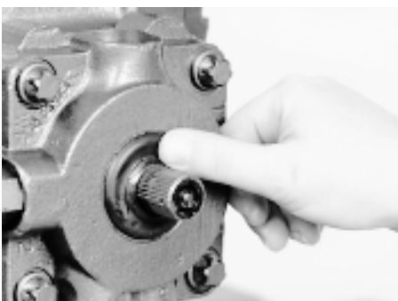
Install dirt & water seal
