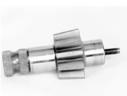
Inspect sector shaft assembly
