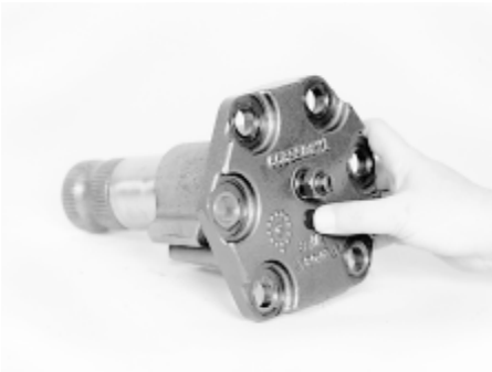
Assemble vent plug
