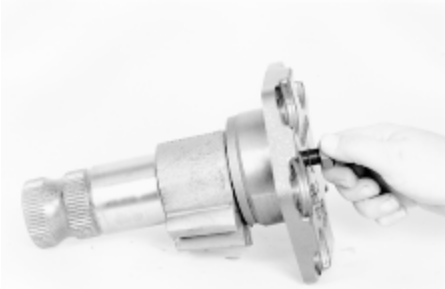
Install jam nut
