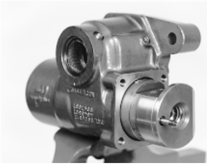
Position rack piston in housing
