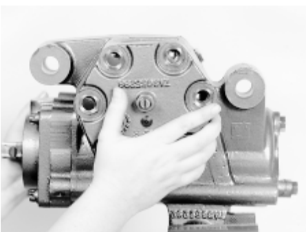
Install sector shaft and side cover into housing
