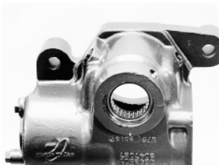
Inspect roller bearing
