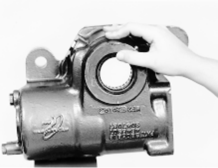
Install dirt seal
