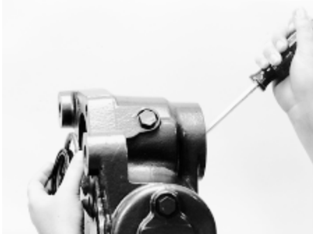
Remove pressure seal (and spacer washer if equipped)
