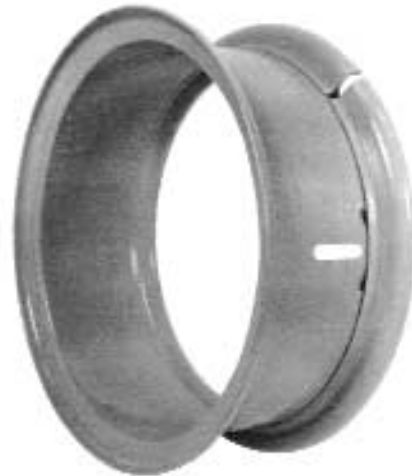
Tube-Type Demountable Rim Assembly (multi-piece)
