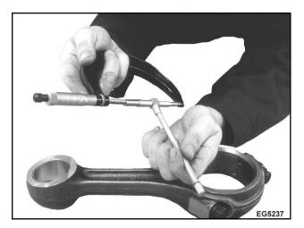
Figure 465 Connecting rod bearing bore taper measurement
