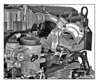
Figure 83 Intake throttle assembly
