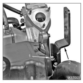
Figure 151 Tube support bracket
