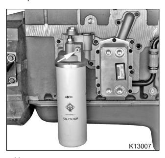
Figure 270 M12 plug assembly
