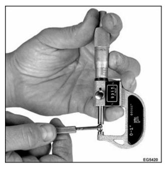
Figure 371 Measure Ball gauge with micrometer
