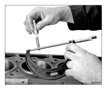
Figure 470 Telescoping gauge measurement
