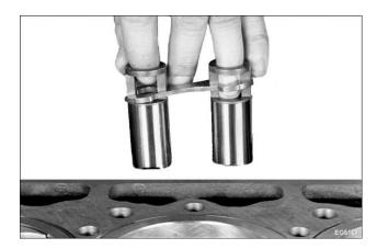
Figure 353 Roller tappets and guide
