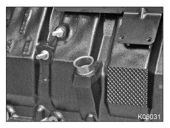
Figure 542 Oil level gauge tube
