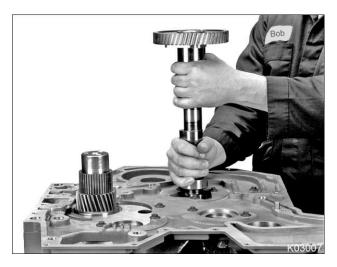
Figure 524 Camshaft assembly installation
