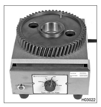
Figure 526 Camshaft gear and hot plate
