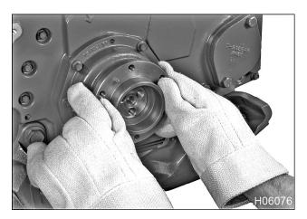
Figure 326 Damper hub installation
