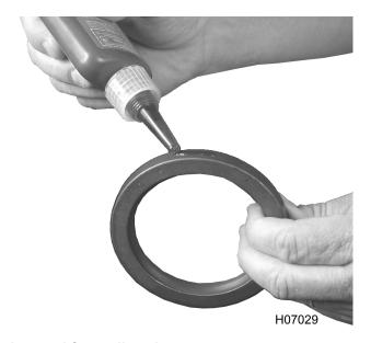
Figure 319 Hydraulic sealant and front oil seal
