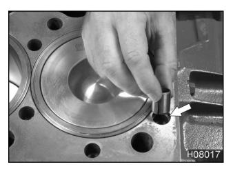
Figure 402 Cylinder head alignment dowel
