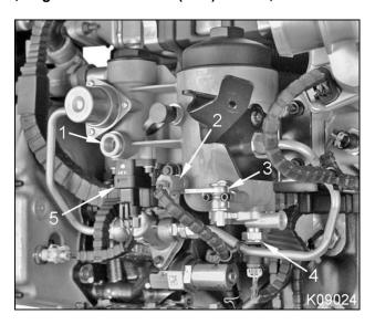
Figure 78 Fuel filter header assembly
