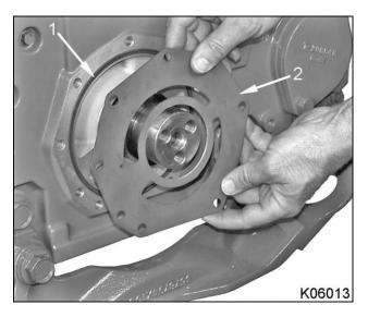
Figure 317 Oil pump housing plate and seal
