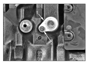
Figure 503 Coolant heater (intake side of crankcase)
