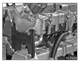
Figure 140 EGR valve manifold support
