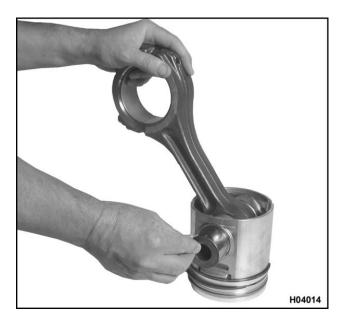
Figure 487 Piston pin installation (typical)
