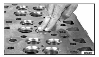
Figure 380 Turn valve on valve seat
