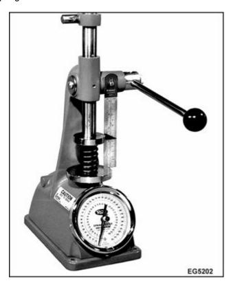
Figure 393 Measure valve spring tension
