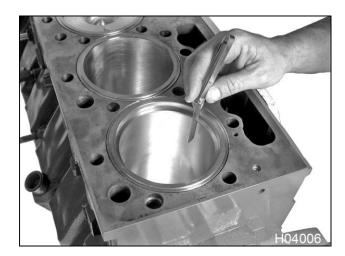
Figure 461 Piston ring end gap measurement
