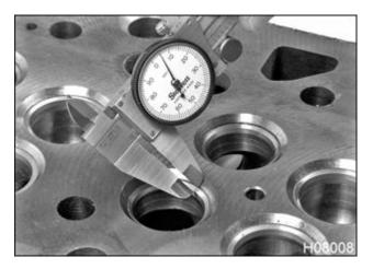
Figure 383 Valve seat width measurement
