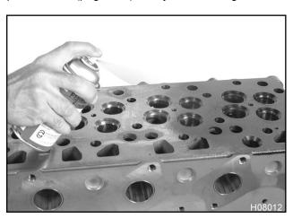
Figure 362 Spray dye penetrant on cylinder head
