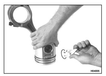
Figure 488 Piston pin retaining ring installation (typical)
