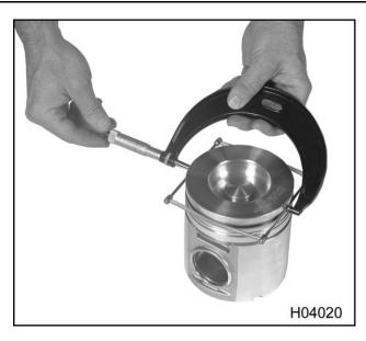
Figure 458 Piston ring groove measurement (top / keystone cross section)
