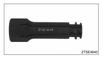
Figure 560 Valve Seat Remover (collet), ZTSE4640
