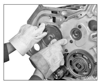
Figure 527 Camshaft gear installation
