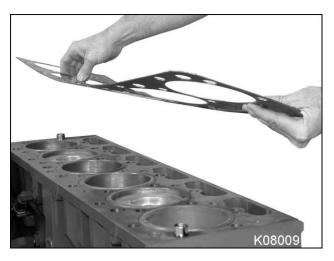
Figure 404 Cylinder head gasket and alignment dowels
