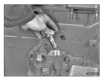
Figure 264 Thermal valve installation
