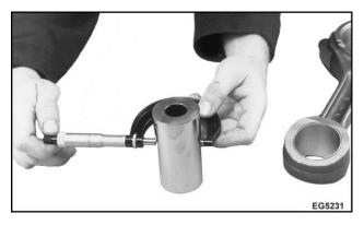
Figure 462 Piston pin measurement
