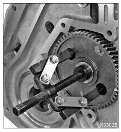
Figure 510 Camshaft gear and Cam Gear Puller
