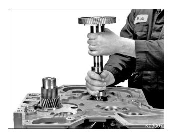
Figure 512 Camshaft assembly removal
