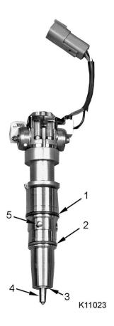
Figure 194 Fuel Injector assembly
