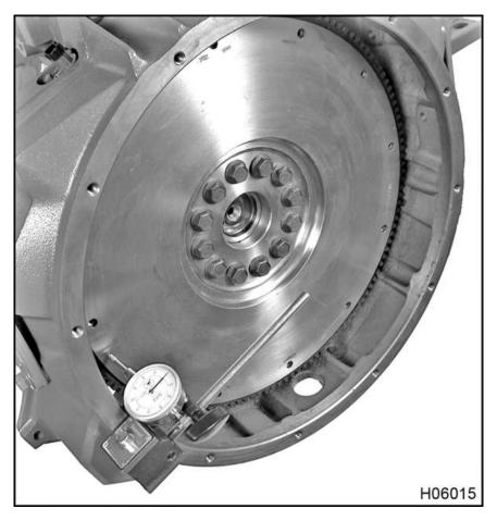
Figure 433 Flywheel surface runout measurement
