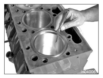
Figure 472 Measure cylinder sleeve piston ring end gap
