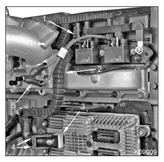
Figure 88 Injector wiring harness
