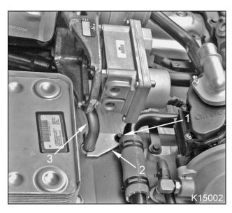
Figure 123 Turbocharger oil drain tube, bracket, and bolt
