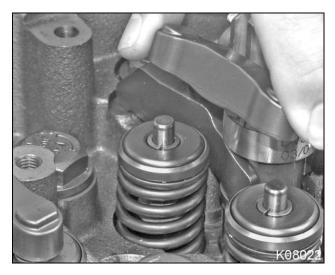
Figure 413 Valve bridge installation
