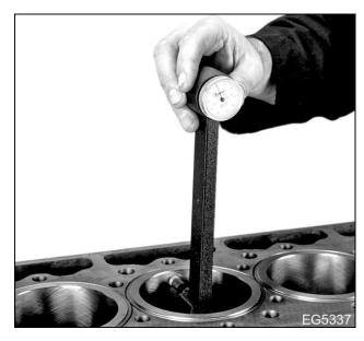
Figure 471 Cylinder sleeve taper measurement
