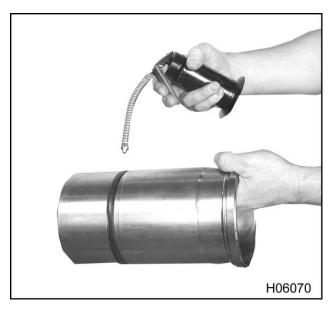
Figure 482 Cylinder sleeve and crevice seal
