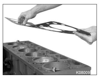
Figure 351 Cylinder head gasket
