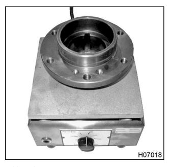
Figure 325 Damper hub and hot plate
