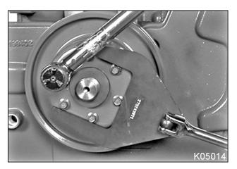
Figure 331 Fan Wrench and fan drive pulley
