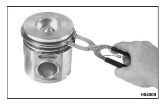
Figure 456 Piston ring removal (typical)
