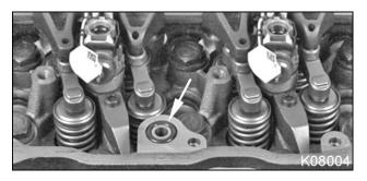
Figure 220 Oil inlet O-ring
