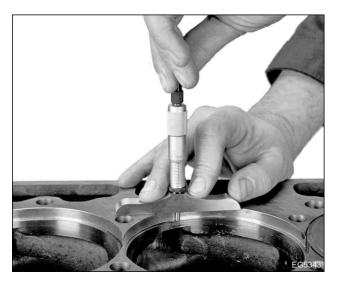
Figure 474 Counterbore depth measurement
