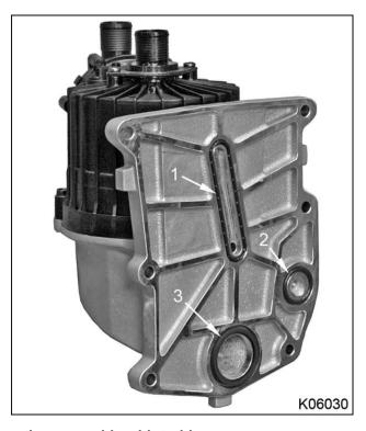
Figure 545 Crankcase breather assembly with turbine
