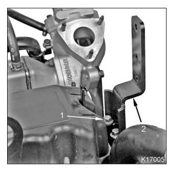
Figure 136 Tube support bracket
