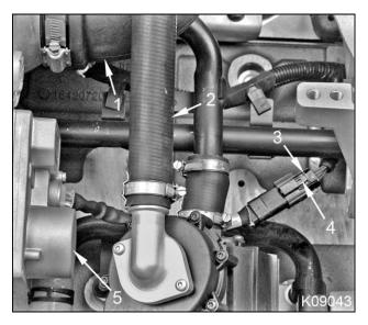
Figure 44 VGT actuator connector and turbocharger air intake duct
