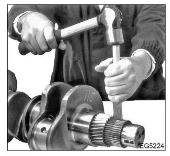
Figure 509 Oil pump spline drive removal
