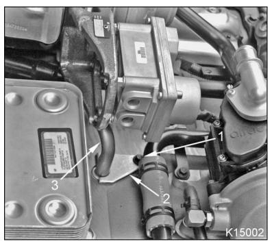
Figure 128 Turbocharger oil drain tube, bracket, and bolt
