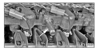
Figure 215 Brake shut-off valve
