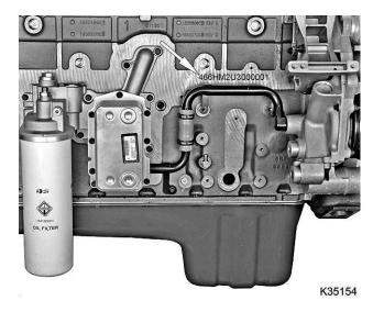
Figure 1 Engine serial number
