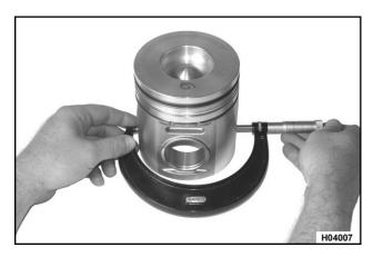
Figure 460 Measure piston skirt diameter (typical)
