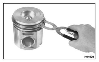
Figure 485 Piston rings installation (typical)
