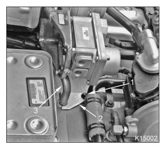
Figure 46 VGT oil drain tube, bracket, and bolt
