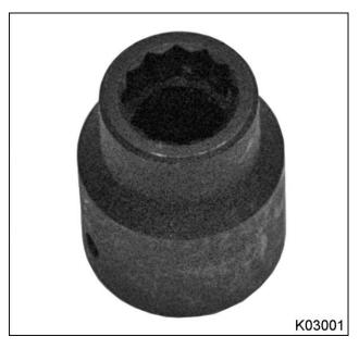
Figure 303 Lower Idler Gear Socket
