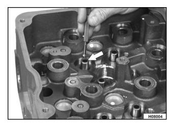
Figure 370 Measure valve guide with ball gauge
