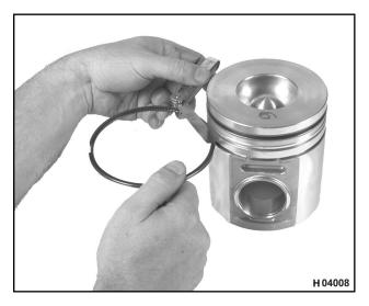
Figure 459 Measure ring groove (typical)
