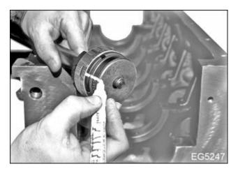
Figure 521 Camshaft bearing oil hole location mark
