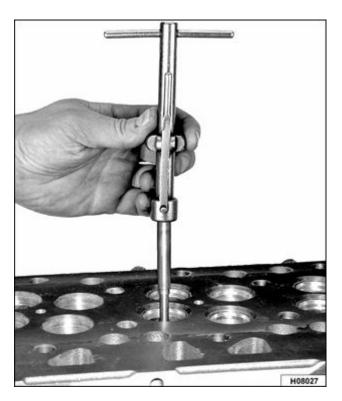
Figure 381 Valve guide pilot
