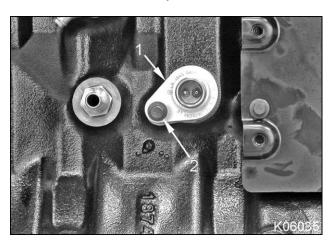
Figure 541 Coolant heater (intake side of crankcase)
