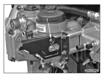
Figure 543 Oil filler tube support
