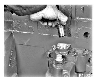
Figure 265 Regulator valve installation
