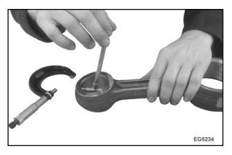
Figure 463 Piston pin bushing measurement
