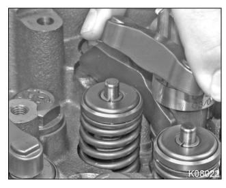
Figure 348 Valve bridge removal
