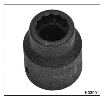
Figure 313 Lower Idler Gear Socket
