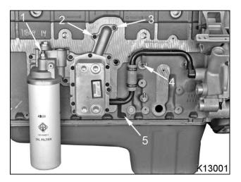
Figure 50 Oil system module and coolant tube
