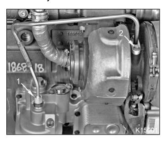
Figure 122 Turbocharger oil supply tube assembly
