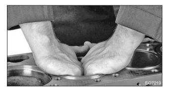
Figure 483 Cylinder sleeve installation
