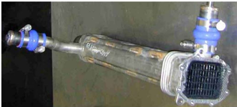
Figure 3 - EGR cooler ports: plugged
