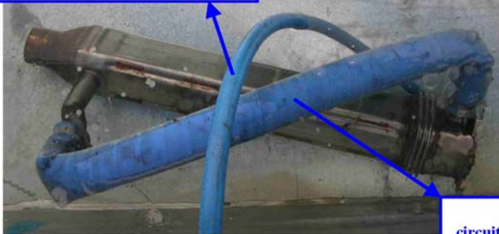
Figure 2 - EGR cooler ports: short-circuited
