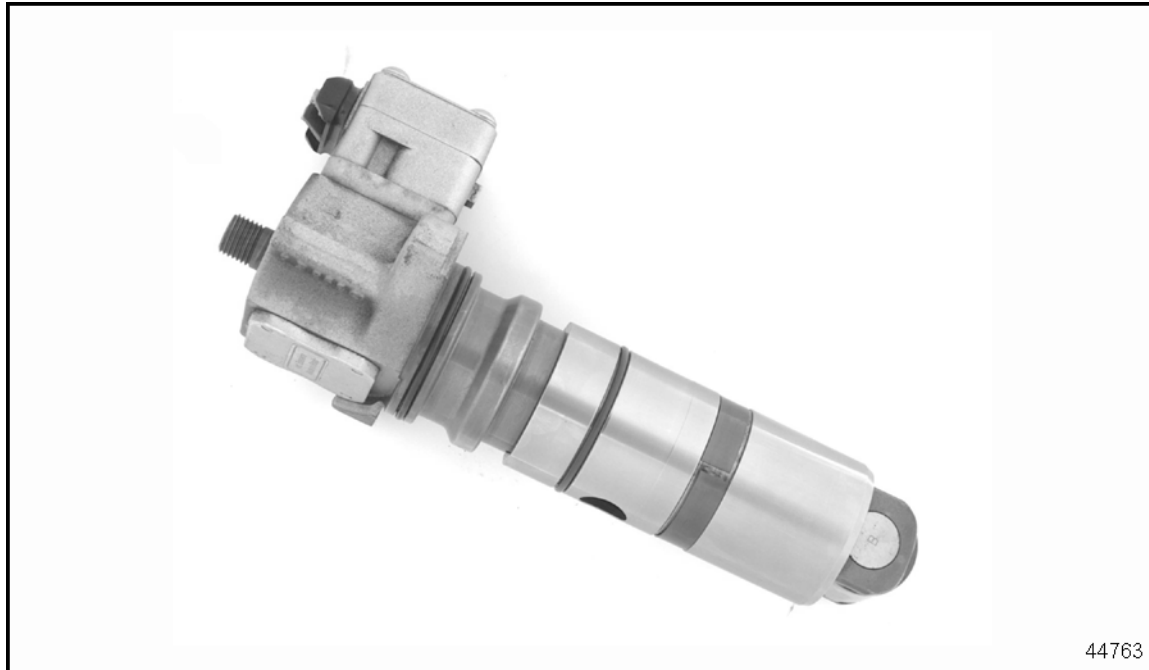
Figure 1-9 MBE Unit Pump
