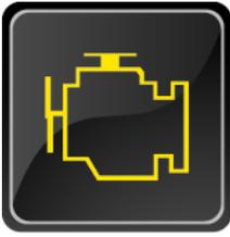
The Malfunction Indicator Lamp (MIL) is controlled by DDEC VI.
