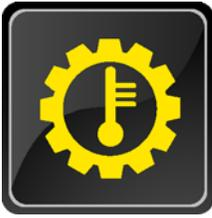
The AGS2 Trans Temp Lamp is controlled by DDEC VI.
