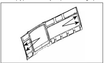
2. Remove (4) screws to remove Upper Switch Cluster.
