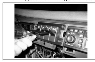
3. Pinch to unlock connector and remove Upper Switch Cluster.
