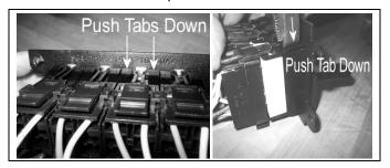
...and then push switch out of plate on top side...
