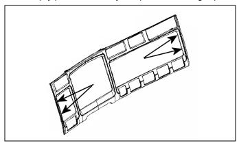
2. Remove (4) screws to remove Speedo - Tach panel.
