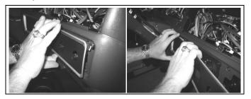
3. Remove (4) screws to remove HVAC module.
