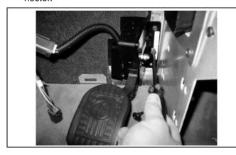
9. Passenger side, pry to remove threshold plate and unscrew (5) screws to remove threshold.
