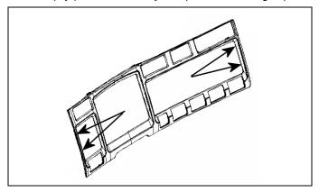
2. Insert (2 per side) 3/32 in. (2.5 mm) diameter punch or allen wrench to unhook and remove radio.
