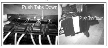
...and then push switch out of plate on top side...
