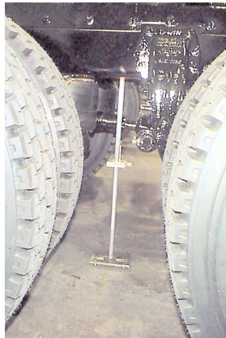
Gage Repositioned Under Frame, Between Axles And Slider Raised To Frame
