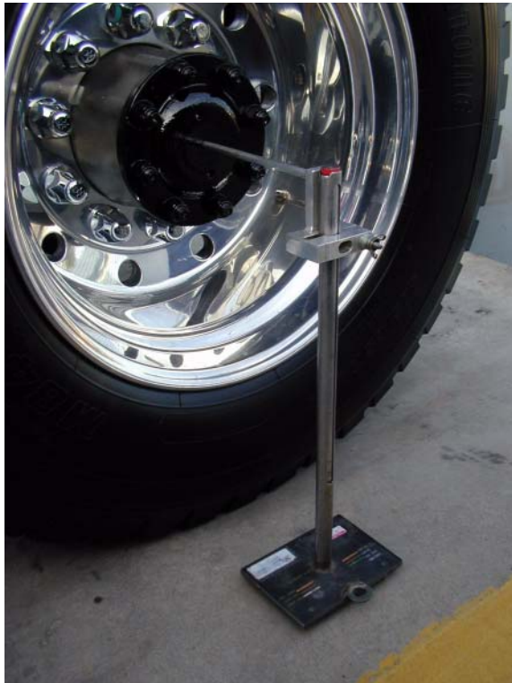
Pointer Aligned With Center Of Hub
