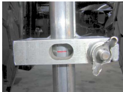
Groove located in the window of the tolerance box.
