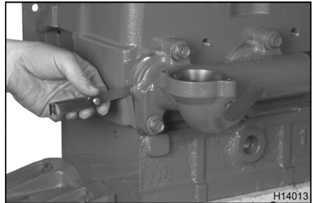
Figure 75 Checking exhaust manifold for cracks and warpage
