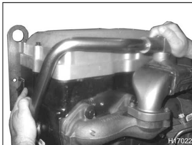
Figure 120 Installing the EGR cooler return tube
