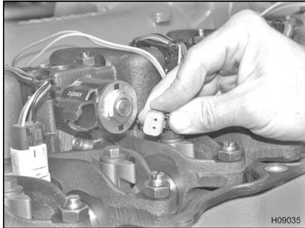
Figure 622 Disconnecting brake shutoff valve
