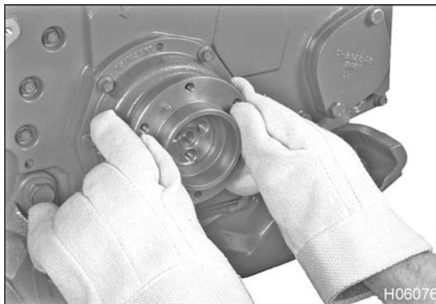
Figure 264 Installation of vibration damper hub
