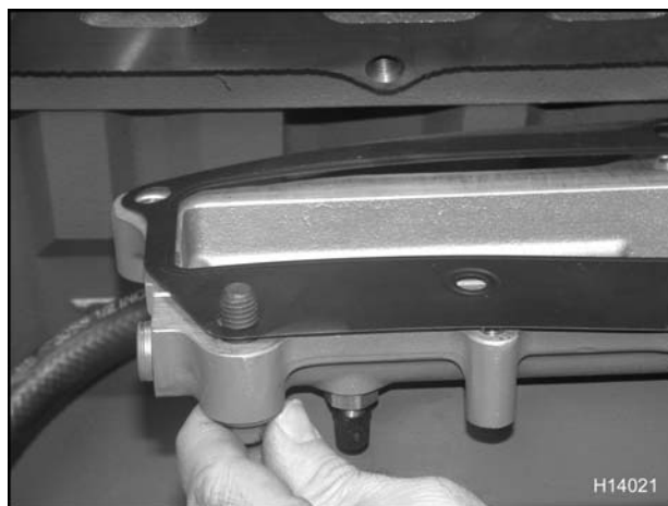
Figure 81 Aligning intake gasket to manifold
