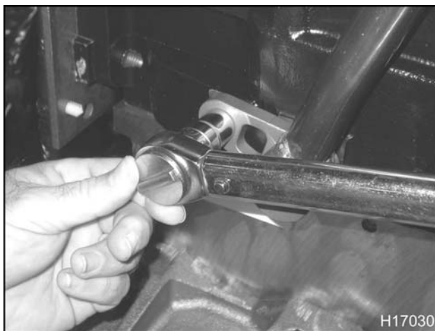
Figure 124 Torquing the EGR cooler return tube mounting bolt
