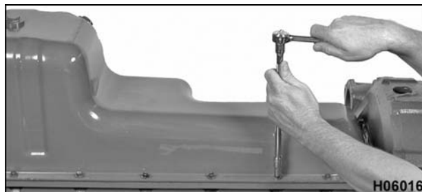
Figure 295 Installing oil pan mounting bolts
