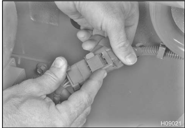
Figure 450 Disconnecting the VGT connector
