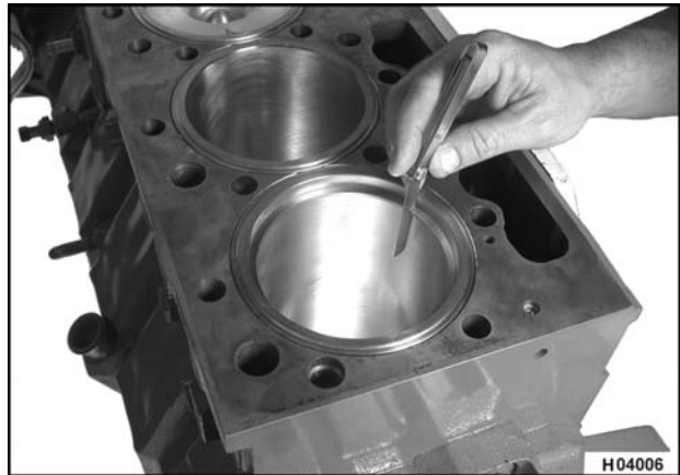
Figure 324 Checking cylinder sleeve piston ring end gap
