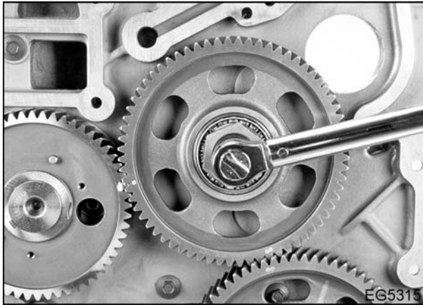
Figure 250 Installing the upper idler gear mounting bolt
