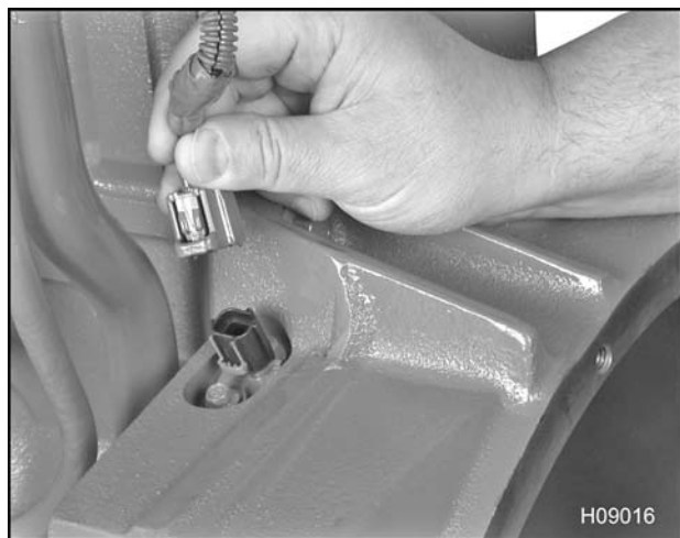
Figure 464 Disconnecting the CKP sensor
