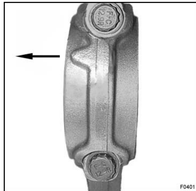
Figure 341 Connecting rod cap with M12 connecting rod cap bolts (protrusion points to front of engine)
