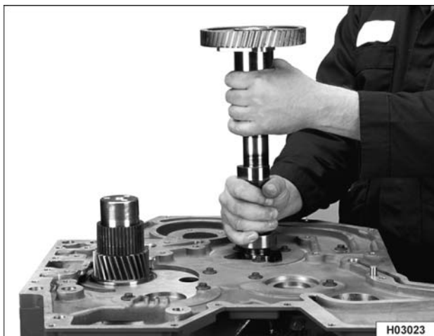
Figure 371 Removing the camshaft assembly
