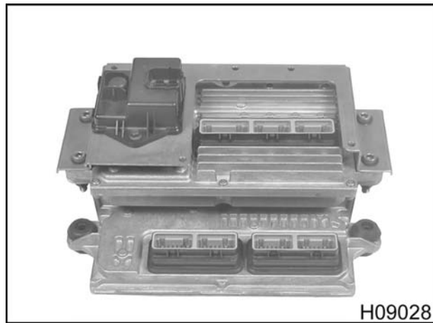
Figure 493 ECM, IDM and EGR drive modules assembled
