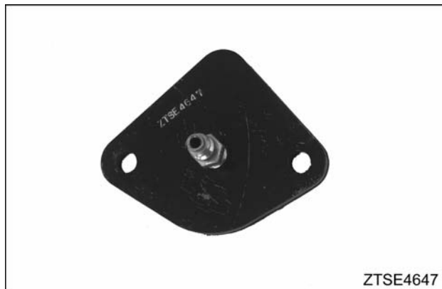
Figure 664 Thermostat opening pressure adapter– cylinder head, ZTSE4647
