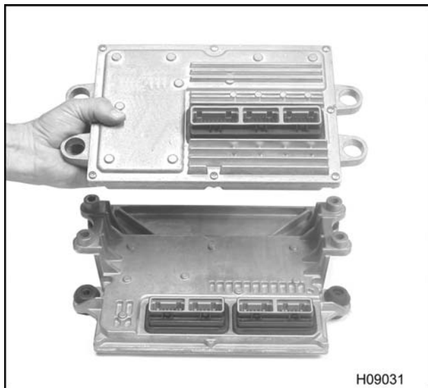
Figure 490 Installing the IDM onto the ECM
