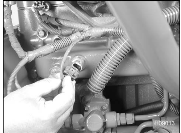
Figure 512 Connecting to the MAT sensor
