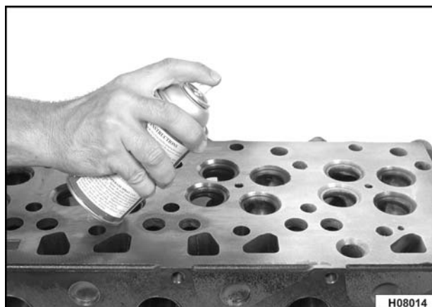
Figure 157 Spraying developer on cylinder head
