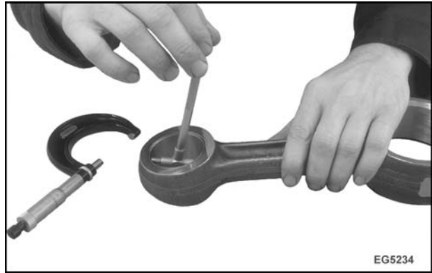
Figure 315 Measuring piston pin bushing inside diameter
