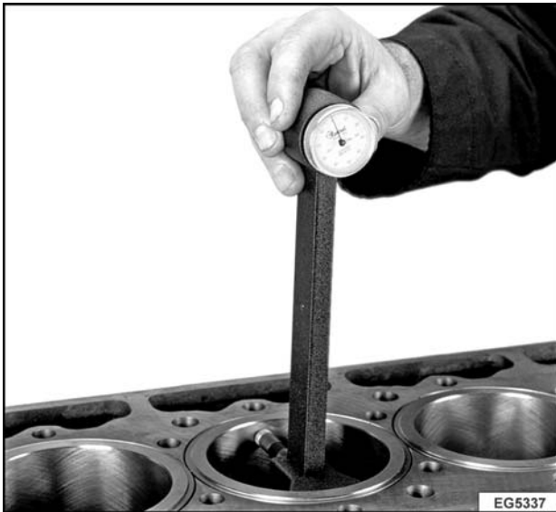
Figure 323 Checking cylinder sleeve inside diameter with dial bore gauge
