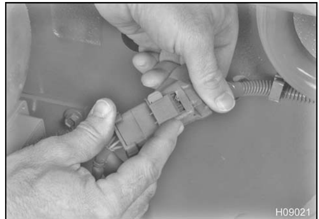
Figure 519 Connecting to the VGT harness
