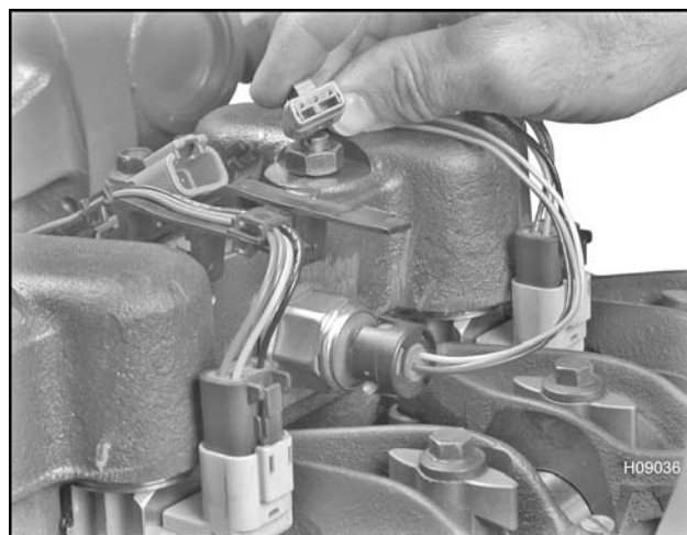
Figure 651 BCP sensor electrical connector
