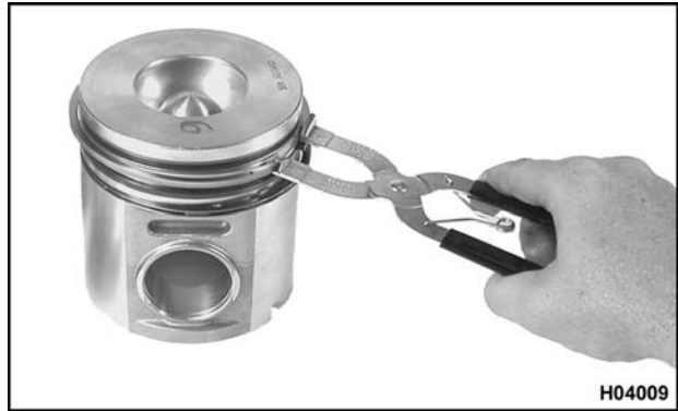
Figure 308 Removing piston rings (DT 466 piston shown)
