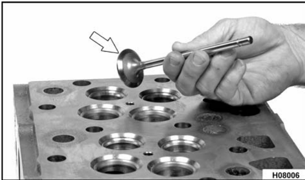
Figure 172 Applying Prussian Blue® to valve face
