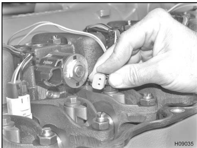
Figure 650 Brake shutoff valve assembly electrical connector
