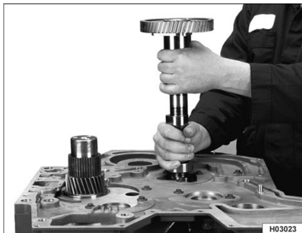
Figure 382 Installing camshaft assembly
