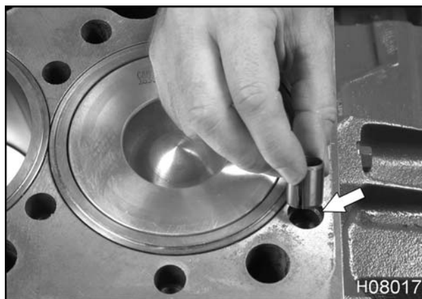
Figure 195 Installing alignment dowels
