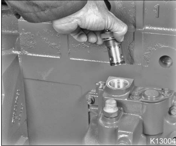
Figure 413 Removing the regulating valve
