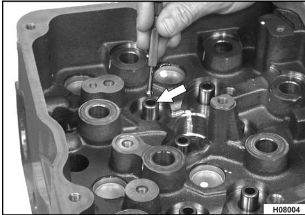
Figure 163 Measuring valve guide with ball gauge
