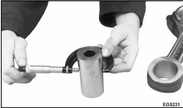
Figure 314 Measuring piston pin outside diameter
