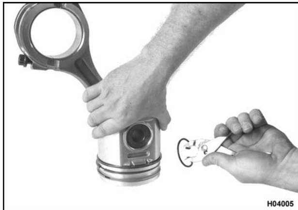
Figure 343 Installing piston pin retaining rings
