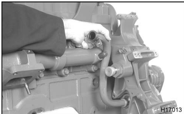
Figure 103 EGR cooler supply tube
