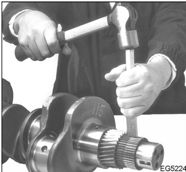
Figure 367 Removing oil pump drive spline
