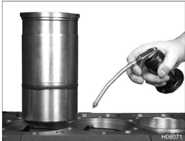
Figure 335 Lubrication of cylinder sleeve bore
