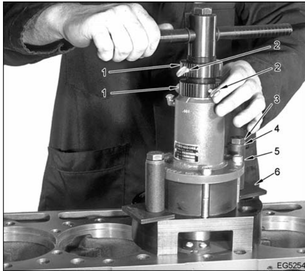
Figure 333 Positioning counterboring tool
