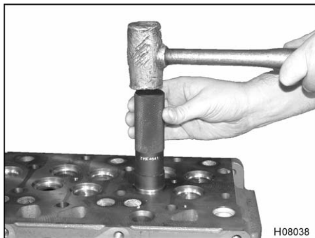
Figure 183 Driving valve seat into place
