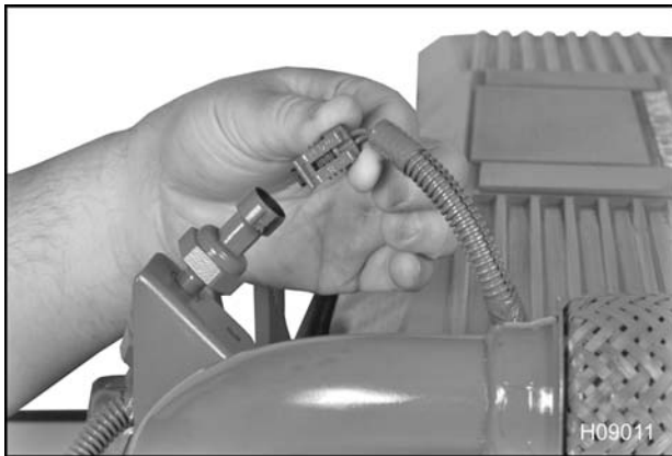
Figure 453 Disconnecting the EBP sensor
