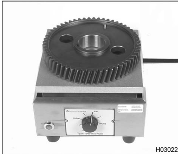
Figure 384 Heating the camshaft gear
