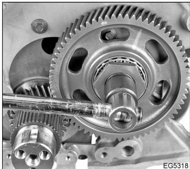
Figure 236 Removing the lower idler gear
