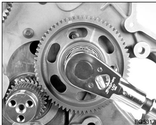
Figure 248 Installing the lower idler gear mounting bolt
