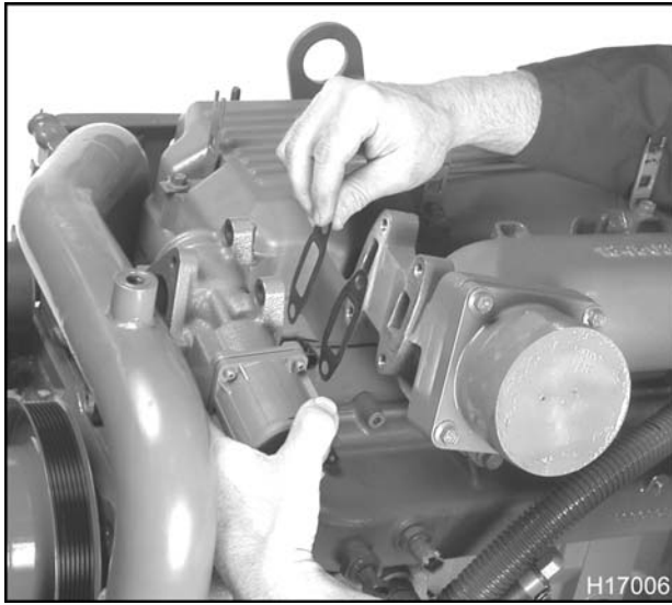
Figure 110 EGR valve gasket at EGR mixer duct
