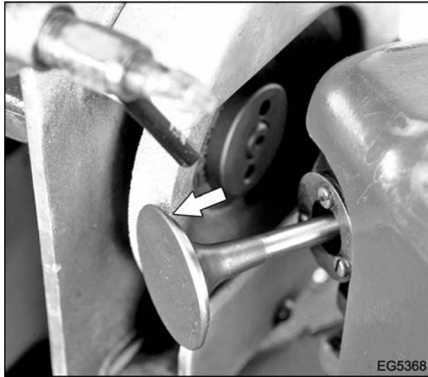
Figure 168 Grinding valve face
