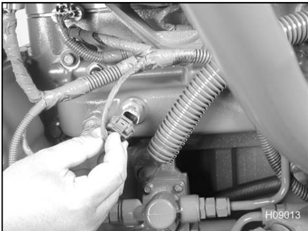
Figure 457 Disconnecting the MAT sensor
