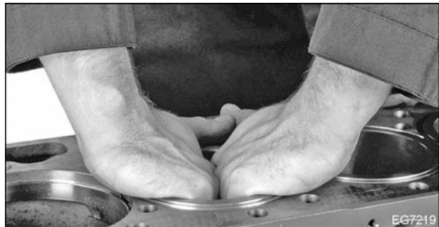
Figure 336 Installation of cylinder sleeve
