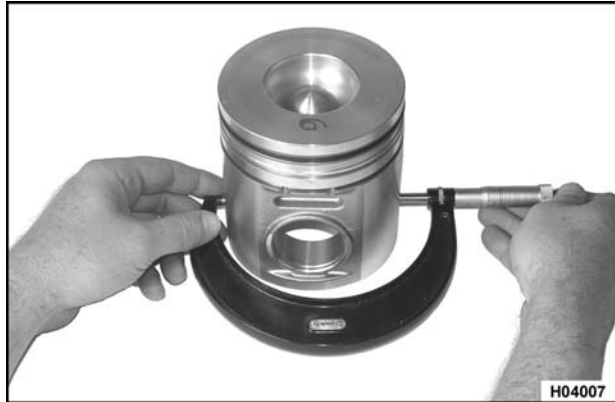
Figure 312 Measuring piston skirt diameter
