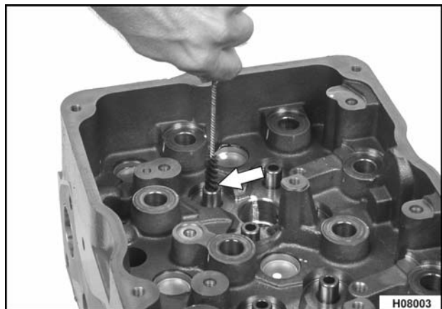
Figure 162 Cleaning valve guides
