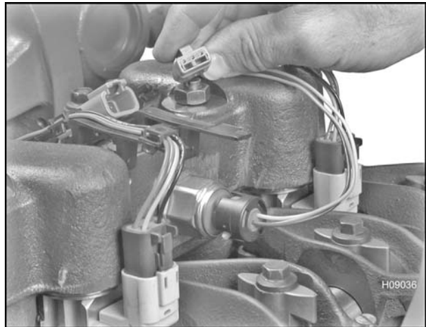
Figure 487 Connecting the BCP sensor
