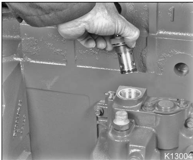
Figure 429 Installing the oil pressure regulating valve
