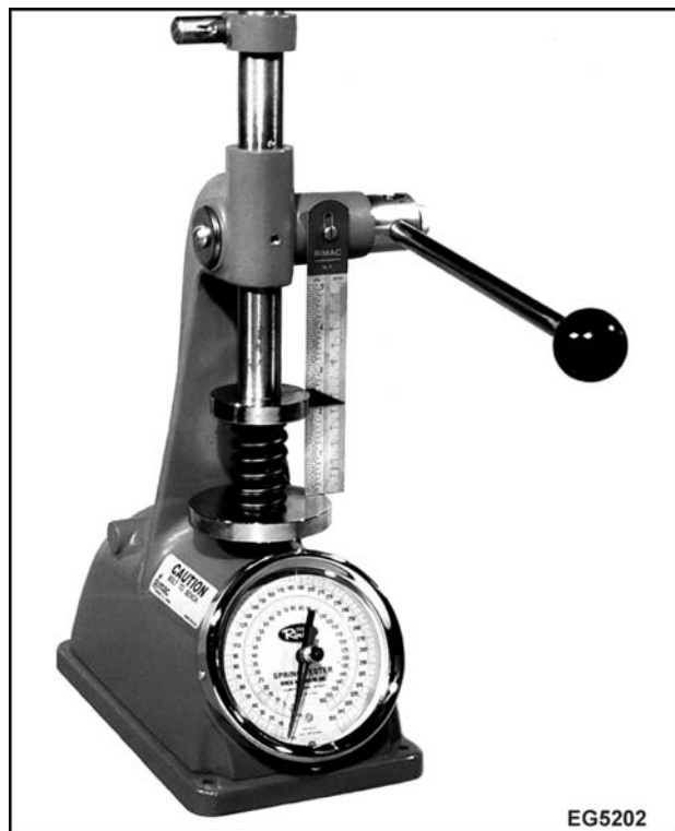
Figure 186 Measuring valve spring tension
