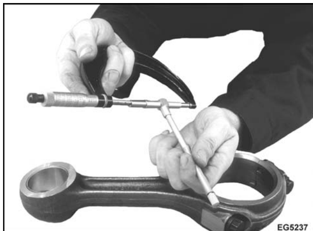
Figure 317 Measuring connecting rod bearing bore taper
