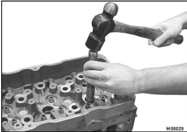
Figure 191 Installing fuel injector sleeve
