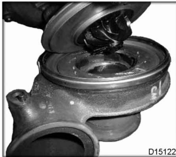
Figure 11 Center section onto the turbine housing
