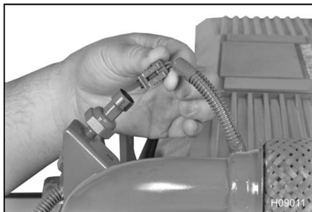
Figure 516 Connecting to the EBP sensor
