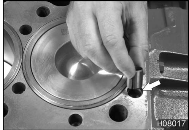
Figure 146 Removing alignment dowels
