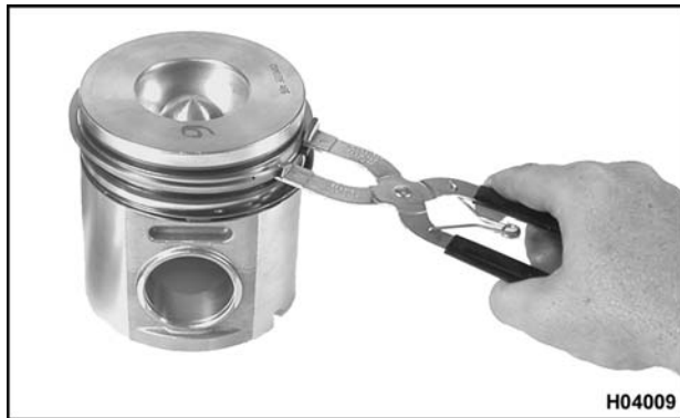
Figure 337 Installing piston rings (466 piston shown)
