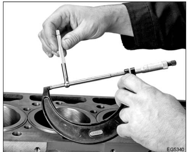
Figure 322 Measuring telescoping gauge
