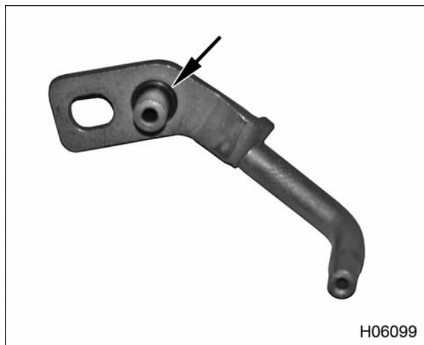
Figure 357 O-ring (underside) of new piston cooling tube
