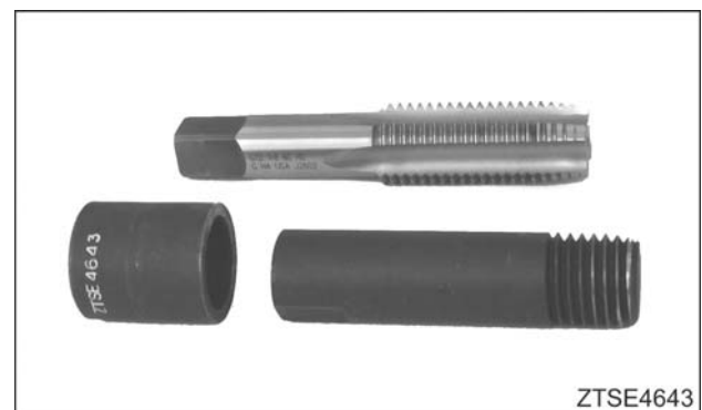
Figure 662 Injector sleeve remover, ZTSE4643
