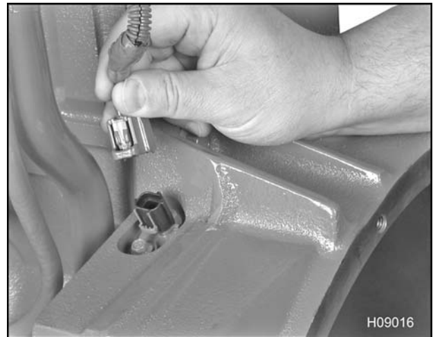
Figure 505 Connecting to the CKP sensor
