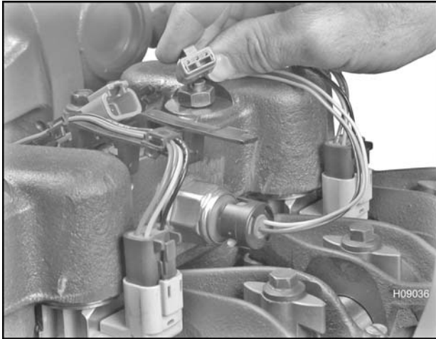
Figure 626 Disconnecting BCP sensor
