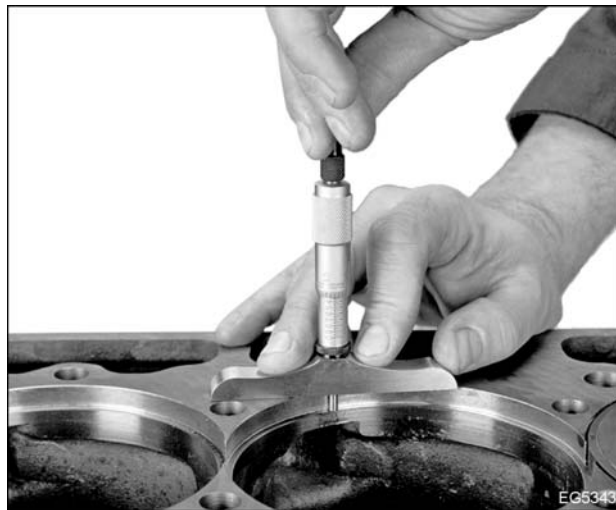
Figure 326 Checking counterbore depth with depth micrometer
