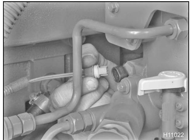
Figure 463 Disconnecting the WIF sensor
