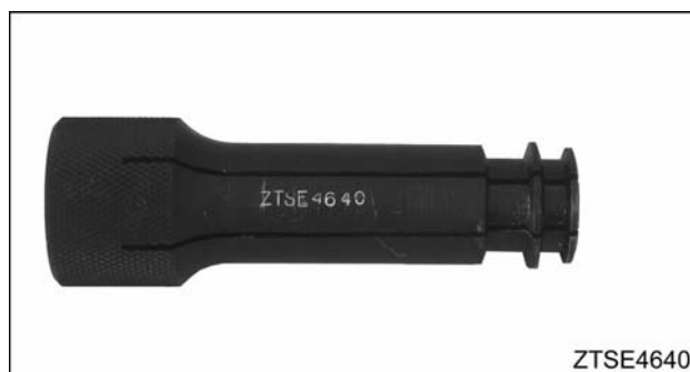
Figure 659 Valve seat remover (collet), ZTSE4640
