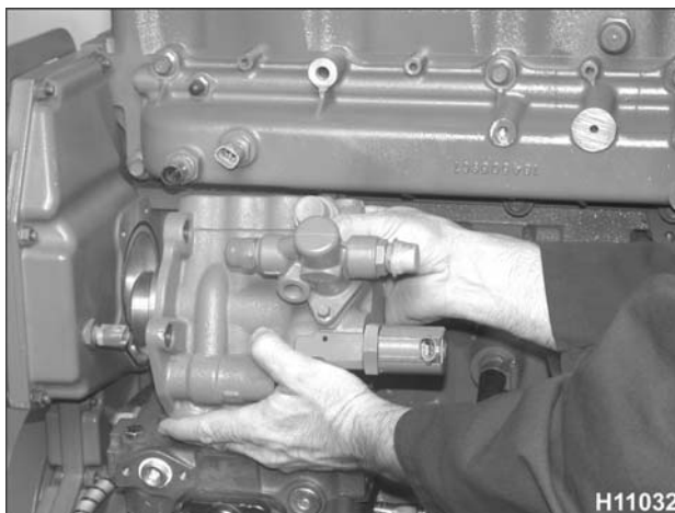
Figure 564 Installing the high-pressure pump assembly
