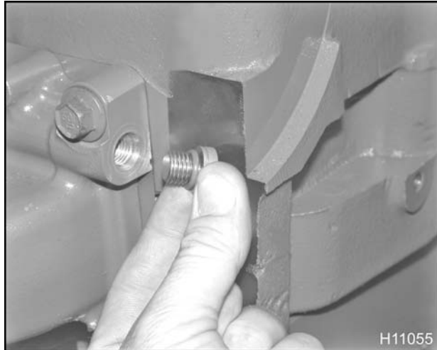
Figure 571 Installing the fuel rail plug assembly (2)
