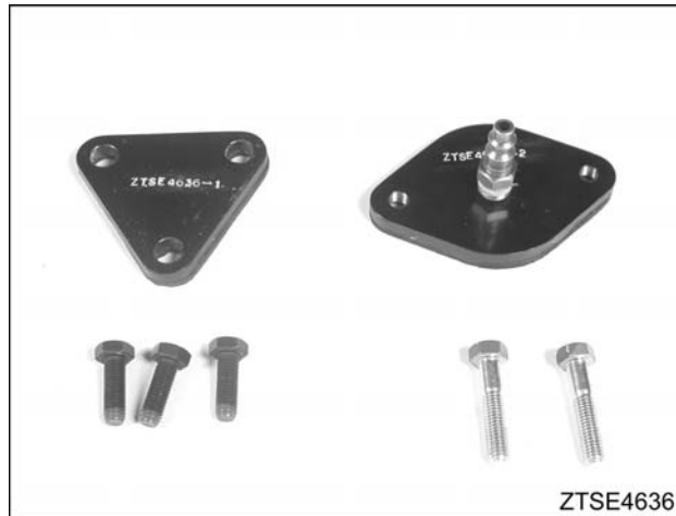
Figure 657 EGR cooler pressure test plates, ZTSE4636
