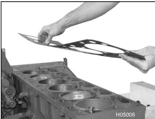
Figure 145 Removing cylinder head gasket
