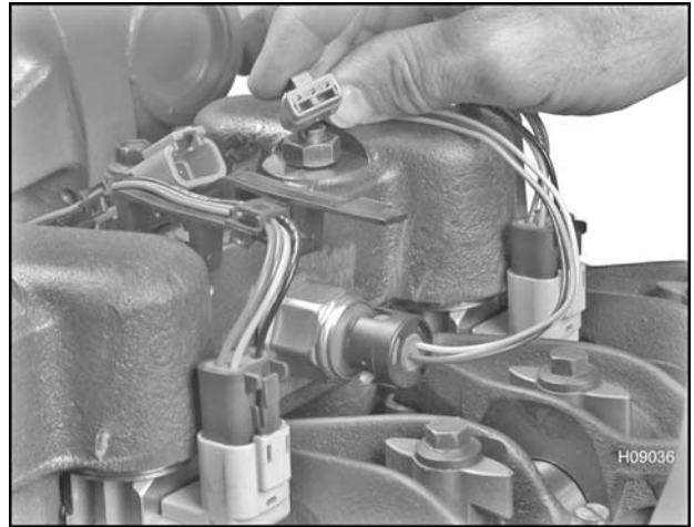
Figure 482 Disconnecting the BCP sensor
