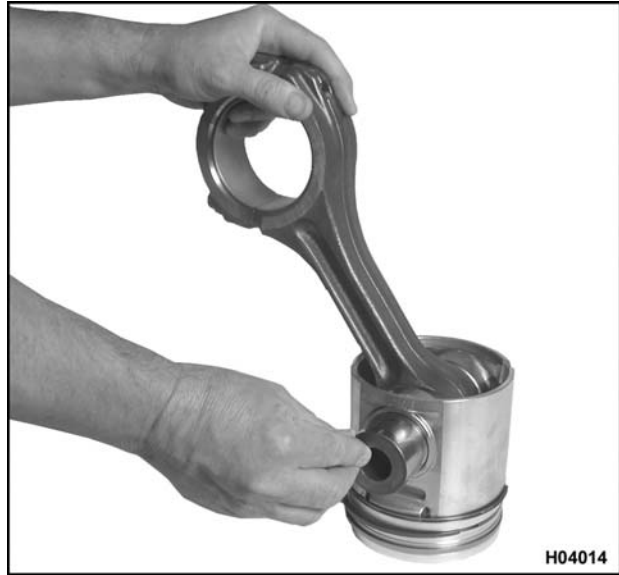
Figure 340 Installing piston pin
