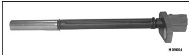
Figure 439 Crankshaft Position (CKP) sensor
