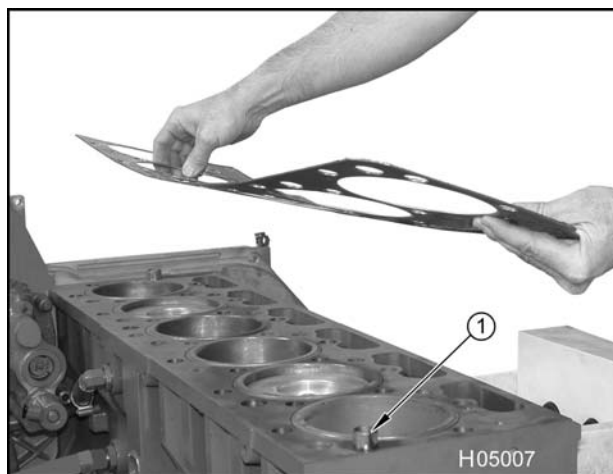
Figure 196 Installing cylinder head gasket
