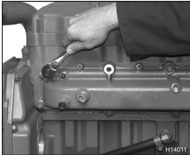
Figure 74 Intake manifold mounting bolts
