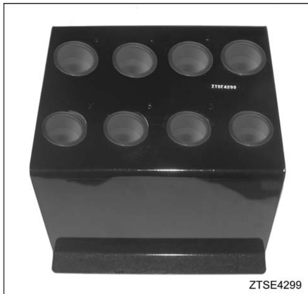
Figure 663 Injector rack – ZTSE4299B, Injector rack cups – ZTSE4645
