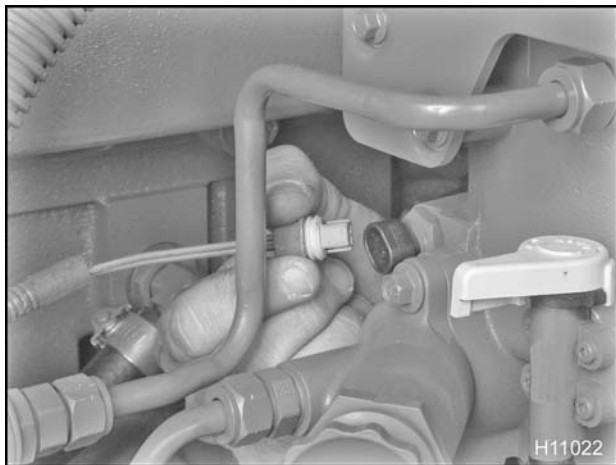
Figure 506 Connecting to the WIF sensor
