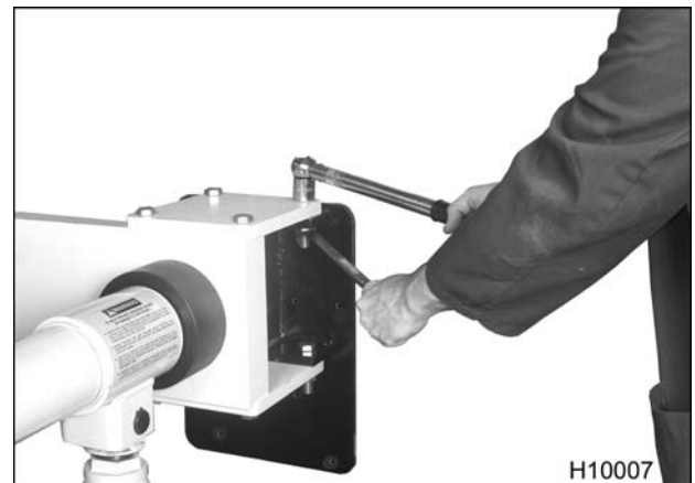
Figure 55 Installing the adapter plate to engine stand
