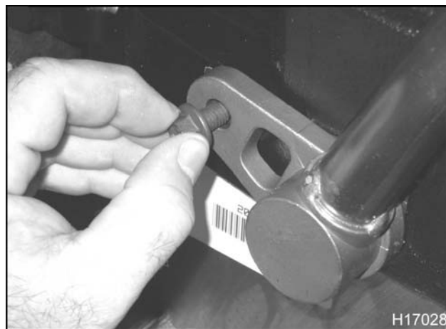
Figure 121 Installing the EGR return tube mounting bolt
