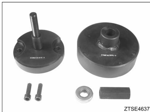
Figure 658 Rear seal installer, ZTSE4637
