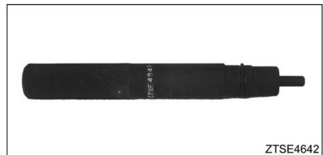
Figure 661 Injector sleeve installer, ZTSE4642
