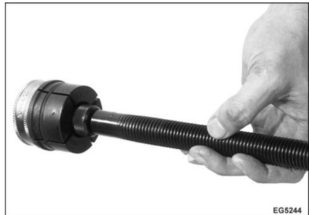
Figure 377 Camshaft bushing installation tool
