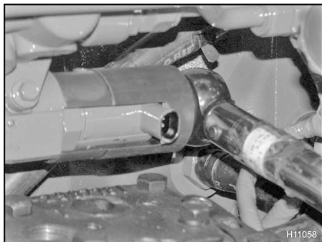
Figure 563 Installing the IPR valve
