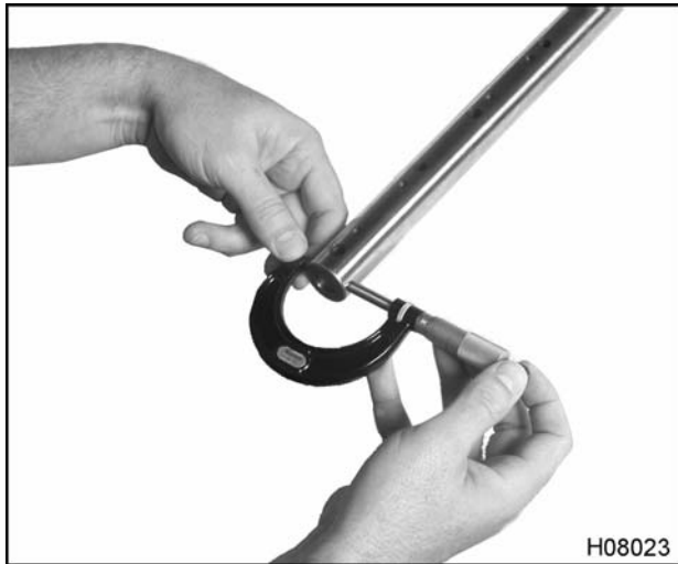
Figure 149 Measuring rocker arm shaft
