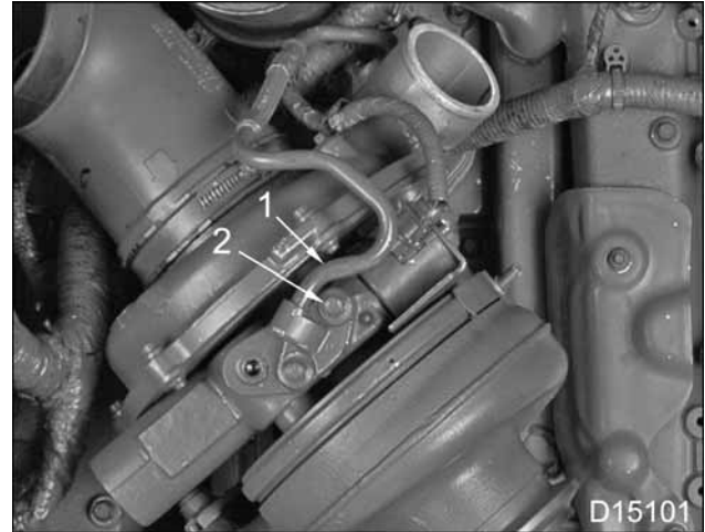
Figure 52 Oil supply tube to VGT
