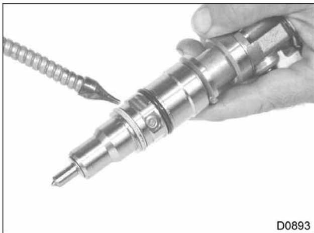
Figure 252 Lubrication of fuel injector O-rings
