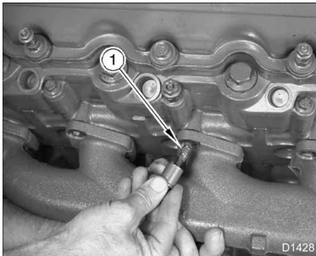
Figure 124 Bolt and spacer for left exhaust manifold
