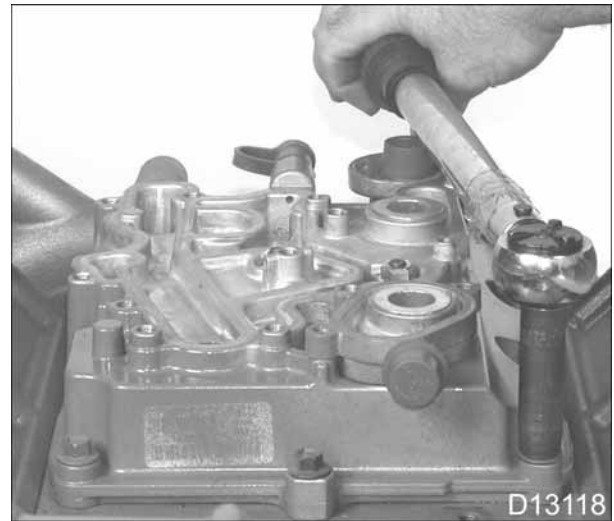
Figure 411 Mounting Bolts for oil cooler cover assembly
