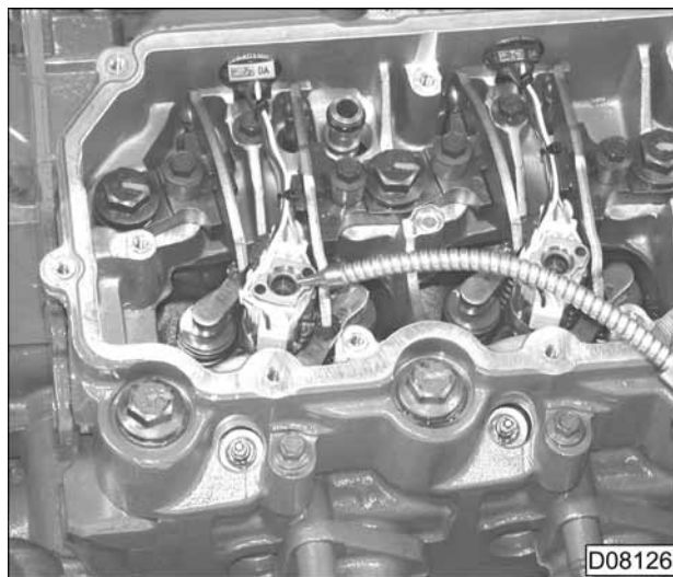
Figure 259 Lubrication of top D-ring
