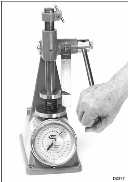
Figure 206 Measurement of valve spring free length under load
