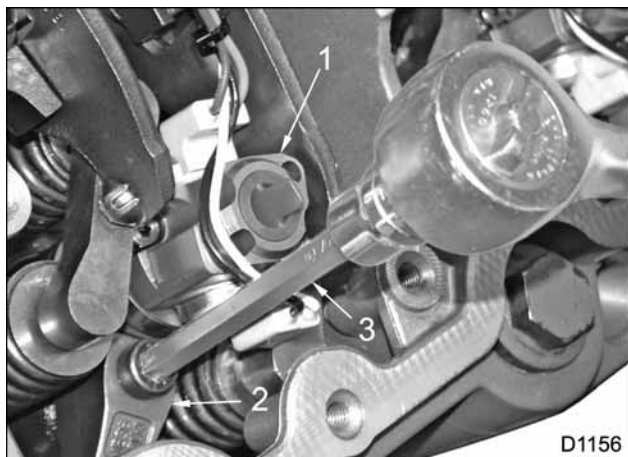
Figure 257 Fuel Injector Hold Down Wrench installed
