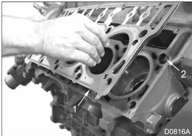
Figure 233 Installation of cylinder head gasket
