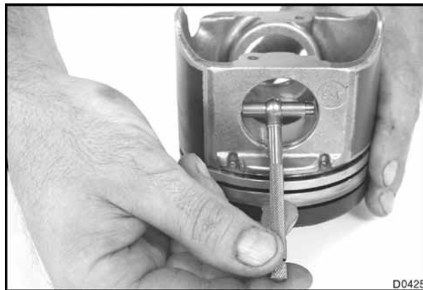
Figure 334 Inside diameter measurement of piston pin bore
