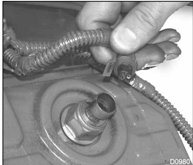
Figure 454 Electrical connector removed from ICP sensor
