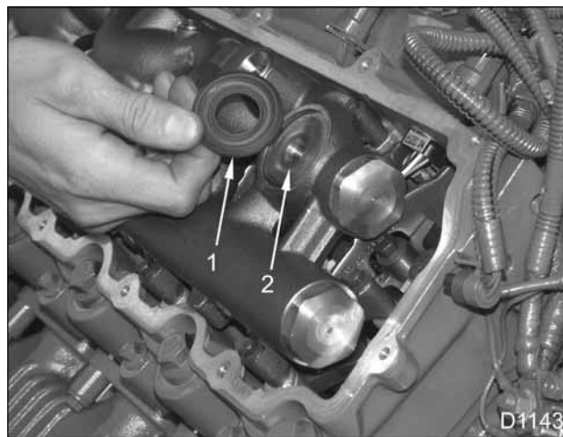
Figure 267 Installation of valve cover seal ring for ICP sensor
