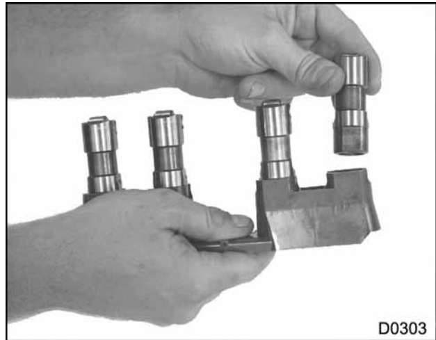
Figure 224 Installation of cam follower in guide
