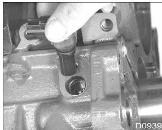
Figure 475 CKP sensor installation
