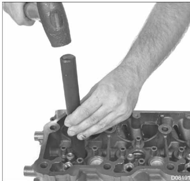
Figure 212 Installation of fuel injector sleeve into bore
