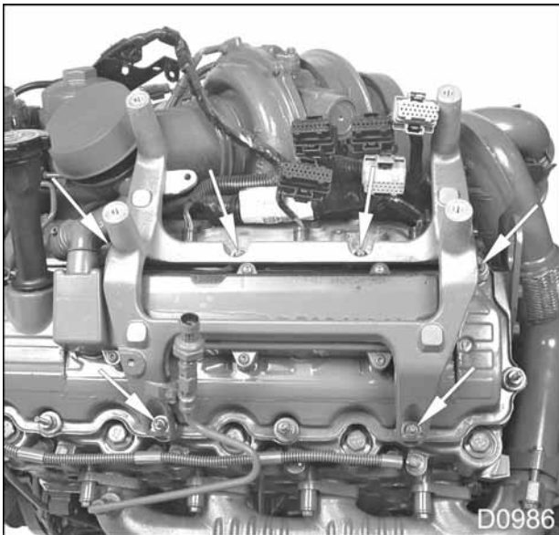
Figure 496 Nuts on valve cover studs for ECM and IDM bracket
