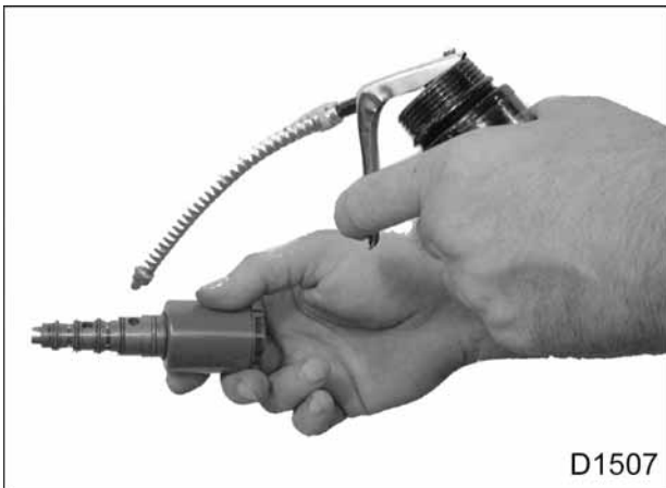
Figure 483 Lubrication of control valve O-rings
