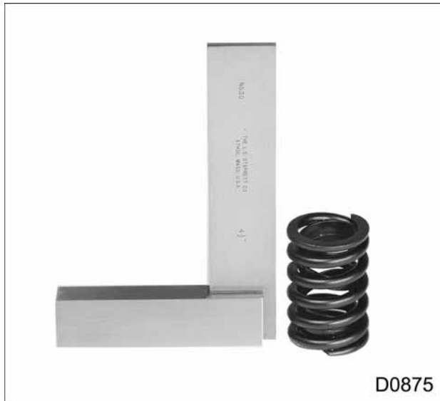
Figure 204 Flatness check of valve spring
