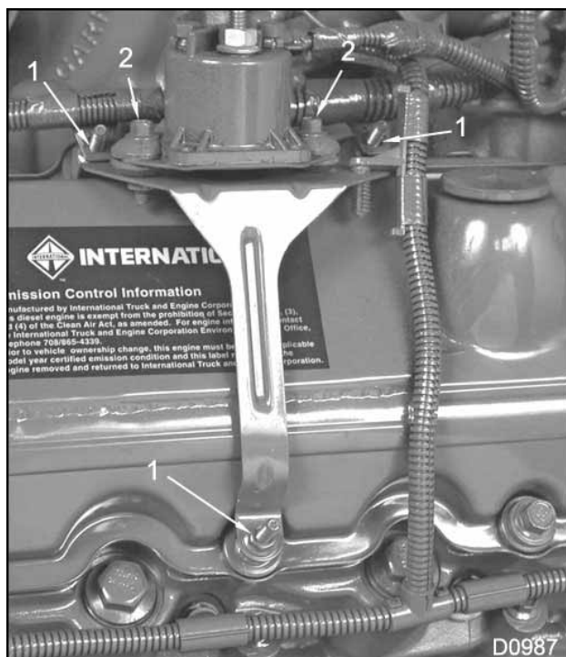
Figure 493 Glow plug relay terminals
