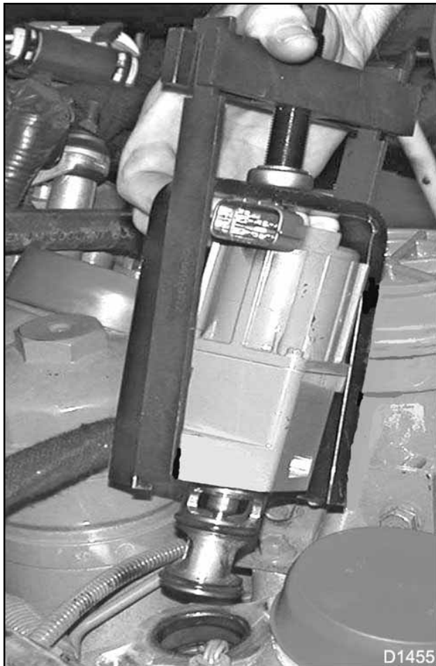
Figure 447 Removal of EGR valve
