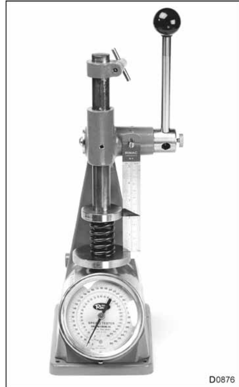
Figure 205 Measurement of valve spring free length
