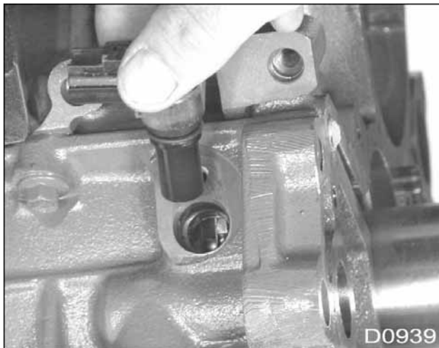
Figure 392 Crankshaft Position (CKP) sensor installation
