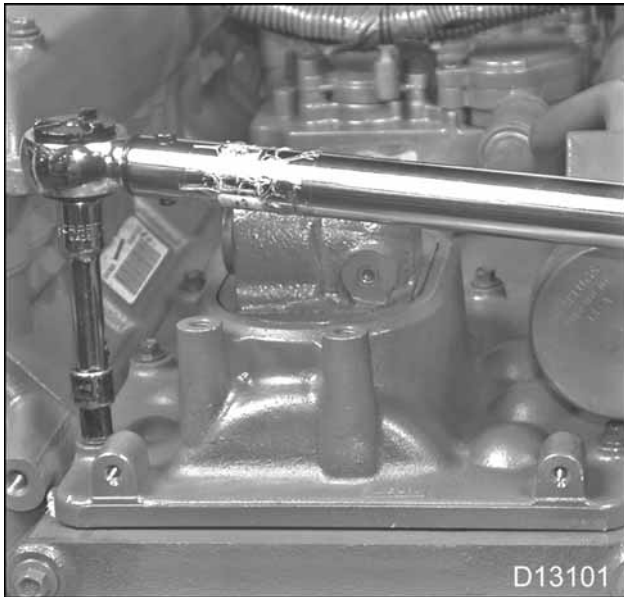
Figure 526 Torquing bolts for high-pressure oil pump cover
