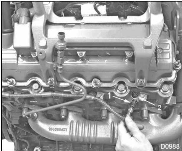
Figure 495 Installation of glow plug harness assembly
