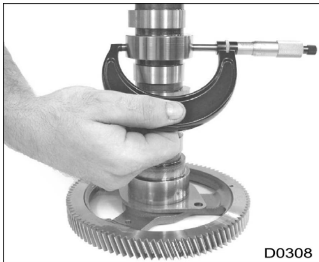
Figure 374 Measurement for camshaft bearing journal
