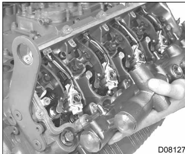
Figure 260 Alignment of oil rail assembly to oil inlets
