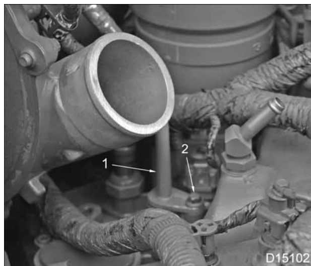
Figure 70 Oil supply tube for VGT to oil cooler cover assembly
