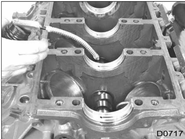
Figure 381 Upper main bearings lubrication
