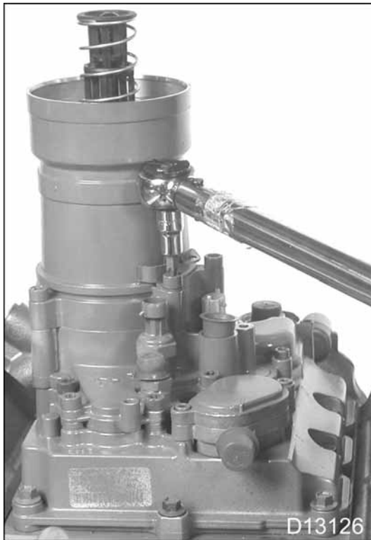
Figure 419 Oil filter housing mounting bolts
