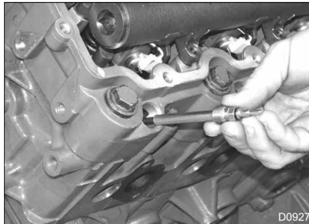
Figure 266 Installation of glow plug
