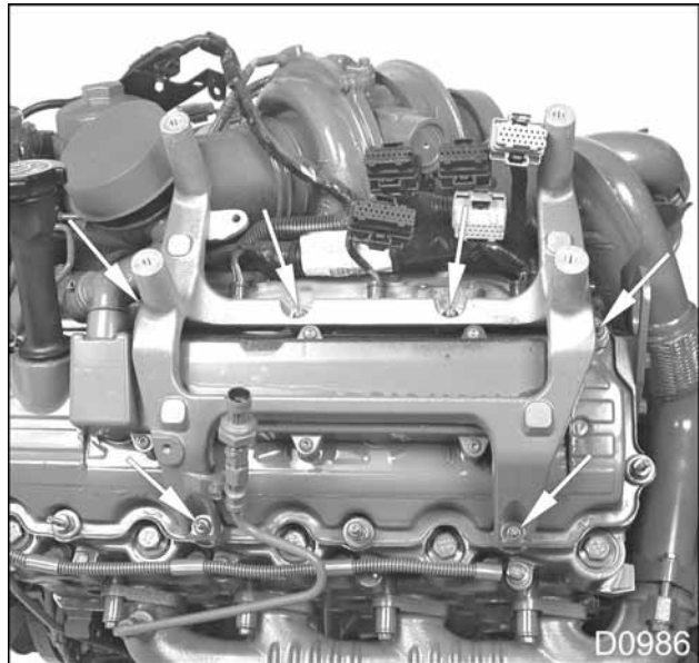
Figure 466 Mounting Bracket Bolts for ECM and IDM
