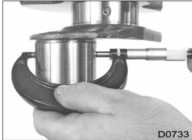
Figure 373 Measurement for crankshaft connecting rod journal
