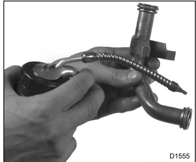
Figure 67 Lubrication for O-rings on oil drain tube for VGT
