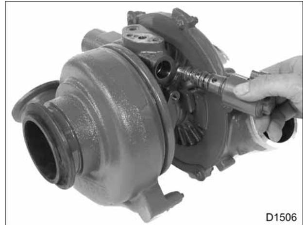
Figure 451 VGT control valve removed
