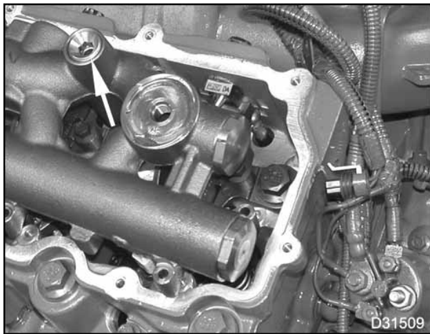
Figure 265 Crankcase-to-head tube plug (hex head)
