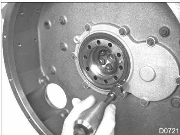
Figure 549 Hammer screw in starter hole
