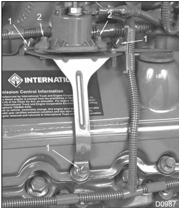
Figure 469 Glow plug relay nuts and bracket nuts
