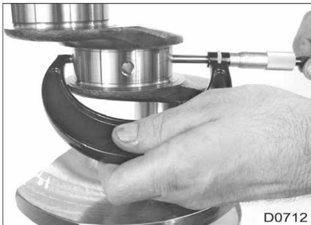
Figure 372 Measurement for crankshaft main journal
