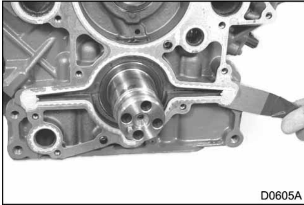
Figure 288 Sealant between crankcase and lower crankcase joint
