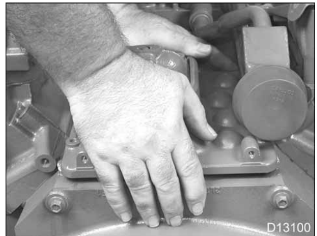
Figure 525 Seating high-pressure oil pump cover
