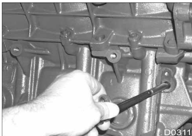
Figure 473 CMP sensor installation
