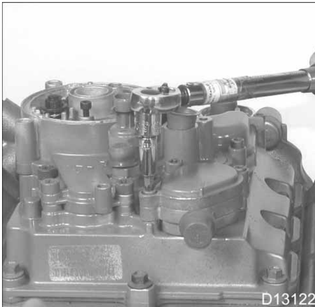
Figure 415 Cover bolts for coolant supply port of EGR cooler
