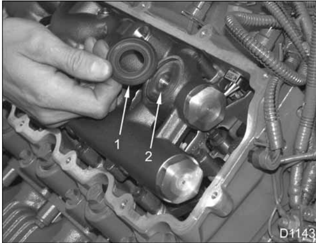
Figure 487 Installation of valve cover seal ring for ICP sensor
