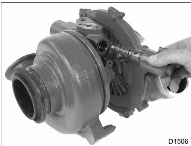
Figure 484 Installation of control valve
