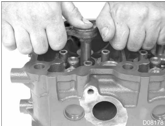
Figure 176 Fuel injector sleeve tapped
