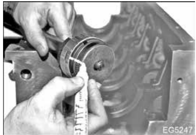
Figure 521 Camshaft bearing oil hole location mark
