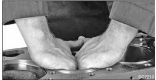
Figure 483 Cylinder sleeve installation
