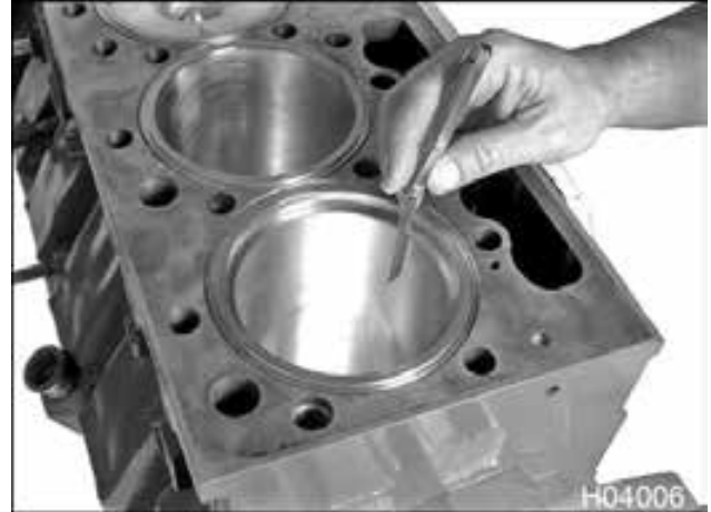
Figure 472 Measure cylinder sleeve piston ring end gap
