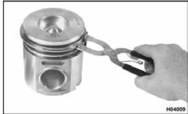
Figure 456 Piston ring removal (typical)
