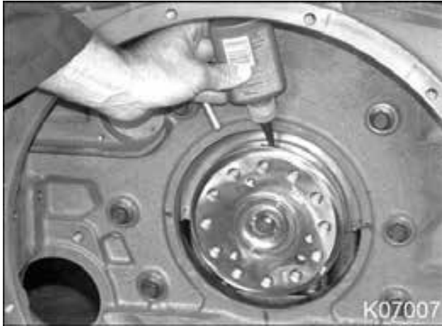
Figure 436 Application of sealant to crankshaft wear sleeve area
