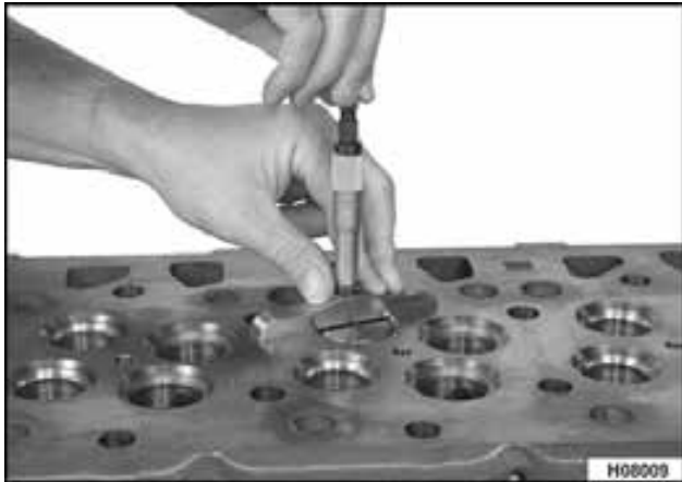
Figure 384 Measure valve recession
