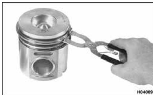
Figure 485 Piston rings installation (typical)
