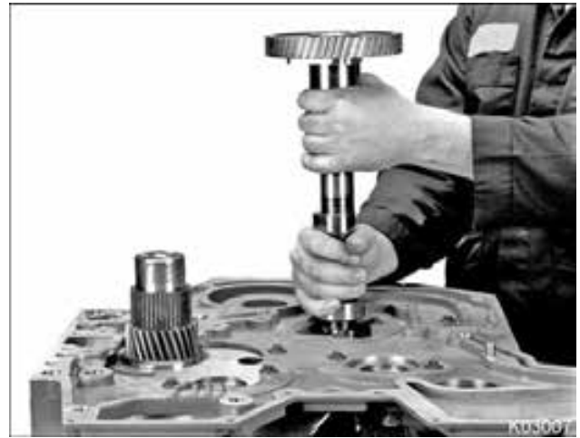
Figure 512 Camshaft assembly removal
