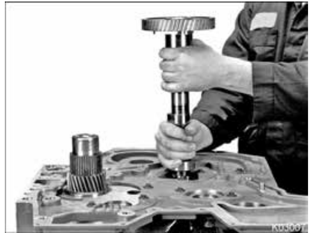
Figure 524 Camshaft assembly installation
