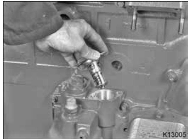
Figure 252 Thermal valve removal
