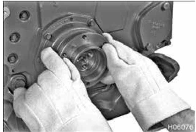
Figure 326 Damper hub installation
