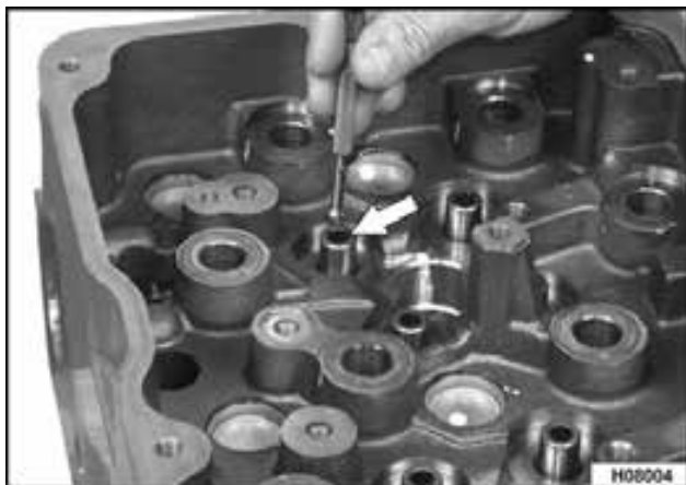
Figure 370 Measure valve guide with ball gauge
