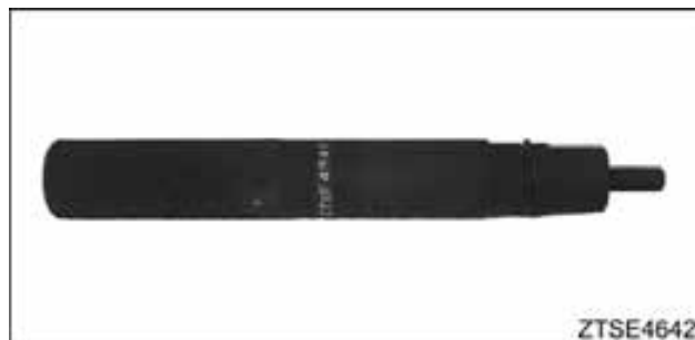
Figure 558 Injector Sleeve Installer, ZTSE4642
