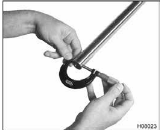
Figure 356 Rocker arm shaft measurement
