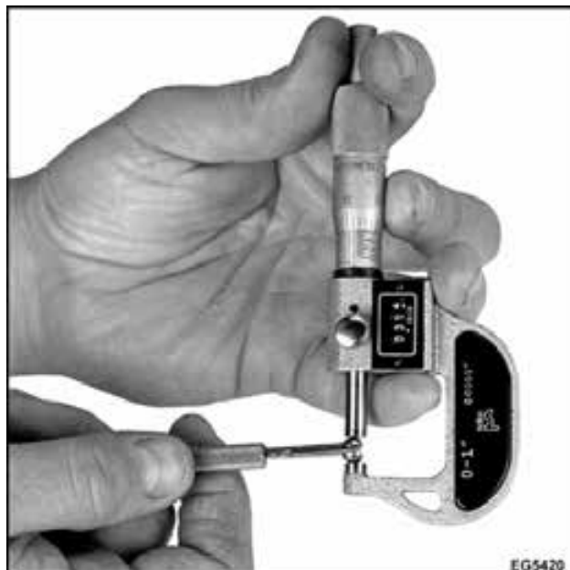
Figure 371 Measure Ball gauge with micrometer
