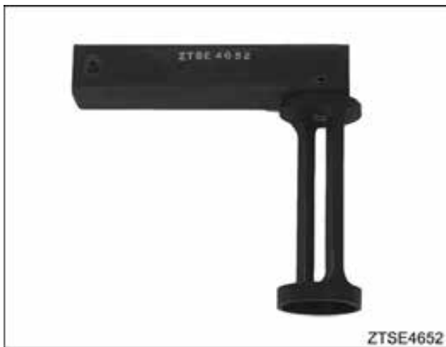
Figure 559 Valve Spring Compressor Jaws, ZTSE4652
