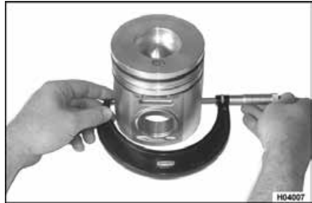
Figure 460 Measure piston skirt diameter (typical)
