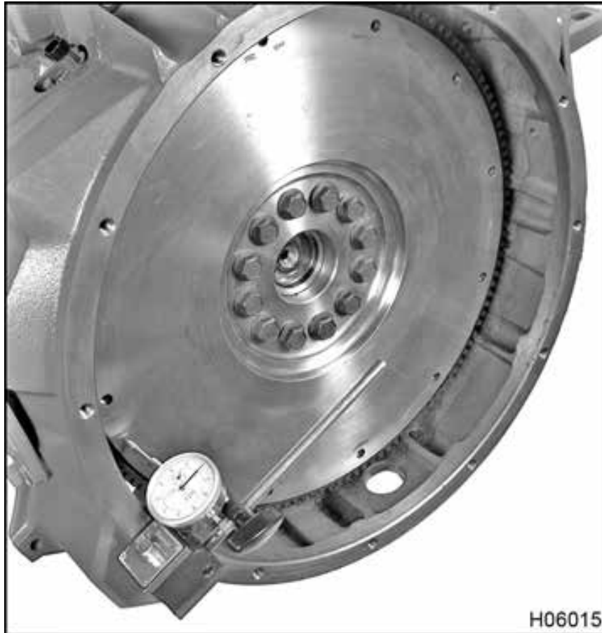
Figure 433 Flywheel surface runout measurement
