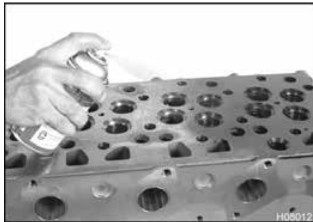
Figure 362 Spray dye penetrant on cylinder head
