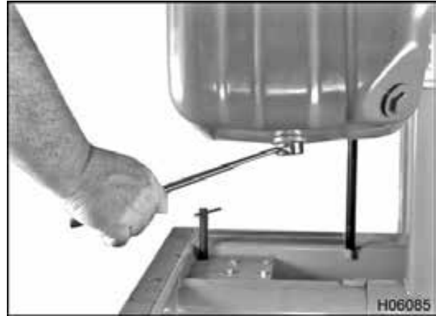
Figure 43 Oil drain plug removal
