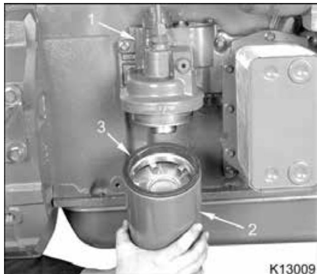
Figure 269 Oil filter installation
