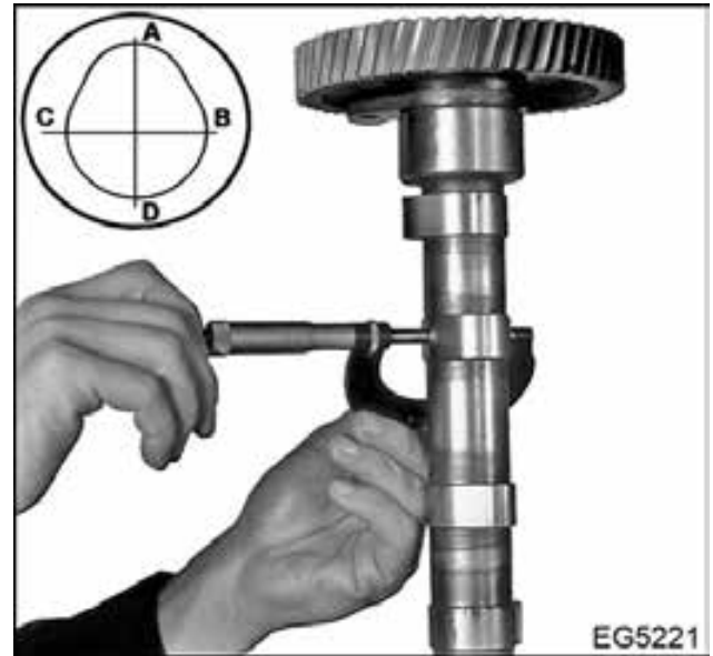
Figure 518 Camshaft lobe and journal measurement
