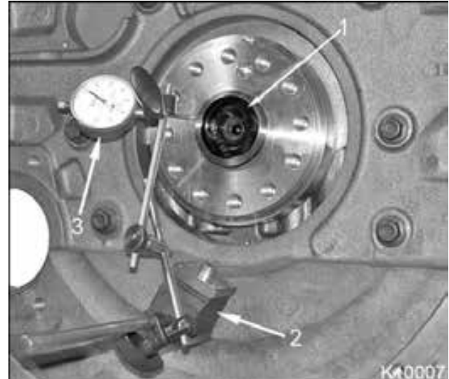
Figure 432 Crankshaft pilot concentricity measurement
