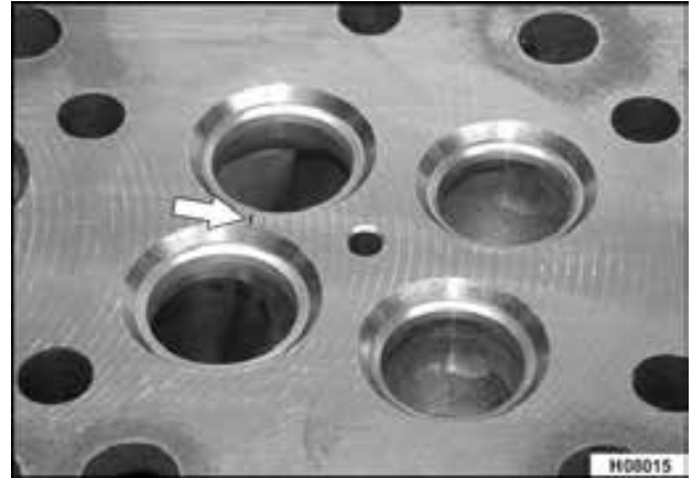
Figure 365 Crack in cylinder head
