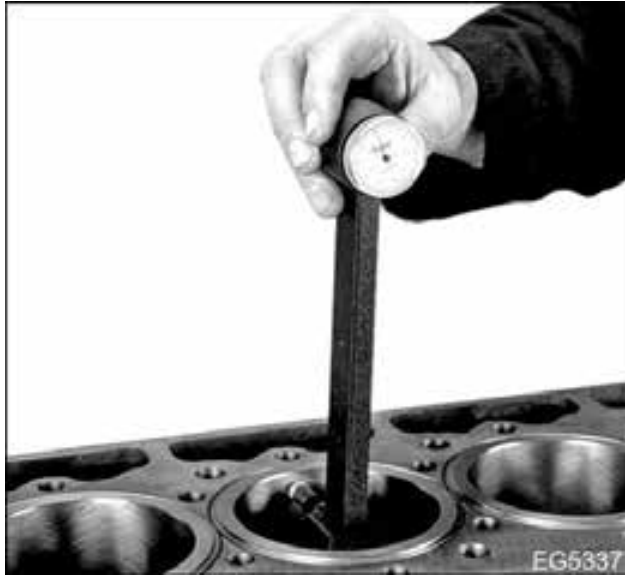
Figure 471 Cylinder sleeve taper measurement
