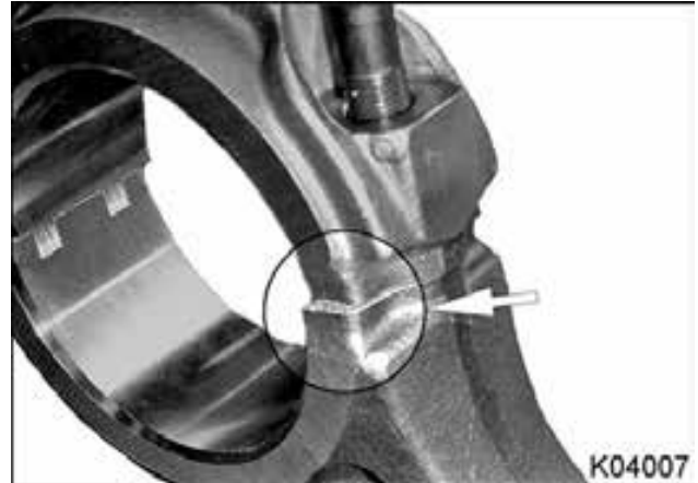
Figure 492 Incorrect connecting rod cap orientation
