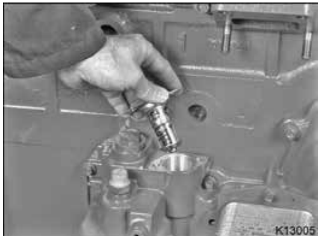
Figure 264 Thermal valve installation
