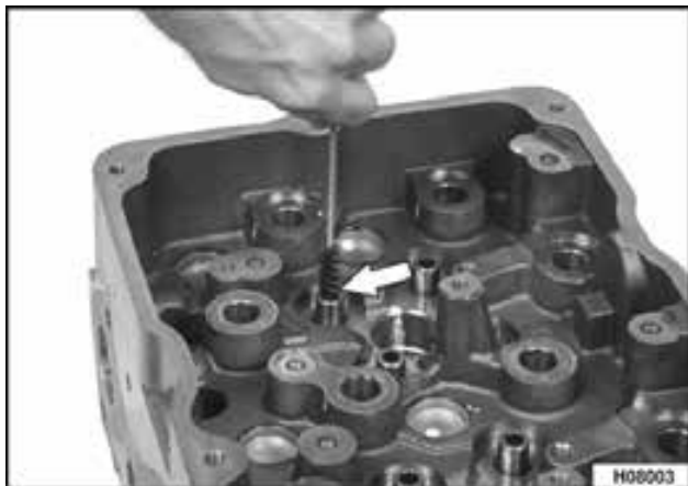
Figure 369 Clean valve guides
