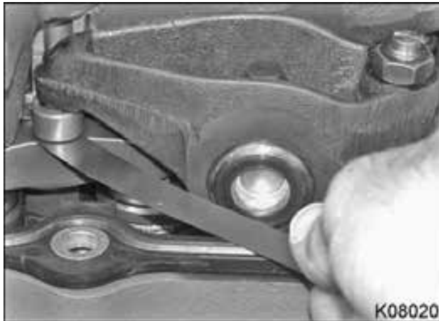
Figure 345 Valve lash measurement
