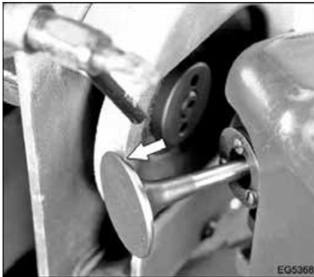
Figure 375 Grind valve face
