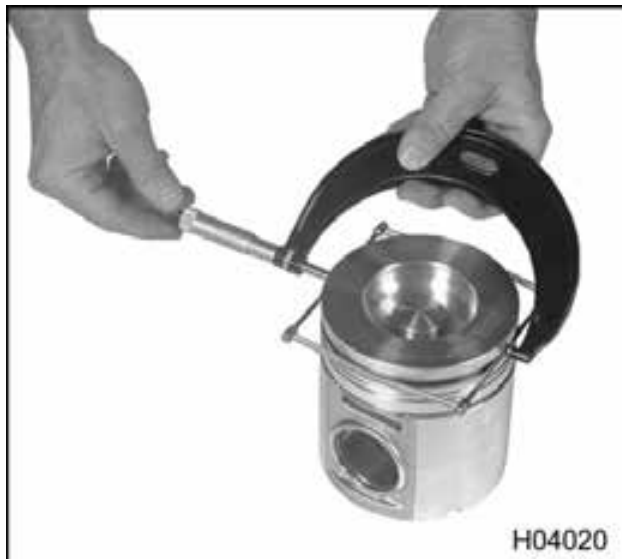
Figure 458 Piston ring groove measurement (top / keystone cross section)
