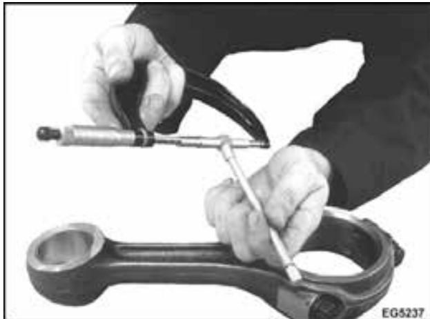
Figure 465 Connecting rod bearing bore taper measurement
