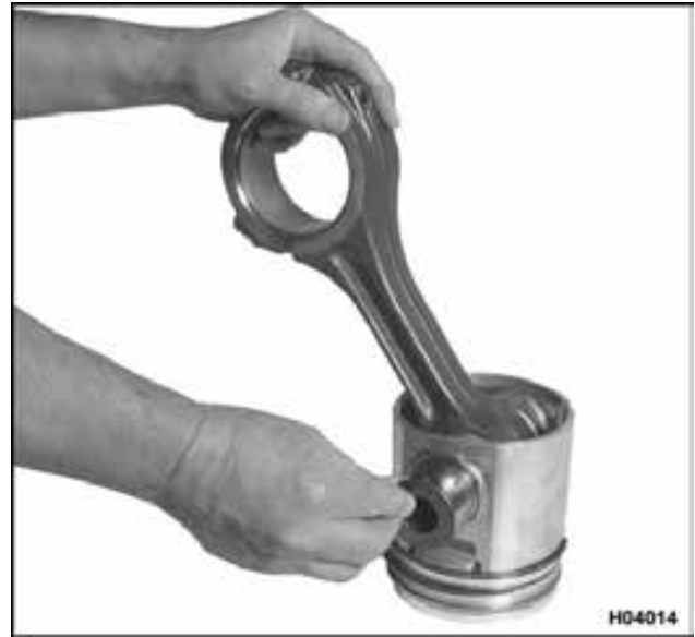
Figure 487 Piston pin installation (typical)
