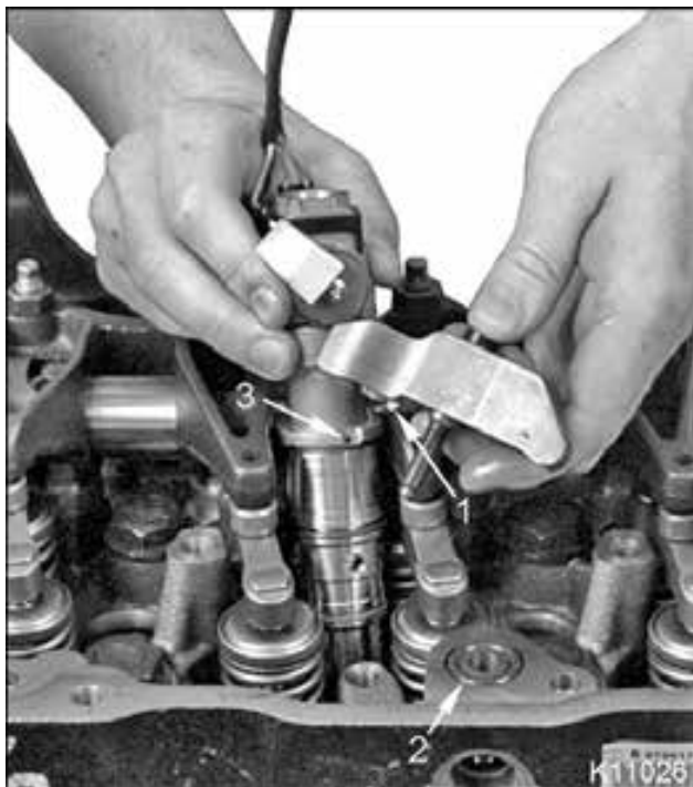
Figure 196 Injector assembly installation
