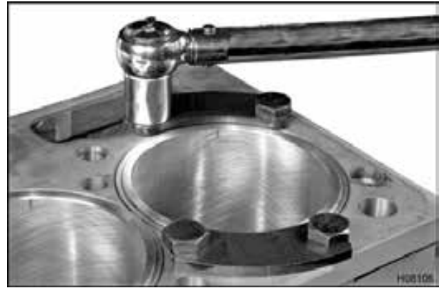
Figure 476 Cylinder Sleeve Holding Adaptor installation
