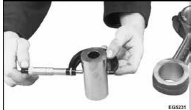
Figure 462 Piston pin measurement
