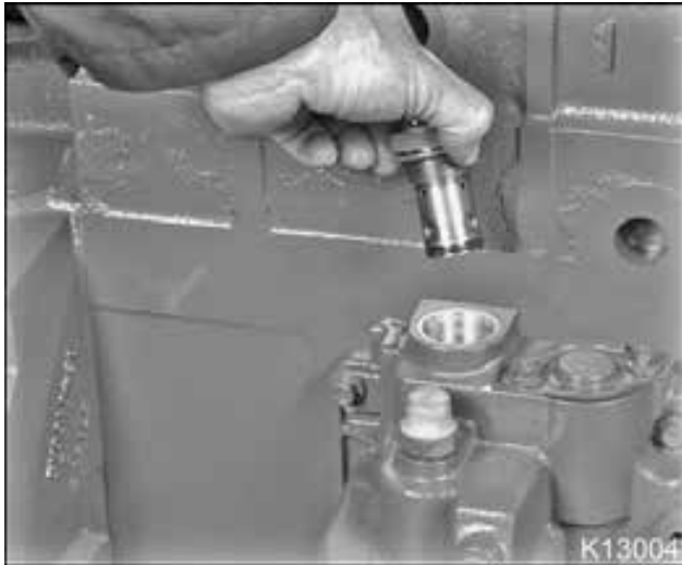
Figure 251 Regulator valve removal
