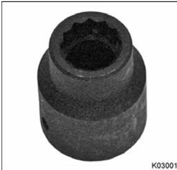
Figure 313 Lower Idler Gear Socket
