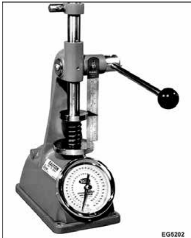
Figure 393 Measure valve spring tension
