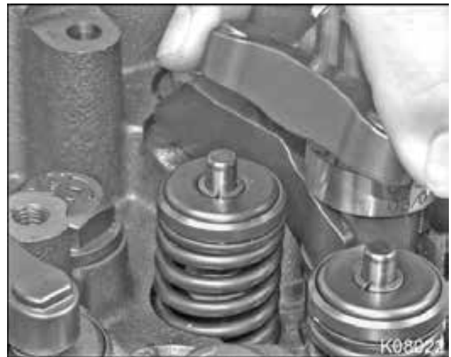
Figure 413 Valve bridge installation
