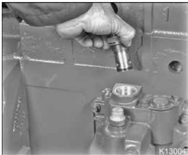
Figure 265 Regulator valve installation
