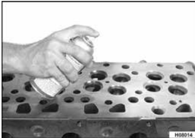
Figure 364 Spray developer on cylinder head
