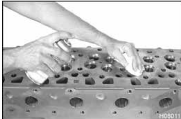
Figure 361 Spray cleaner on cylinder head
