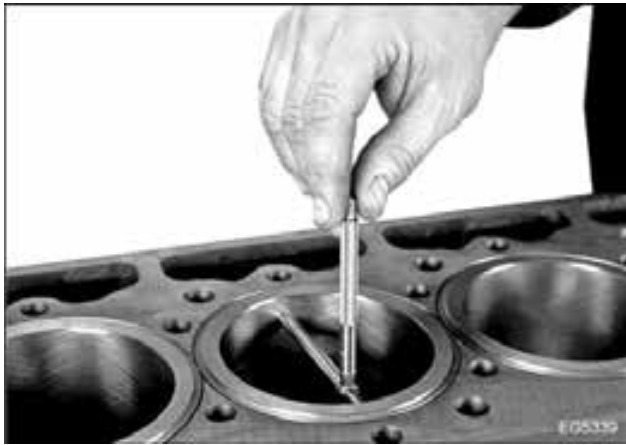
Figure 469 Cylinder sleeve taper measurement
