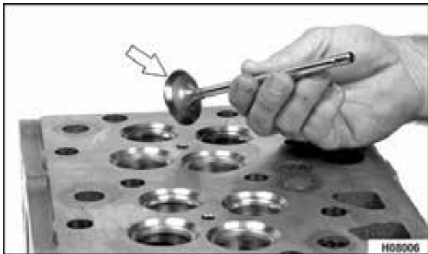
Figure 379 Apply marker paste to valve face
