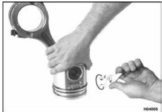
Figure 488 Piston pin retaining ring installation (typical)
