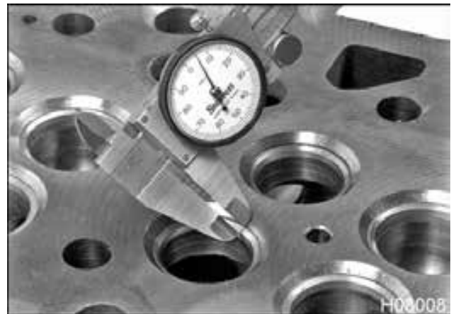
Figure 383 Valve seat width measurement
