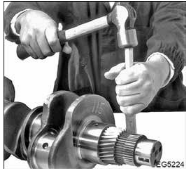
Figure 509 Oil pump spline drive removal
