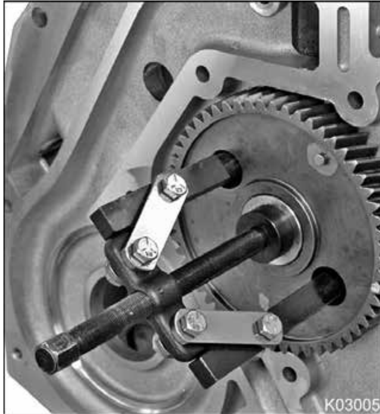
Figure 510 Camshaft gear and Cam Gear Puller
