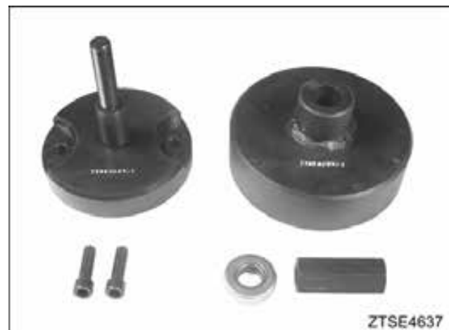
Figure 566 Rear Seal Installer, ZTSE4637
