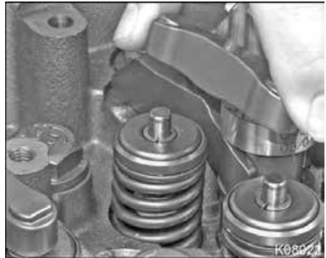
Figure 348 Valve bridge removal
