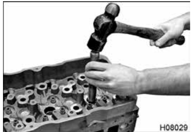
Figure 398 Install fuel injector sleeve
