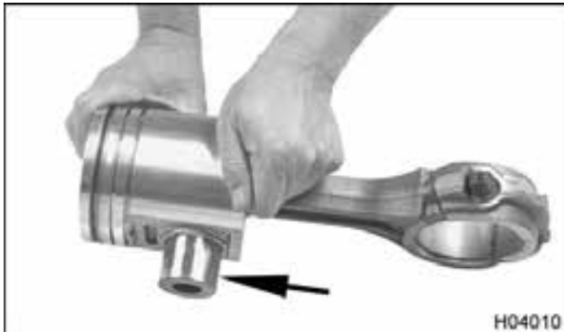
Figure 455 Remove piston pin (typical)
