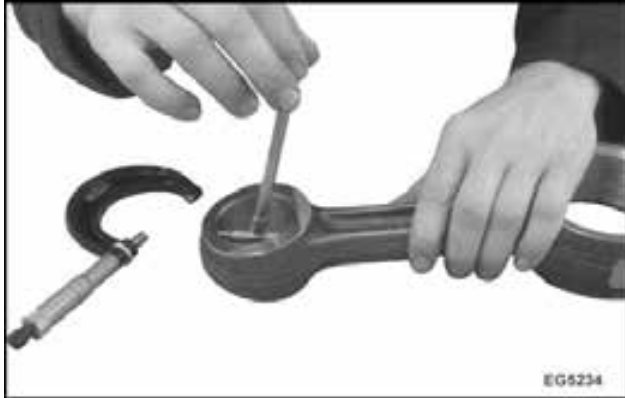
Figure 463 Piston pin bushing measurement
