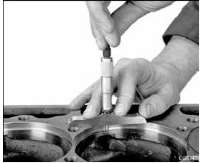
Figure 474 Counterbore depth measurement
