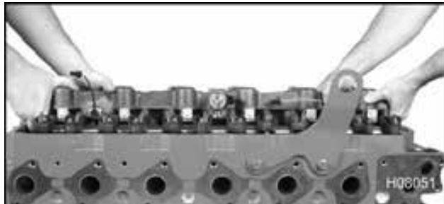
Figure 218 High-pressure oil manifold removal
