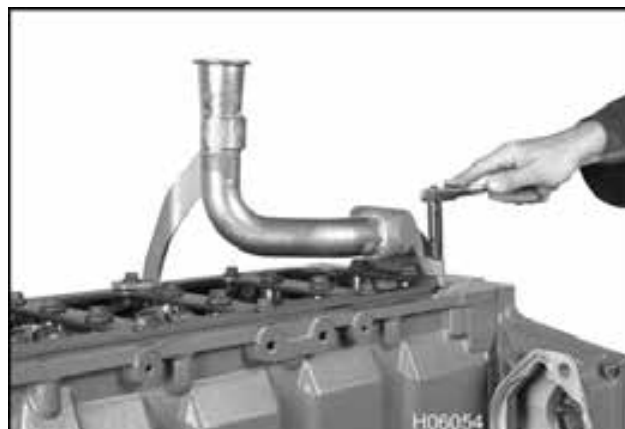
Figure 277 Oil suction tube assembly installation (typical)
