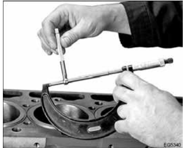
Figure 470 Telescoping gauge measurement
