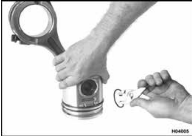
Figure 454 Piston pin retaining ring removal (typical)
