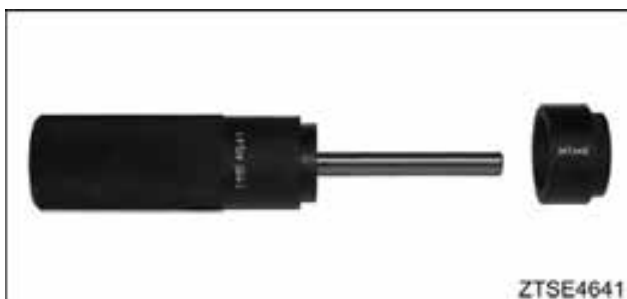
Figure 561 Valve Seat Installer, ZTSE4641
