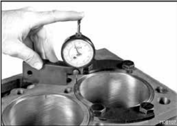
Figure 477 Cylinder sleeve protrusion measurement
