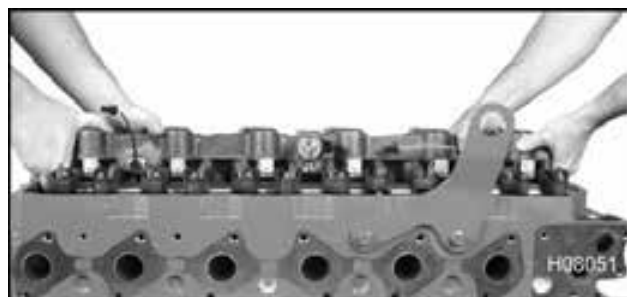
Figure 232 High-pressure oil manifold installation
