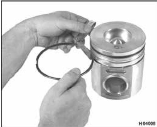
Figure 459 Measure ring groove (typical)
