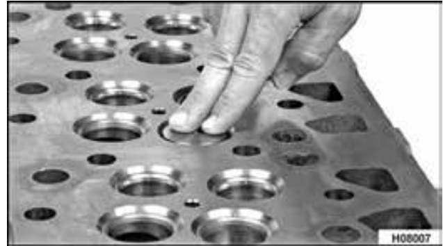
Figure 380 Turn valve on valve seat
