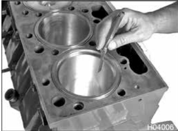
Figure 461 Piston ring end gap measurement
