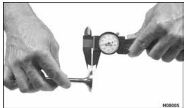
Figure 377 Valve face margin measurement
