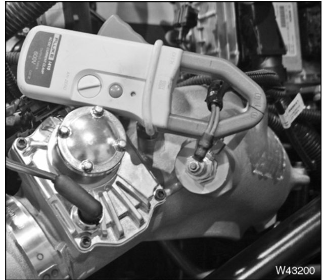
Figure 76 Current clamp on CSFI power circuit
