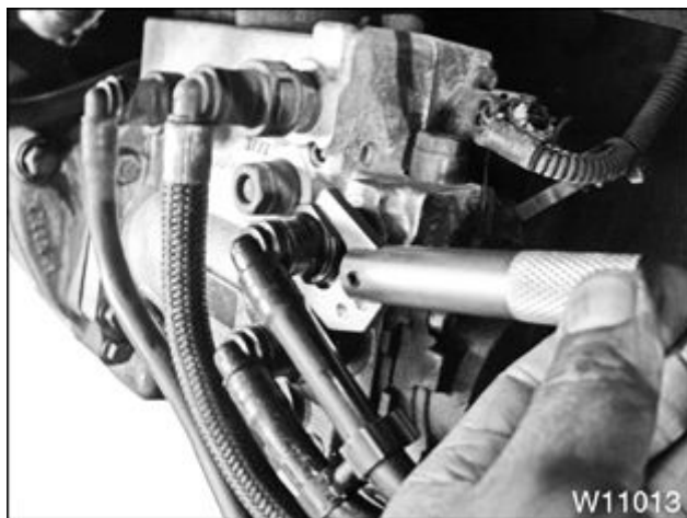
Figure 267 Use of Fuel Line Disconnect Tool
