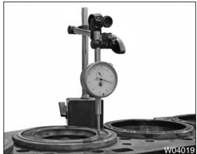
Figure 753 Checking piston protrusion (typical)
