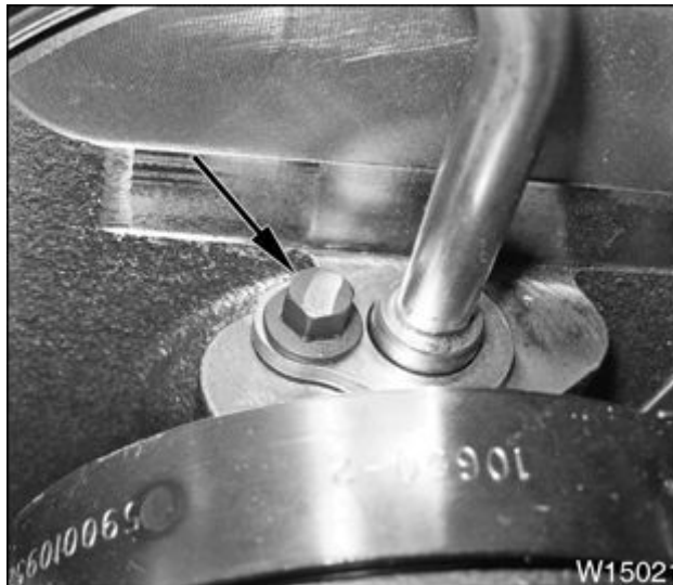
Figure 215 Turbocharger oil supply tube M6 x 12 bolt at high-pressure turbocharger
