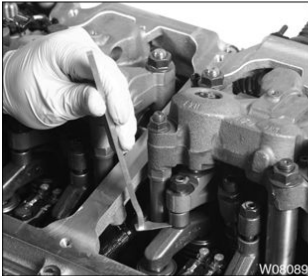
Figure 588 Lash gauge on exhaust valve bridge
