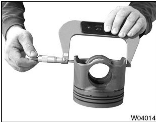
Figure 762 Piston skirt diameter
