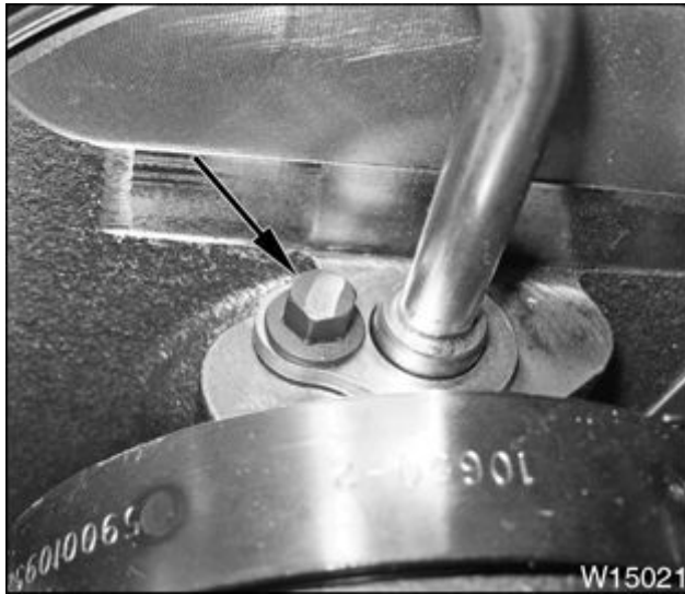
Figure 200 Turbocharger oil supply tube M6 x 12 bolt at high-pressure turbocharger
