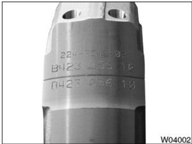
Figure 755 Correct connecting rod and cap joint fit
