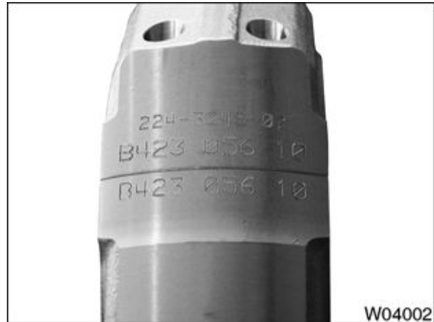
Figure 778 Correct connecting rod and cap joint fit
