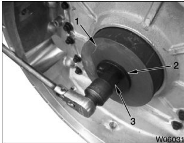
Figure 746 Rear seal installer pressing hub
