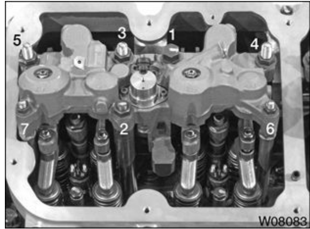
Figure 575 Valve brake actuator assembly torque sequence
