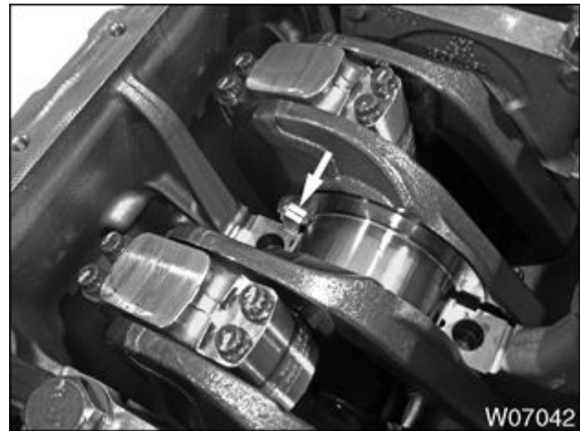
Figure 813 Thrust plate bearing installation
