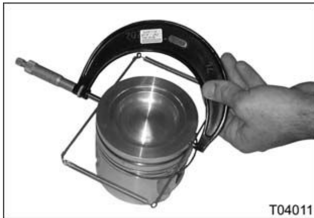
Figure 760 Measuring piston ring groove (top / keystone cross section)
