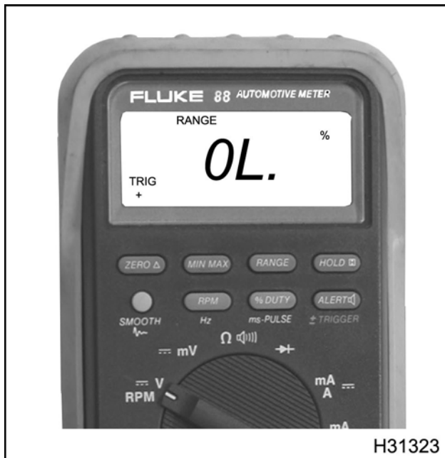
Figure 355 Fluke 88 in duty cycle mode with positive trigger slope
