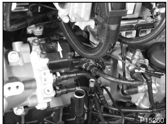
Figure 128 CMP, CKP and FPCV Breakout Harness installed
