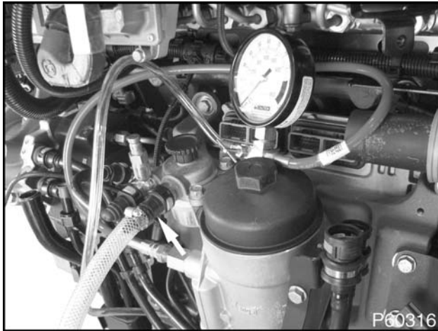
Figure 124 Fuel Inlet Restriction and Aeration Tool installed
