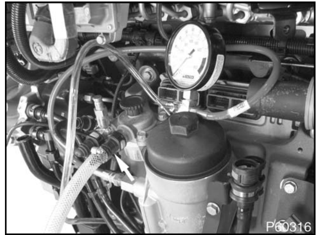
Figure 141 Fuel Inlet Restriction and Aeration Tool installed
