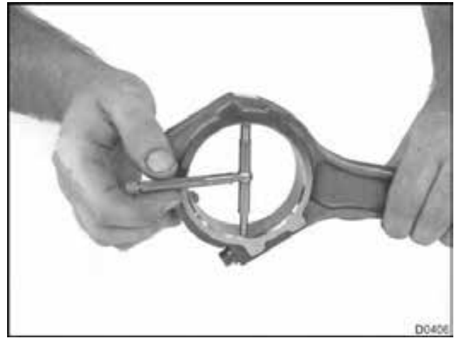
Figure 592 Connecting rod bearing bore out-of-round measurement
