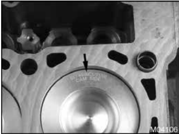
Figure 602 CAM SIDE stamp on piston
