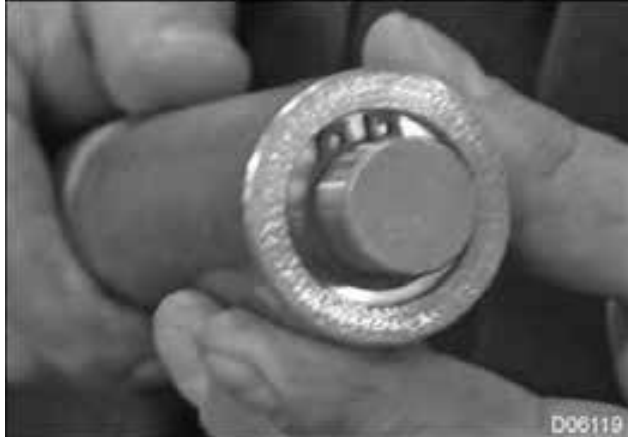
Figure 560 Power steering idler shaft and external retaining ring in Power Steering Idler Shaft Installation Tool
