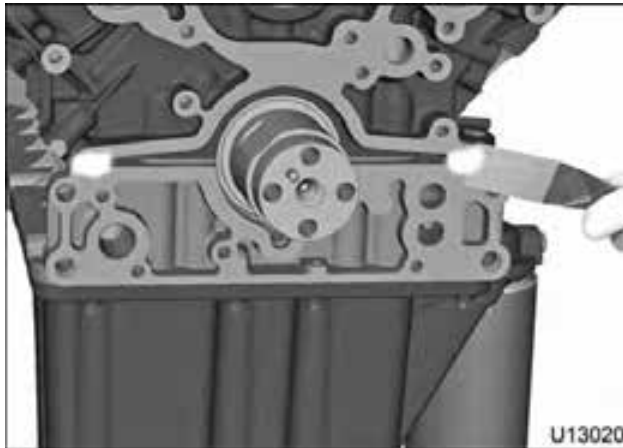
Figure 396 Removal of sealant
