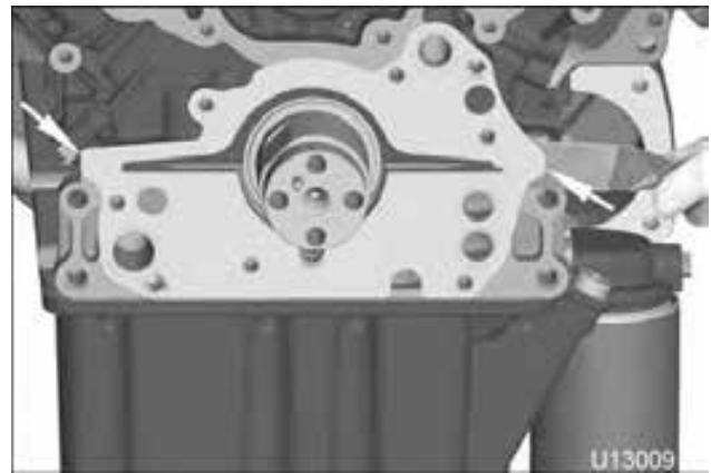
Figure 395 Cutting sealant between oil pump to engine gasket
