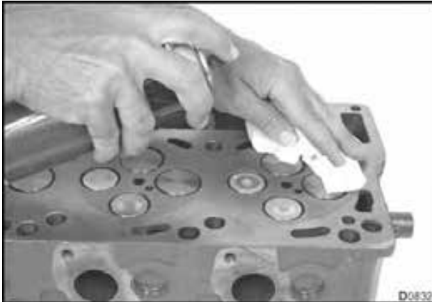
Figure 467 Cleaner sprayed on cylinder head (typical)
