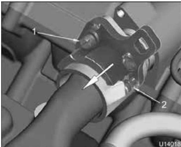
Figure 429 Installation of Cross-over Tube Removal Tool
