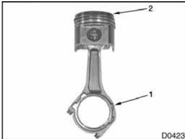
Figure 595 Correct position of installed connecting rod (typical)
