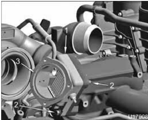
Figure 145 Intake Air Heater (IAH)
