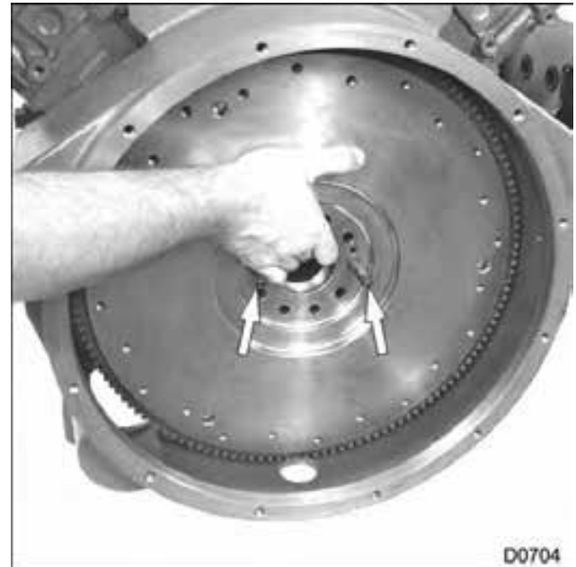
Figure 575 Flywheel assembly installation (typical)
