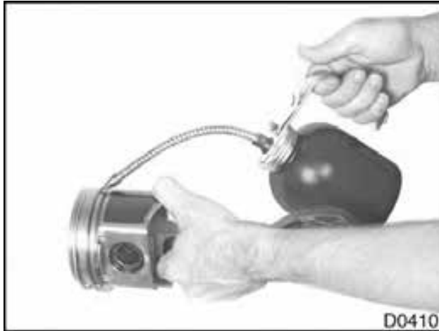
Figure 599 Piston and piston ring lubrication (typical)
