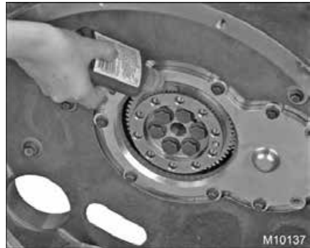
Figure 568 Application of hydraulic sealant
