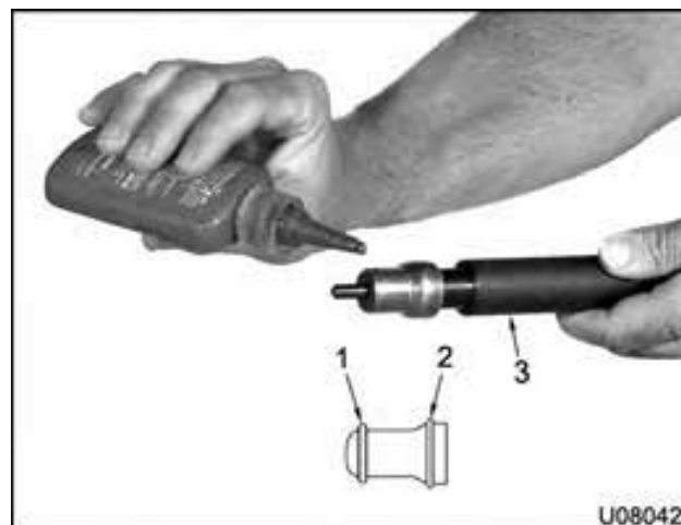
Figure 486 Application of Loctite® 620 Retaining Compound to fuel injector sleeve
