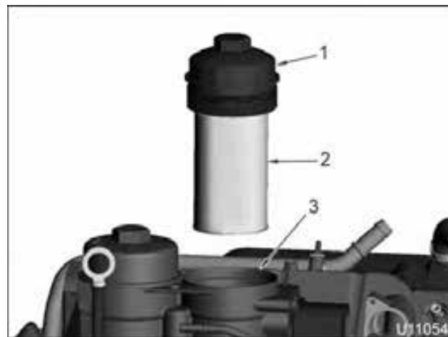
Figure 272 Removal of Secondary fuel filter cap and fuel element filter
