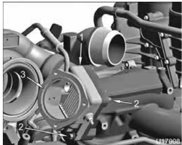
Figure 163 Intake Air Heater (IAH)
