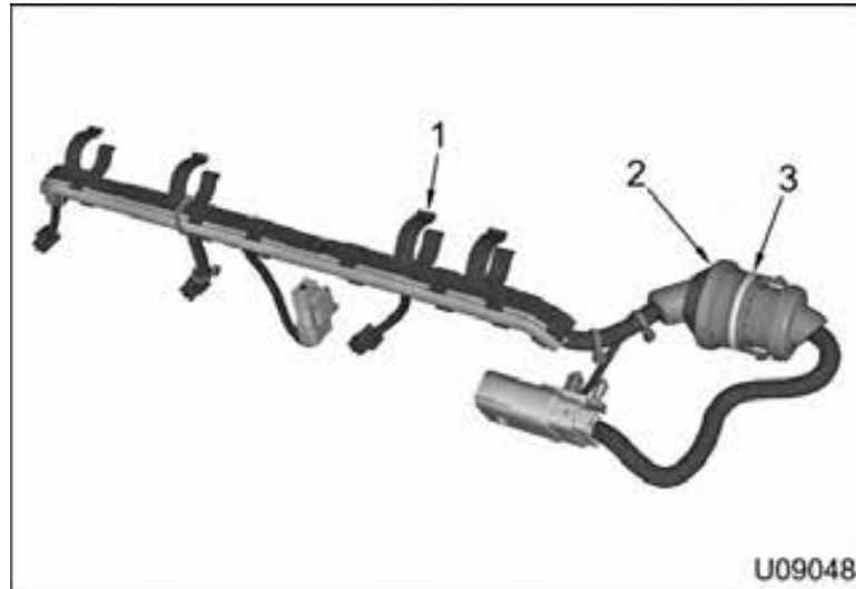
Figure 98 Right Under Valve Cover (UVC) harness
