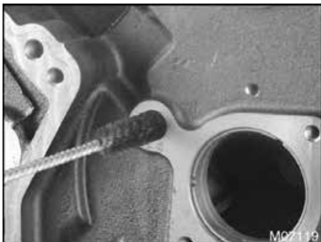
Figure 620 Main oil gallery cleaning
