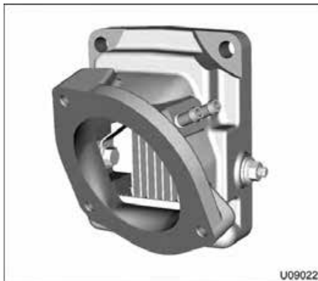
Figure 56 Intake Air Heater (IAH)
