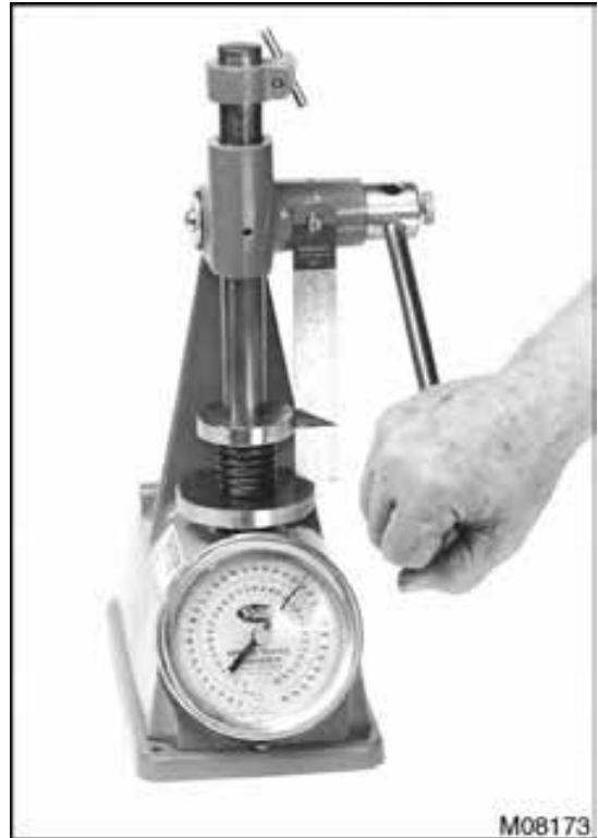
Figure 479 Measurement of valve spring length under load
