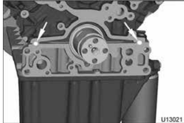
Figure 414 Application of Liquid Gasket (RTV) to Tee joints
