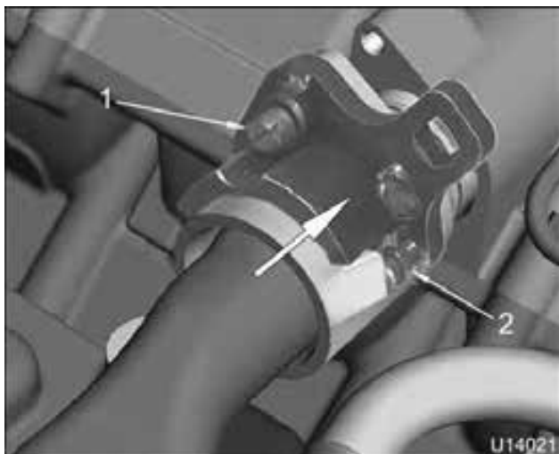
Figure 528 Installation of Cross-over Tube Removal Tool
