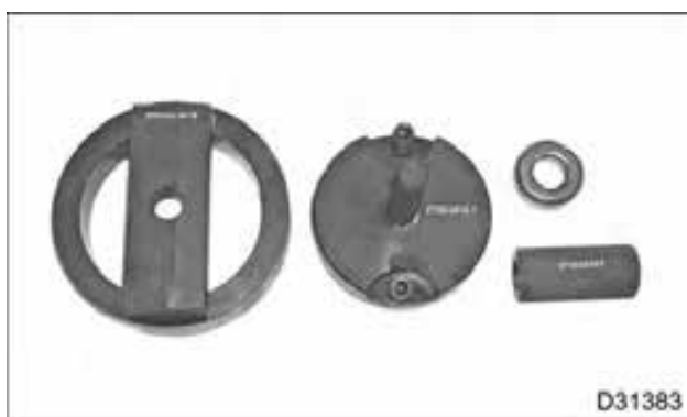
Figure 650 ZTSE4515-2C Rear Seal Installer w/ 40 mm Cap Screws
