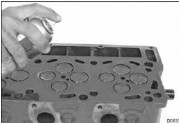
Figure 468 Dye penetrant sprayed on cylinder head (typical)
