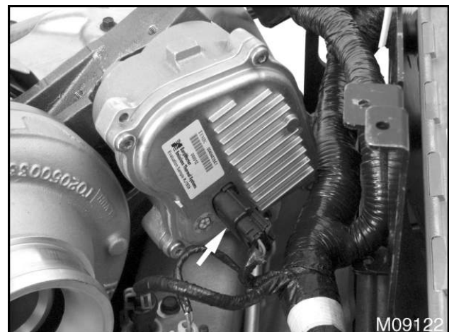
Figure 153 VGT actuator electrical connector
