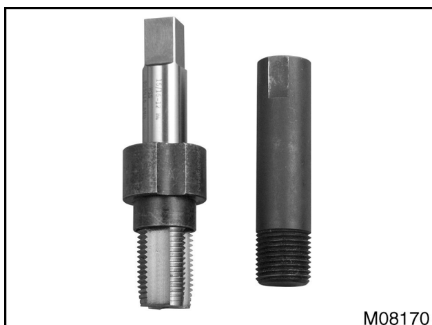
Figure 615 ZTSE4732 Injector Sleeve Remover
