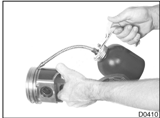
Figure 551 Piston and piston ring lubrication
