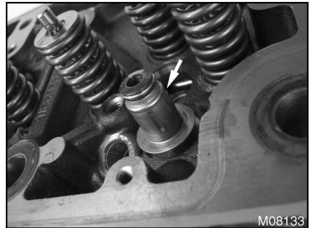
Figure 415 Valve seal assembly (typical)
