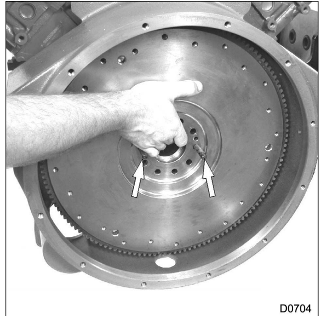
Figure 514 Flywheel assembly installation (typical)
