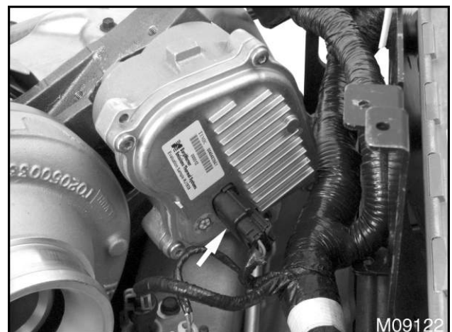
Figure 134 VGT actuator electrical connector
