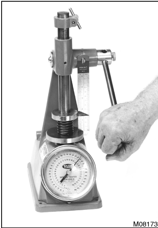
Figure 405 Measurement of valve spring free length under load
