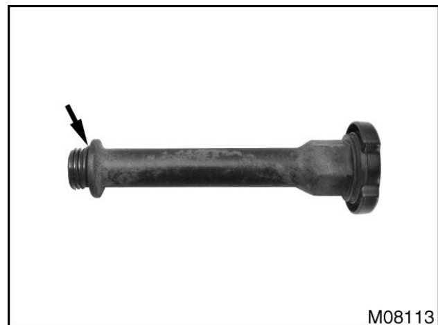
Figure 438 Oil fill extension O-ring seal
