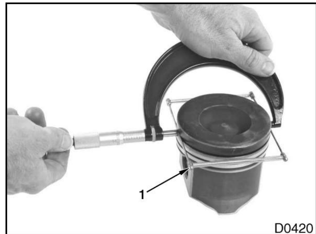
Figure 538 Top compression ring groove
