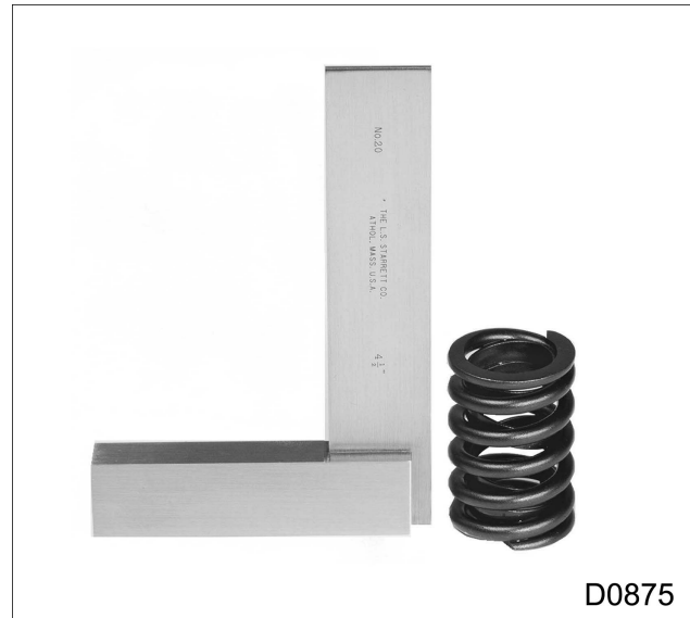
Figure 404 Flatness check of valve spring
