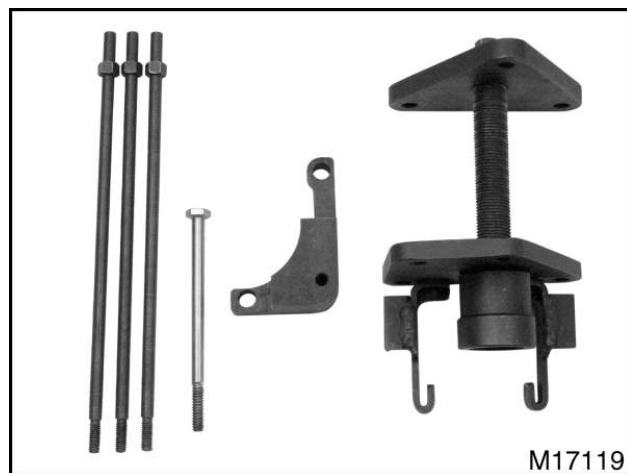
Figure 617 ZTSE4743 EGR Valve Puller
