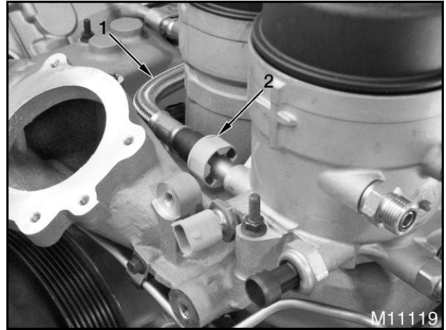
Figure 261 Filter to pump tube assembly connection
