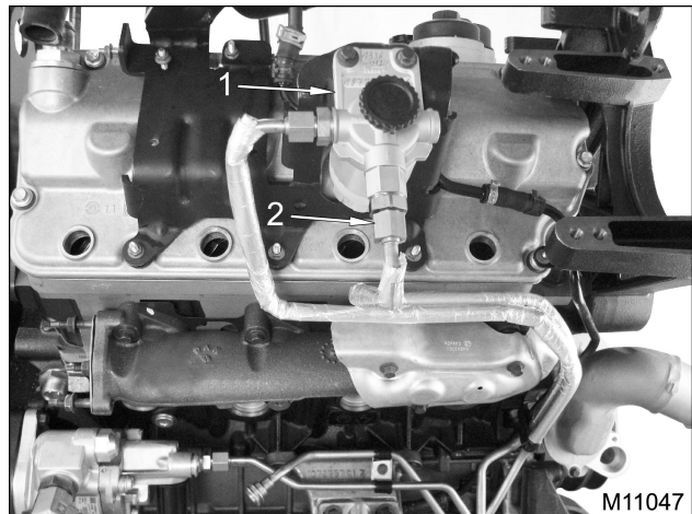
Figure 270 Fuel primer pump assembly tube connections
