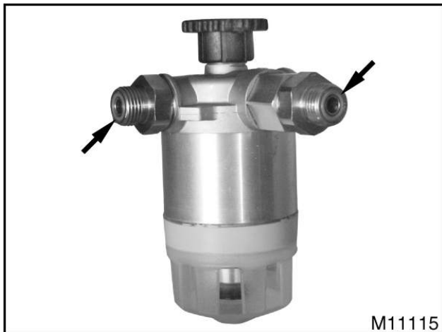
Figure 210 Fuel primer pump assembly O-rings
