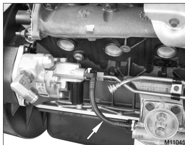
Figure 202 Primary fuel filter to pump tube assembly
