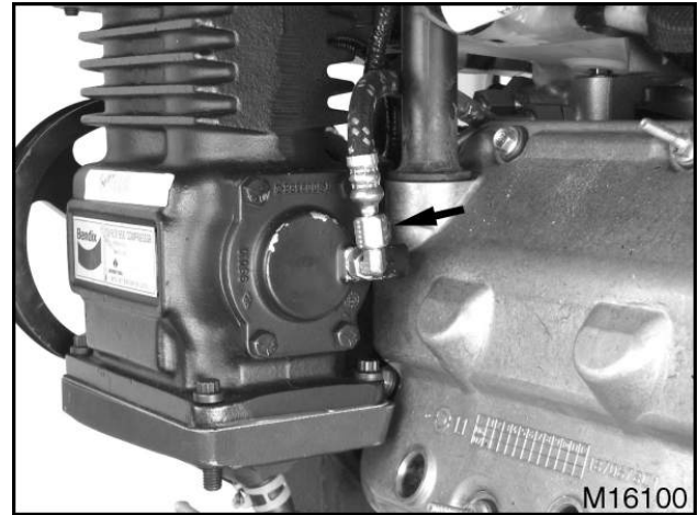
Figure 161 Oil supply hose fitting nut
