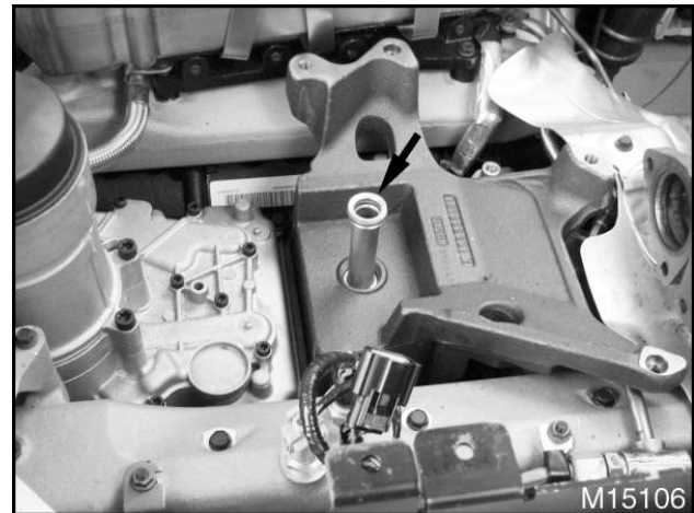
Figure 137 Turbo oil drain tube
