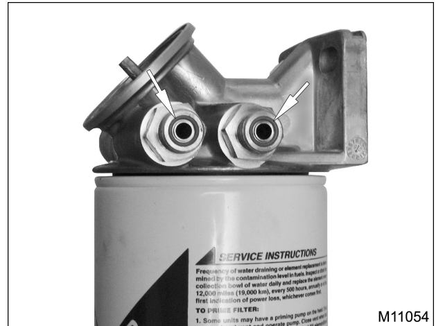
Figure 272 Fuel filter primary header O-rings
