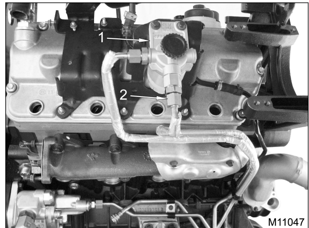
Figure 208 Fuel primer pump assembly tube connections
