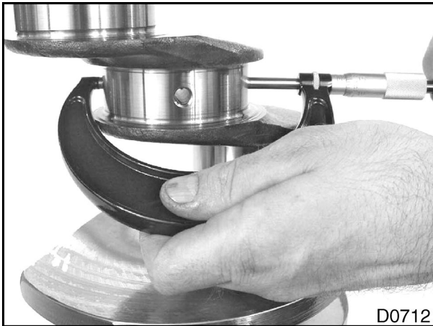
Figure 575 Measurement of crankshaft main journal
