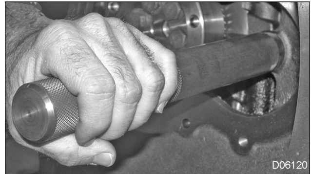
Figure 500 Power steering idler shaft installation
