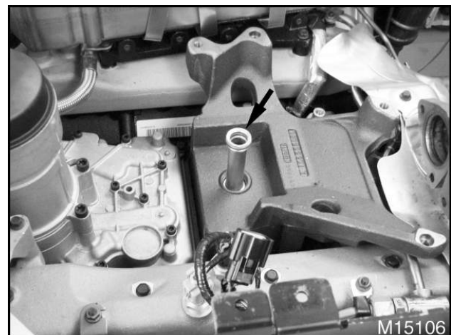
Figure 147 Turbo oil drain tube
