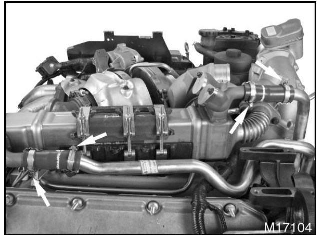
Figure 101 Coolant hose clamps
