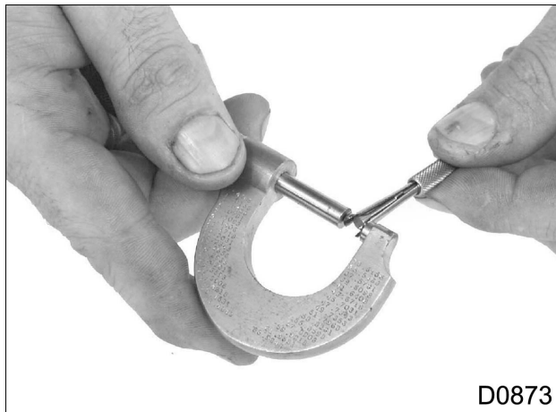
Figure 401 Measurement of Small Hole Gauge (valve guide ID)
