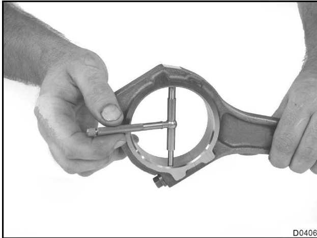
Figure 544 Measurement for out-of-round of connecting rod
