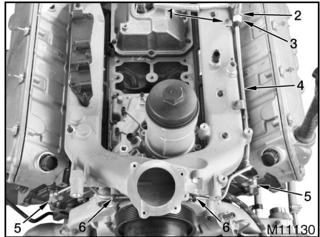
Figure 252 Injector return tube assembly
