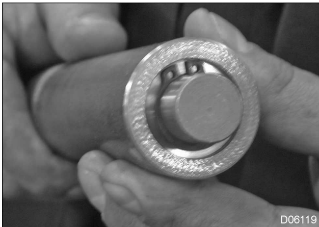
Figure 499 Power steering idler shaft and external retaining ring in Power Steering Idler Shaft Installation Tool
