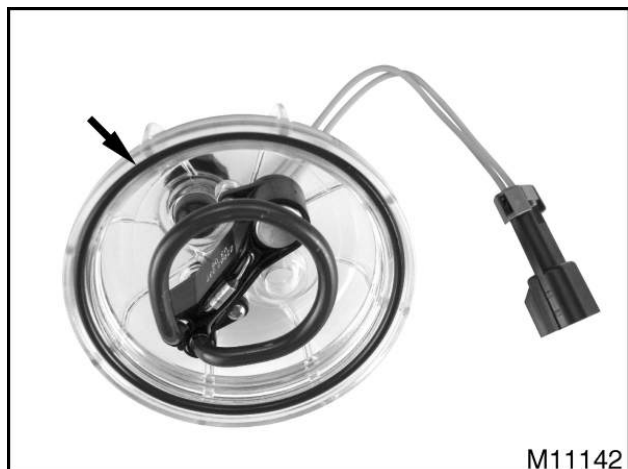
Figure 199 Element and bowl primary filter seal
