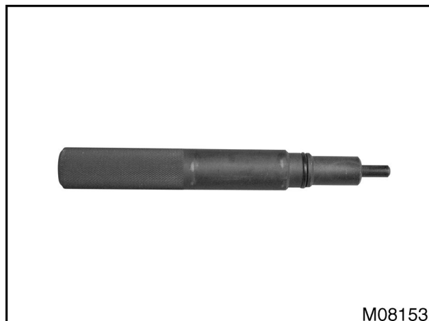
Figure 616 ZTSE473 Injector Sleeve Installer
