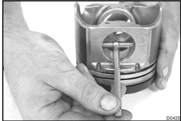
Figure 546 Inside diameter measurement of piston pin bore
