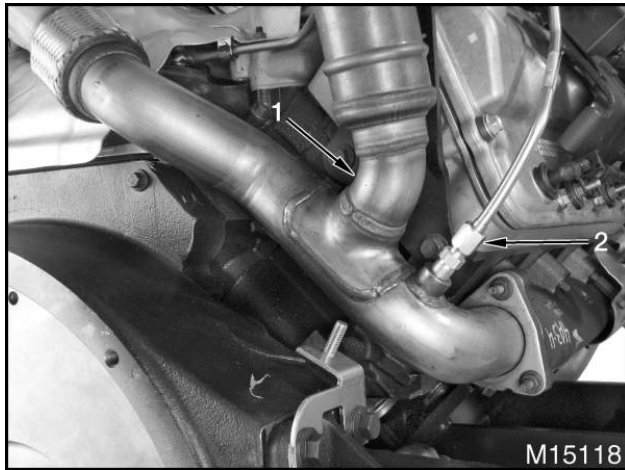
Figure 128 Exhaust Back Pressure (EBP) sensor tube connection
