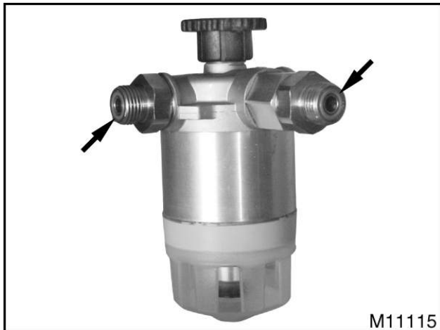
Figure 268 Fuel primer pump assembly O-rings
