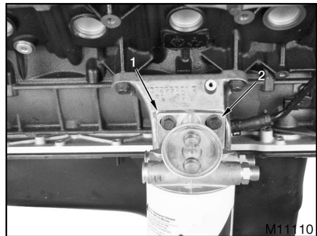
Figure 205 Fuel filter primary header to primary filter bracket support bolts
