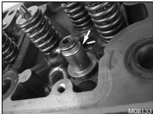
Figure 380 Valve seal assembly (typical)
