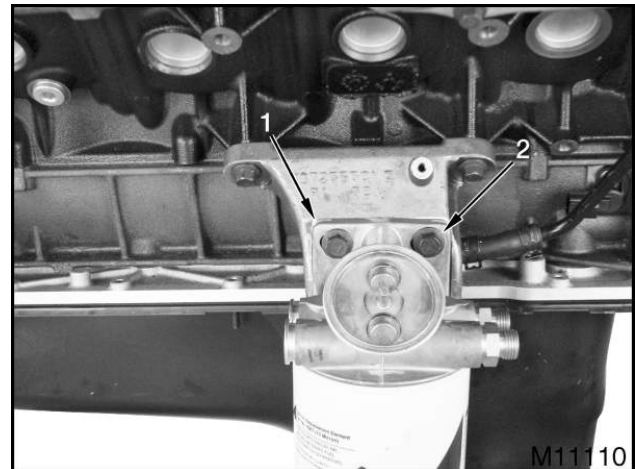
Figure 273 Fuel filter primary header to filter bracket support bolts
