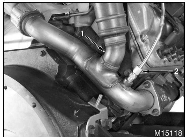
Figure 156 EBP sensor tube connection
