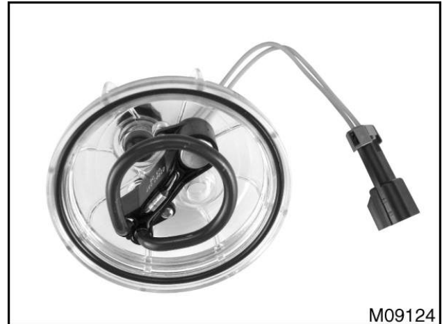
Figure 48 Bowl assembly with fuel heater/probe
