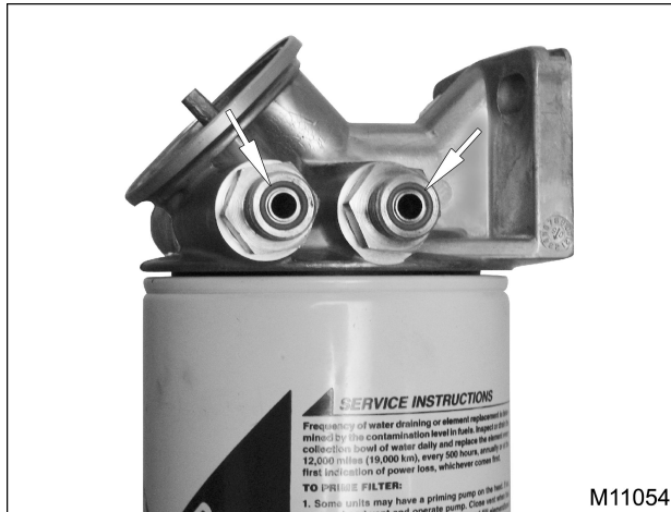
Figure 206 Fuel filter primary header O-rings
