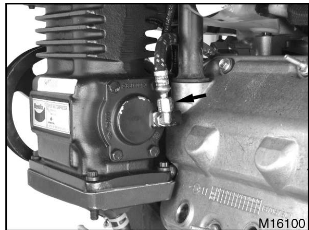
Figure 191 Oil supply hose fitting nut
