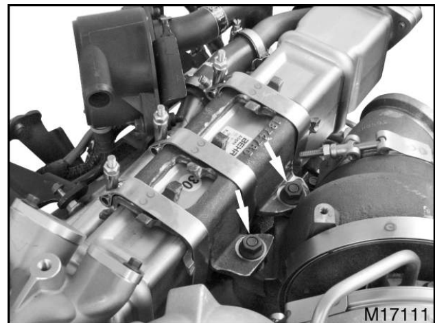
Figure 118 EGR top bracket nuts
