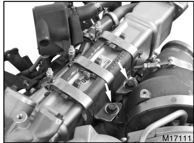
Figure 106 EGR top bracket nuts
