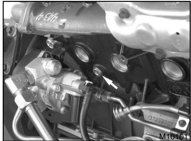
Figure 31 Left side coolant drain plug
