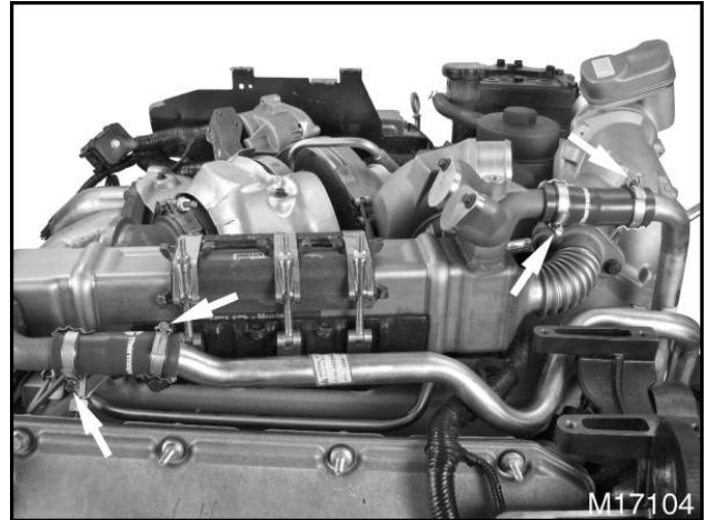
Figure 121 Coolant hose clamps
