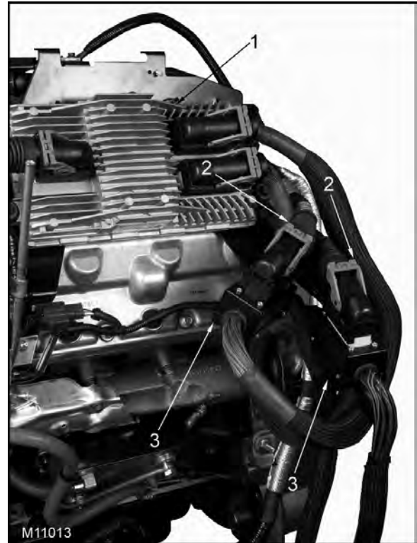
Figure 88 ECM connected to breakout box
