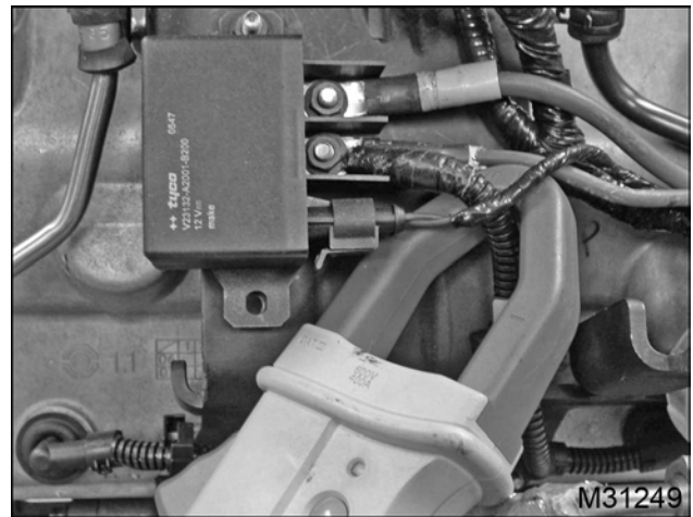
Figure 102 Current clamp around right side glow plug loom
