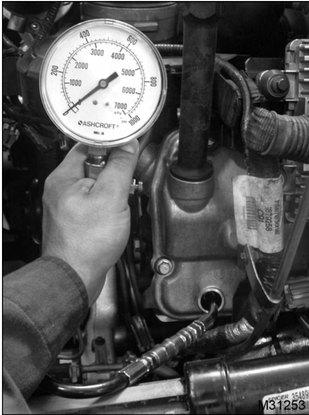
Figure 126 Cylinder Compression Gauge installed
