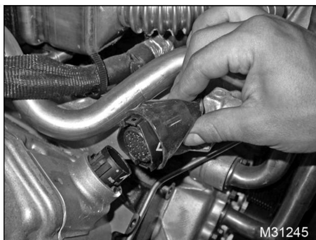
Figure 119 15-pin UVC connector
