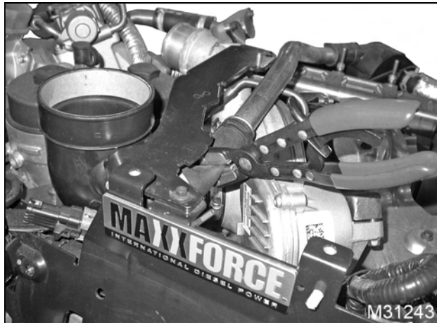
Figure 122 Recirculation tube clamped closed
