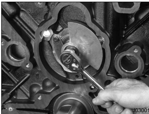
Figure 476 Balance shaft counterweight bolt
