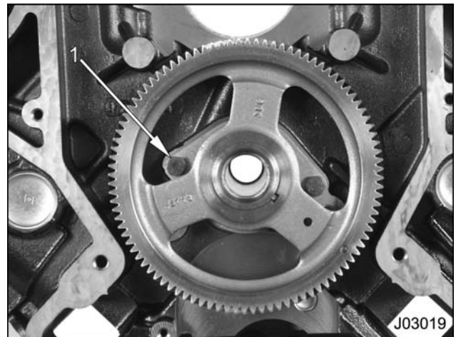
Figure 511 Camshaft thrust plate mounting bolts
