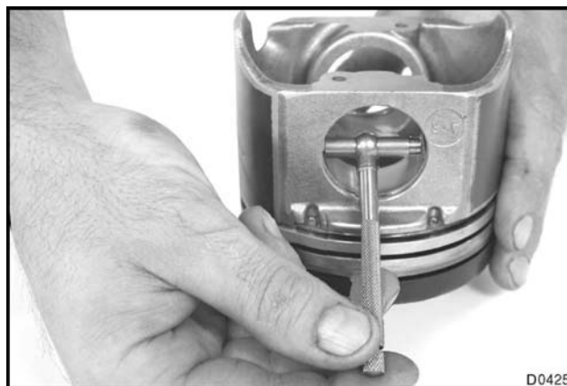
Figure 459 Piston pin bore inside diameter measurement
