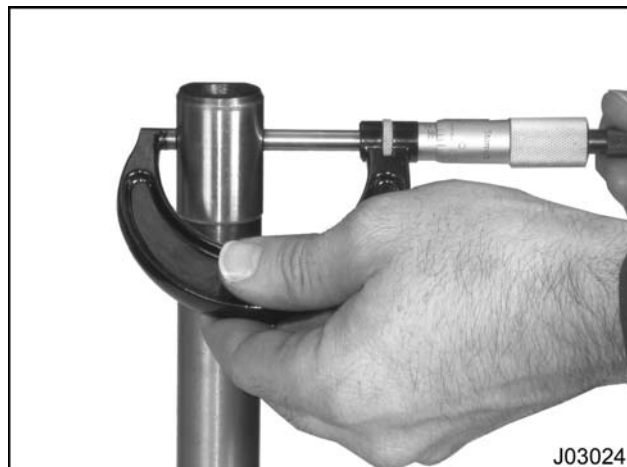
Figure 504 Primary balancer shaft outside diameter measurement
