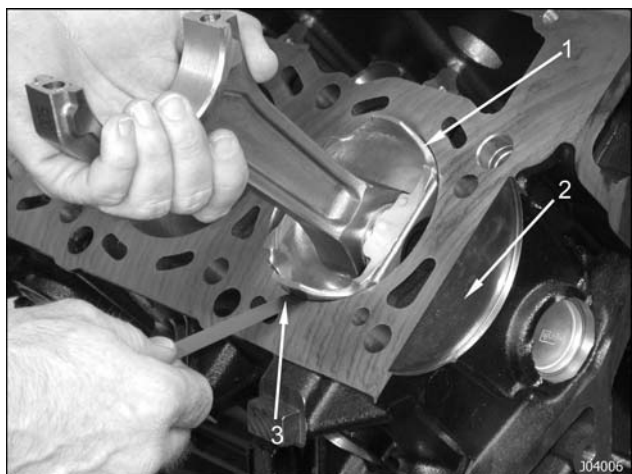
Figure 452 Piston skirt clearance in cylinder bore
