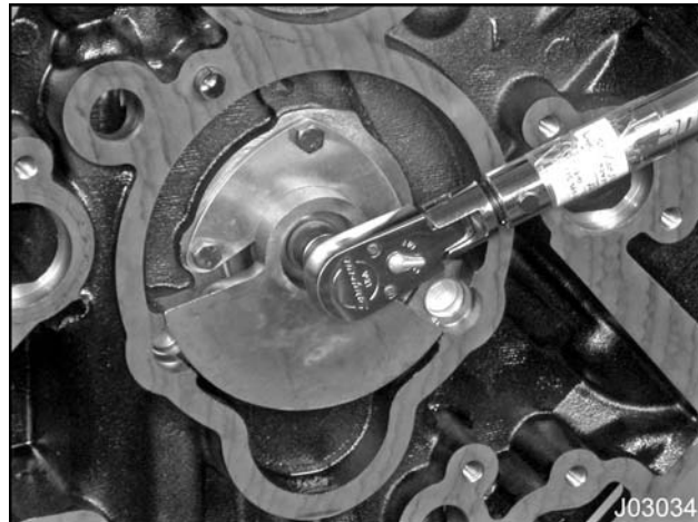
Figure 515 Balance shaft counterweight bolt
