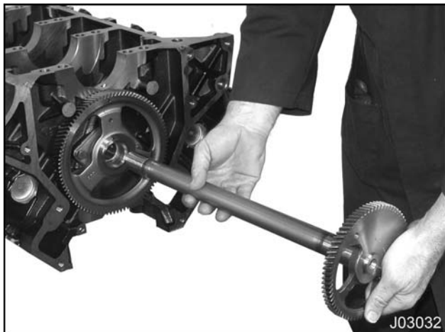
Figure 513 Primary balance shaft installation
