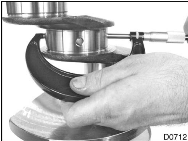
Figure 499 Crankshafts main journal measurement
