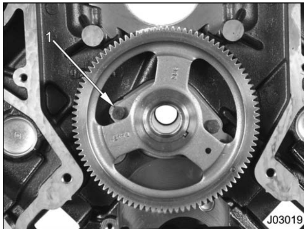
Figure 489 Camshaft thrust plate mounting bolts
