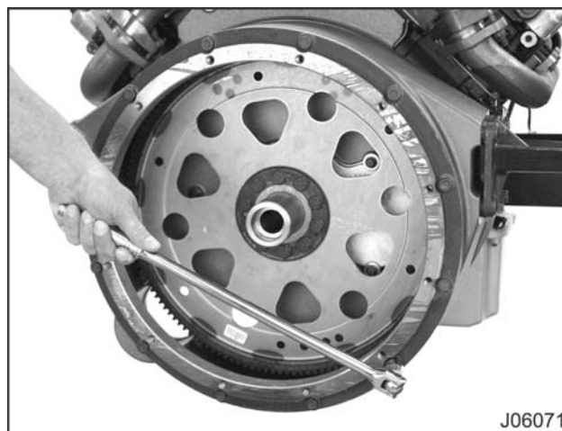
Figure 401 Transmission adapter ring bolt removal (stripped chassis)
