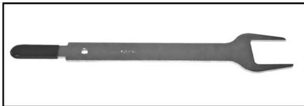
Figure 568 Fan Wrench (pulley bolts), ZTSE4587
