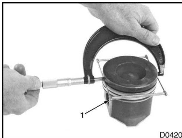
Figure 449 Top compression ring groove measurement
