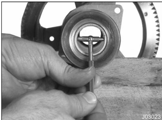
Figure 503 Primary balance shaft bushing inside diameter measurement
