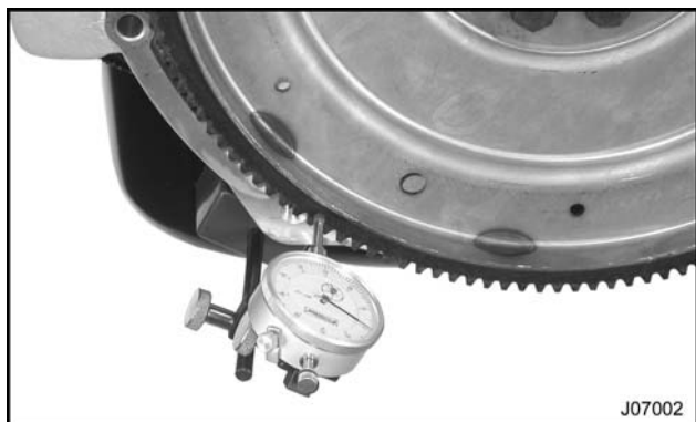
Figure 419 Ring gear run out measurement (typical)
