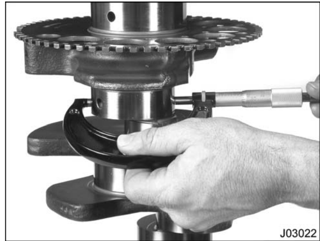
Figure 500 Crankshaft connecting rod journal measurement
