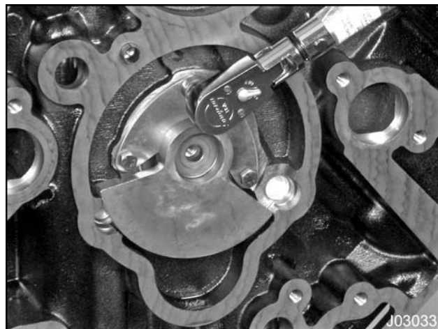
Figure 514 Balance shaft thrust plate bolts
