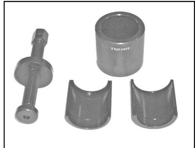
Figure 556 Front Wear Sleeve Remover, ZTSE4517
