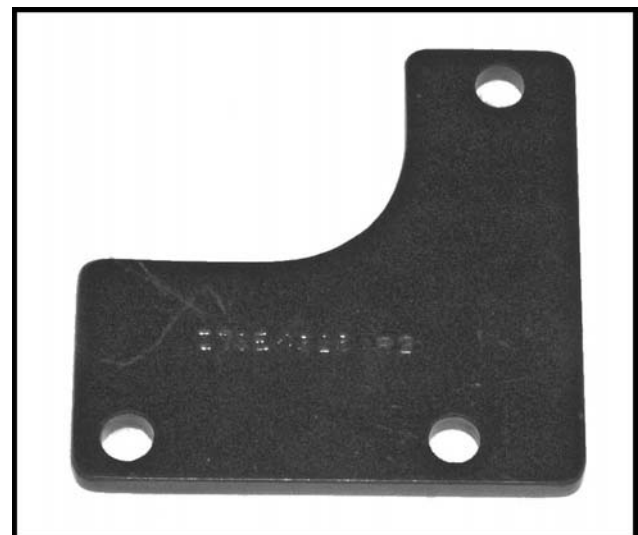
Figure 558 Oil Cooler Test Plate / Pressure Adapter, ZTSE4525
