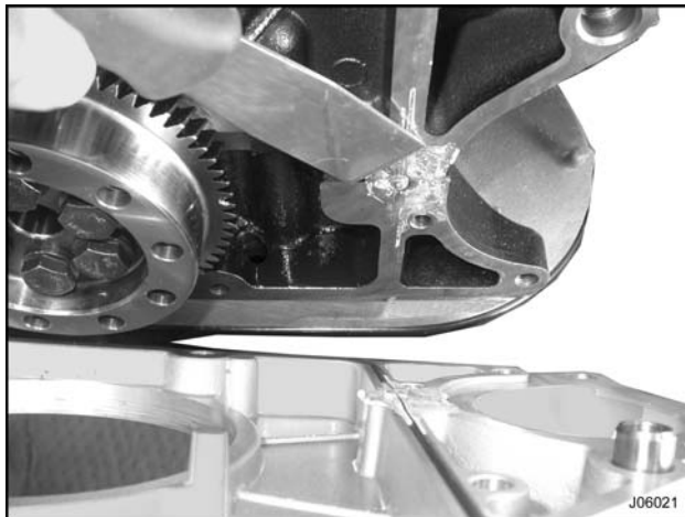
Figure 416 Rear cover and lower crankcase sealant cut location (typical)
