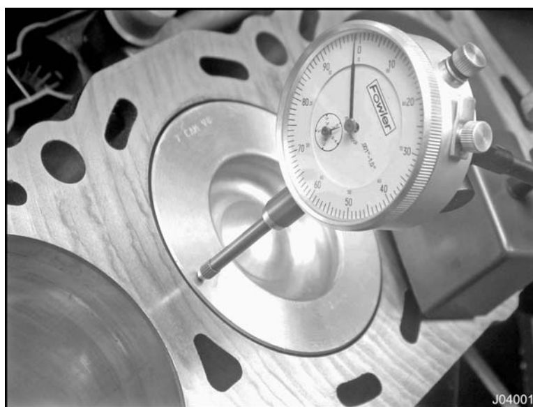
Figure 442 Piston protrusion measurement
