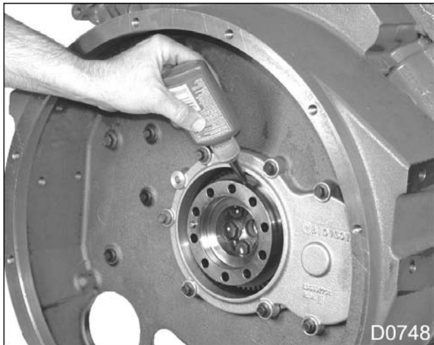
Figure 436 Sealant application to crankshaft secondary flange
