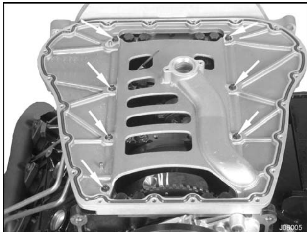
Figure 268 Upper oil pan mounting bolts (CityStar™)
