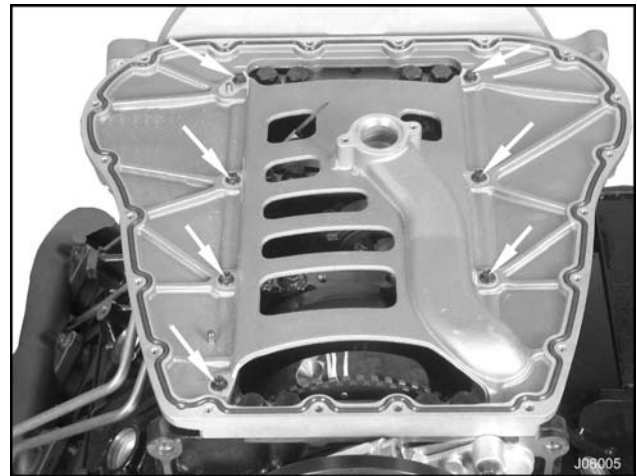
Figure 274 Upper oil pan mounting bolts (CityStar™)
