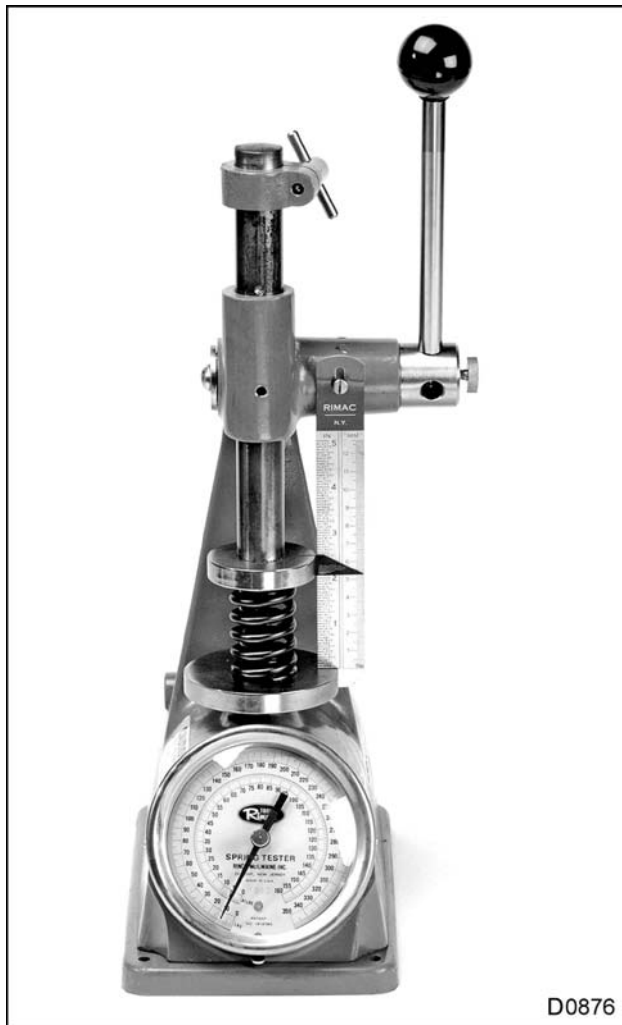
Figure 354 Check valve spring free length
