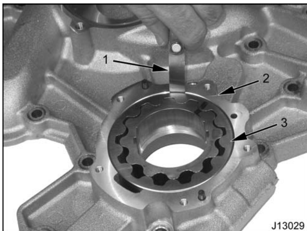
Figure 297 Inspect gerotors for wear
