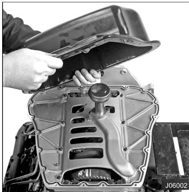
Figure 266 Lower oil pan removal (typical)
