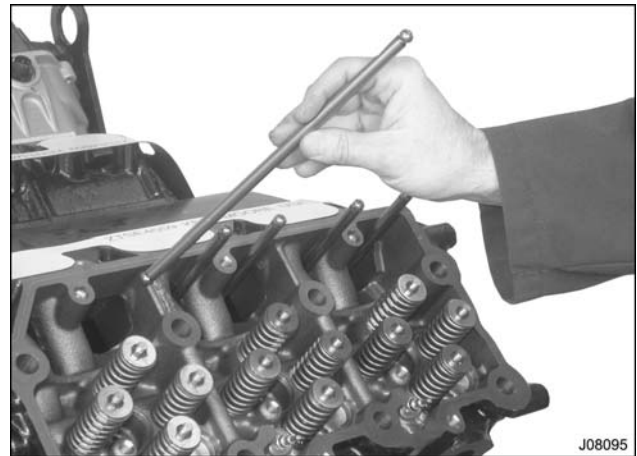
Figure 324 Push rod removal
