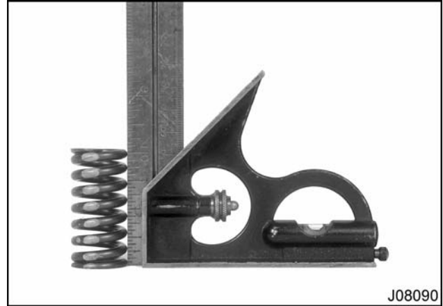
Figure 353 Check the squareness of each valve spring
