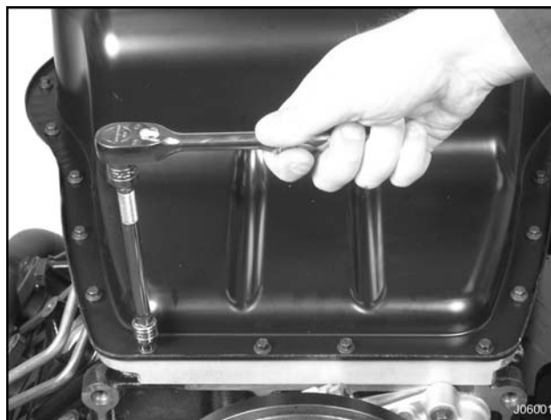
Figure 264 Lower oil pan mounting bolts
