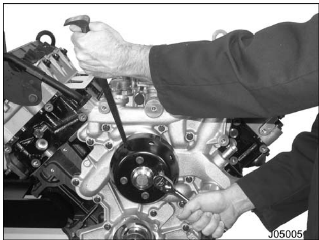
Figure 289 Water pump / fan drive pulley removal
