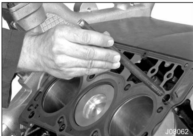
Figure 388 Guide pin installation
