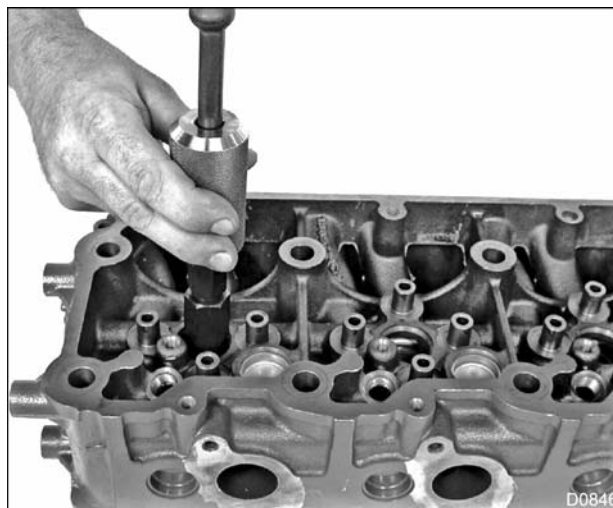
Figure 357 Injector Sleeve Remover and slide hammer
