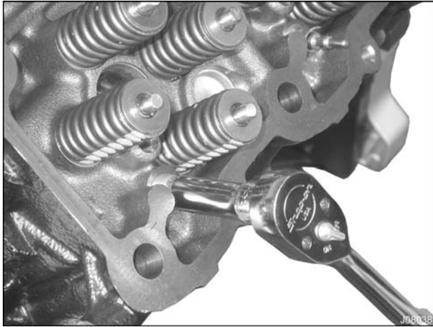
Figure 325 Glow plug removal
