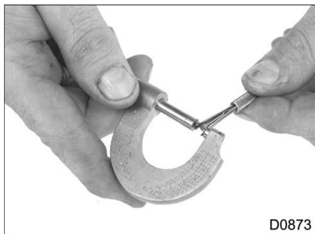
Figure 349 Measuring the small hole gauge (valve guide ID)
