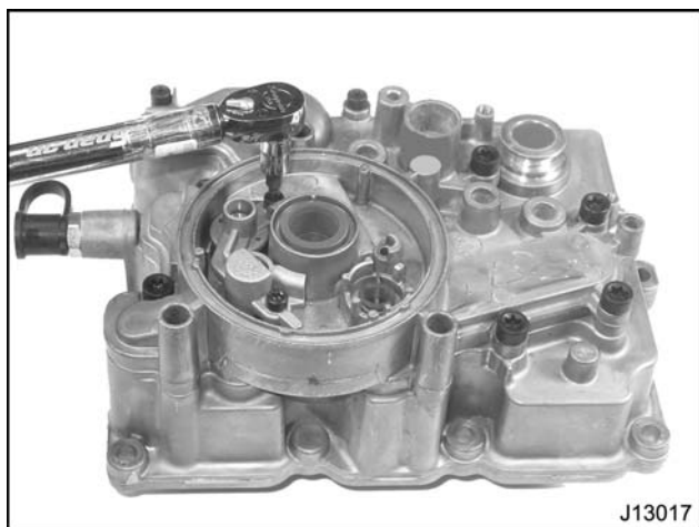
Figure 250 Oil bypass / filter inlet guide screws
