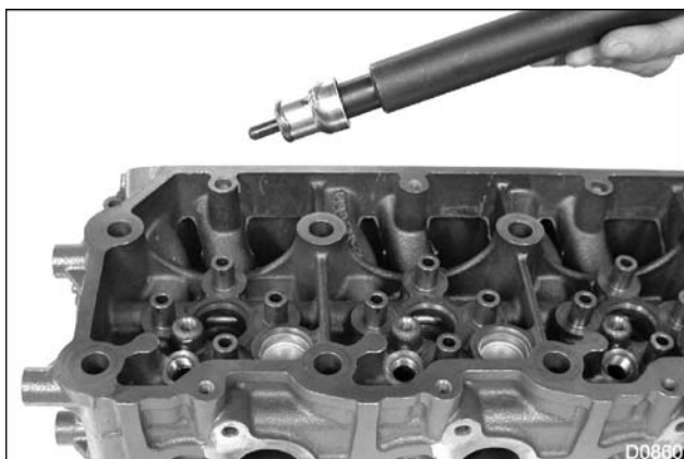
Figure 363 Installing fuel injector sleeve
