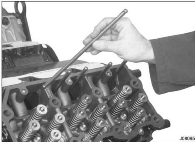
Figure 390 Installing push rod
