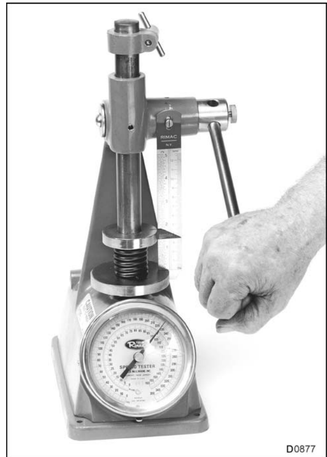
Figure 355 Measuring valve spring length under load
