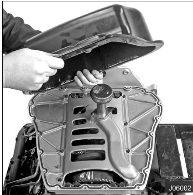
Figure 277 Lower oil pan installation (typical)
