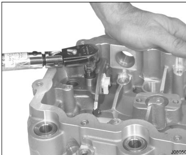
Figure 382 Installing an end rocker fulcrum plate
