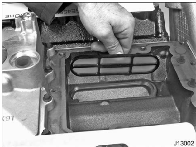
Figure 239 High-pressure oil pump inlet strainer
