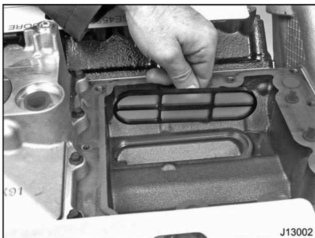
Figure 254 Pump inlet strainer
