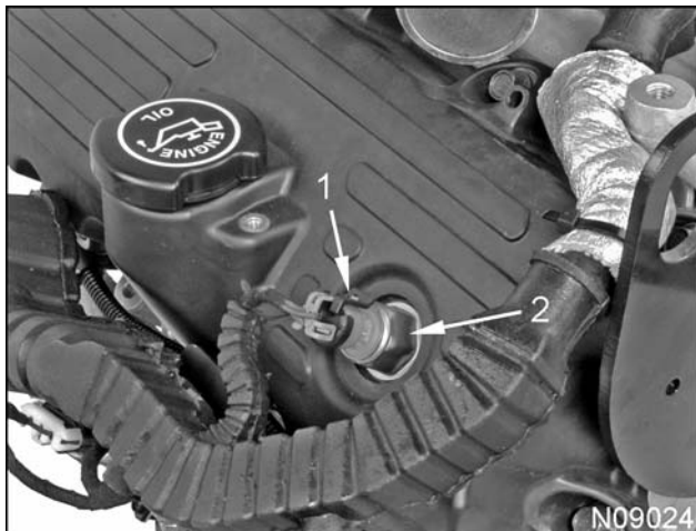
Figure 101 ICP sensor and harness connector
