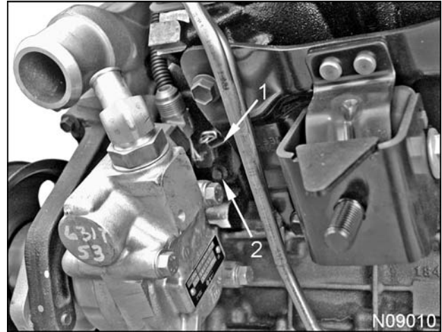
Figure 74 CMP sensor and harness connector
