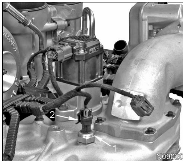
Figure 106 MAP sensor and harness connector
