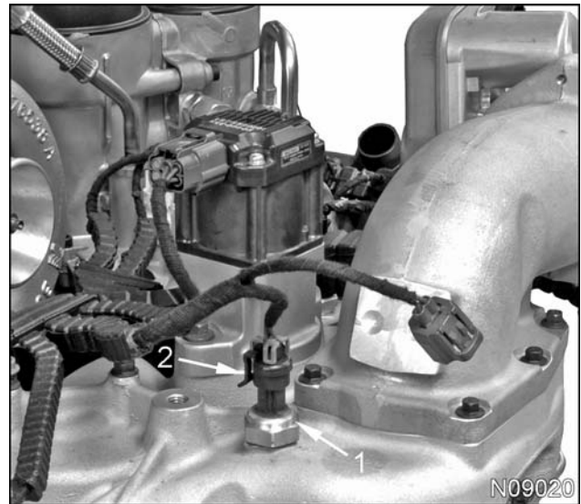
Figure 85 MAP sensor and harness connector
