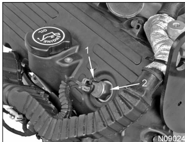
Figure 89 ICP sensor and harness connector
