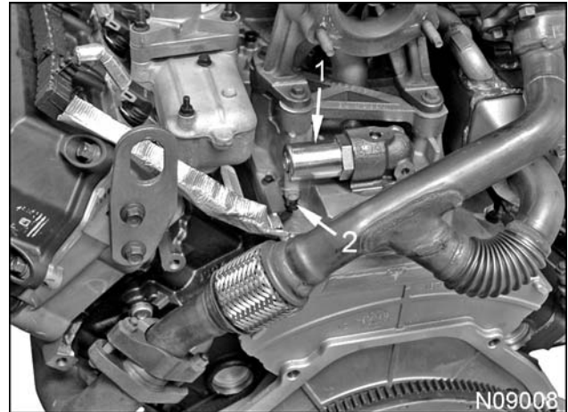
Figure 72 IPR valve and harness connector (connector heat shield removed)
