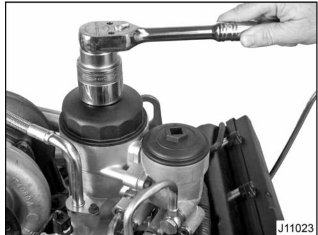
Figure 44 Oil filter cap removal
