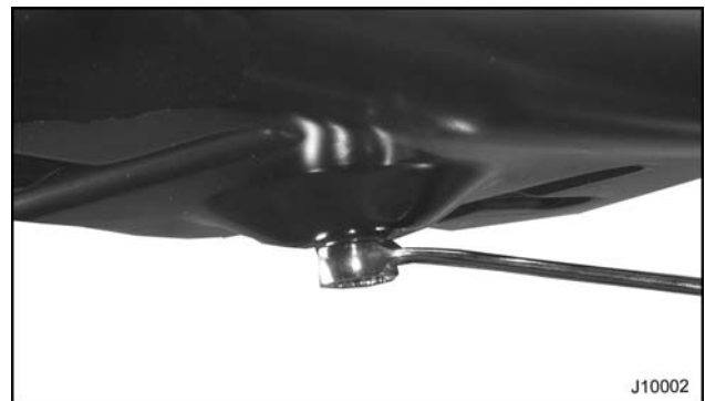
Figure 45 Oil drain plug removal
