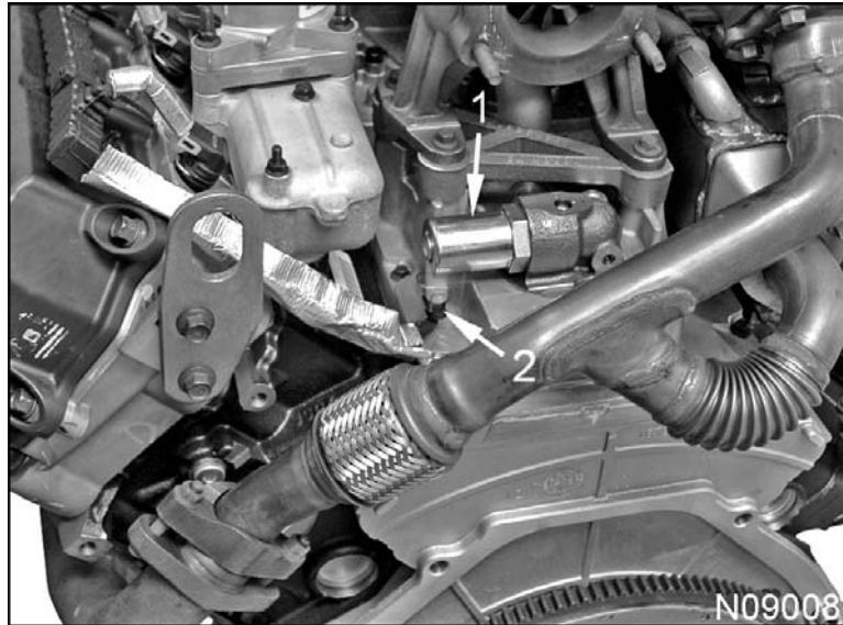
Figure 120 IPR valve and harness connector (connector heat shield removed)
