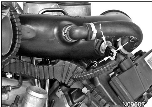
Figure 121 IAT sensor and harness connector
