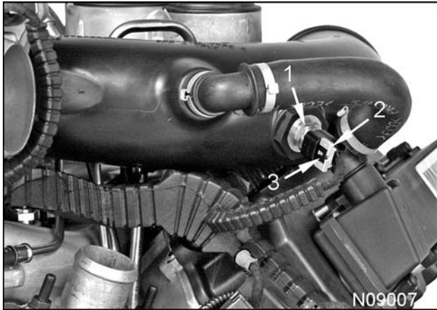
Figure 71 IAT sensor and harness connector
