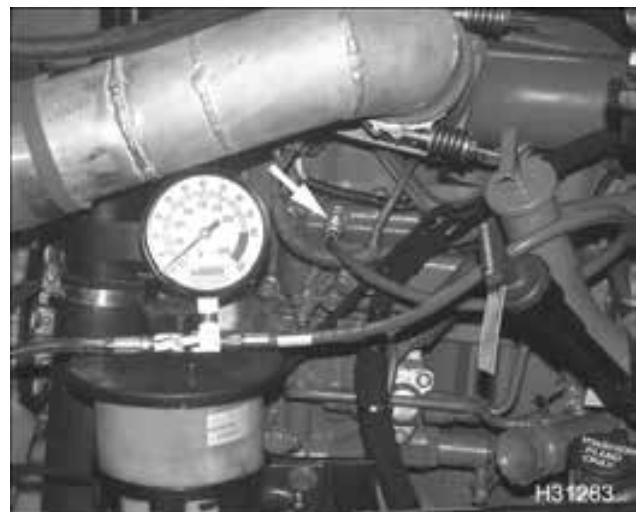
Figure 291 Fuel Pressure Gauge to fuel pressure test adapter
