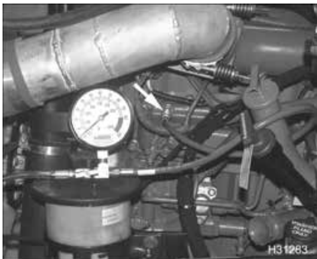
Figure 216 Fuel Pressure Gauge to fuel pressure test adapter
