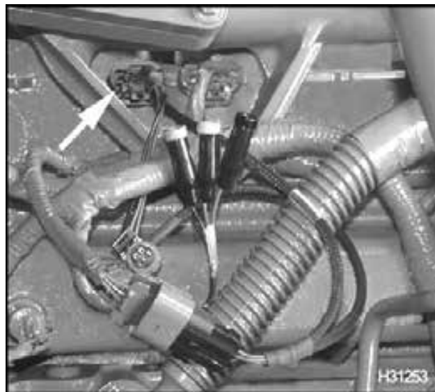
Figure 314 VC Gasket Breakout Harness to pass-through connector for BCP sensor
