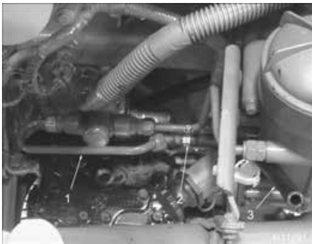
Figure 220 Test hose to fuel line
