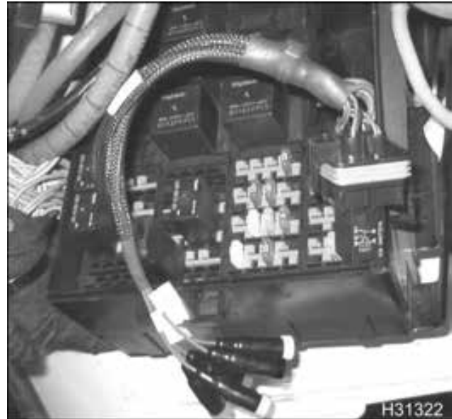
Figure 204 Relay Breakout Harness to power distribution center
