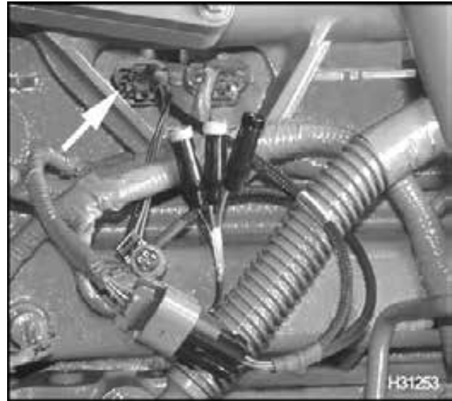
Figure 354 VC Gasket Breakout Harness to pass-through connector for BCP sensor
