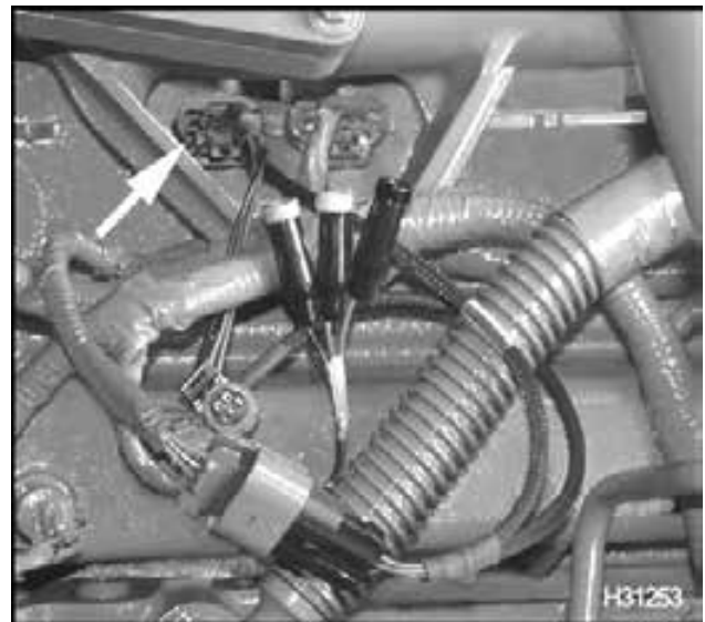
Figure 186 VC Gasket Breakout Harness to pass-through connector for BCP sensor
