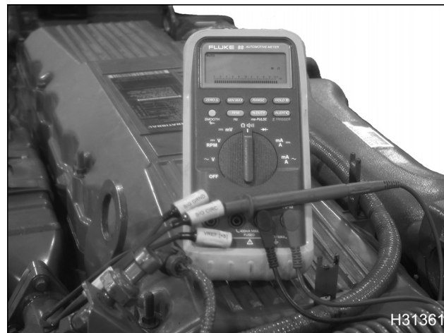
Figure 371 Resistance check to ECM chassis ground
