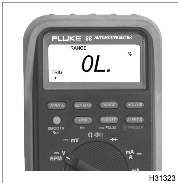
Figure 563 FLUKE 88 in duty cycle mode with positive trigger slope
