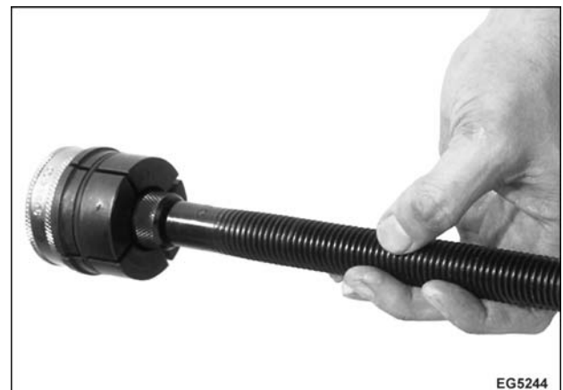
Figure 377 Camshaft bushing installation tool
