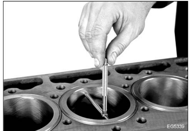
Figure 321 Checking cylinder sleeve inside diameter with telescoping gauge
