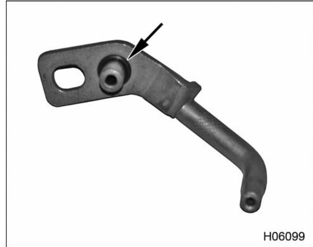
Figure 300 O-ring (underside) of new piston cooling tube
