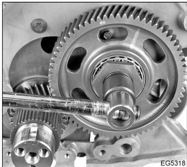
Figure 236 Removing the lower idler gear
