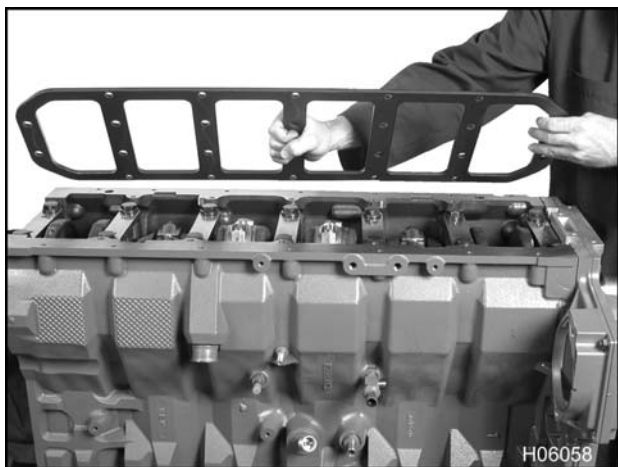
Figure 363 Removing the crankcase ladder
