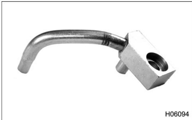
Figure 298 Old piston cooling tube
