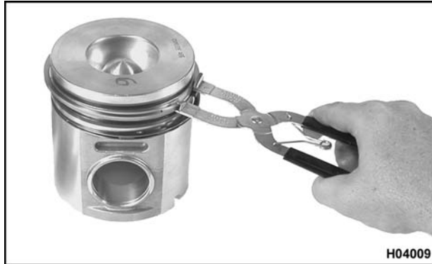
Figure 337 Installing piston rings (466 piston shown)
