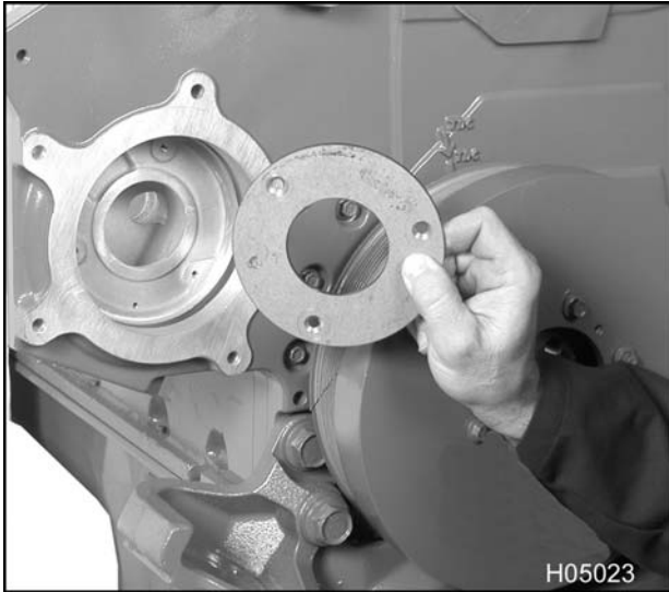
Figure 271 Water pump wear plate (Generation 1 front covers only)
