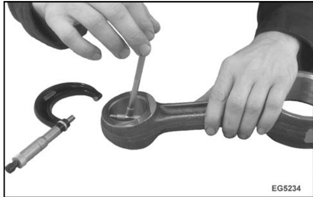
Figure 315 Measuring piston pin bushing inside diameter
