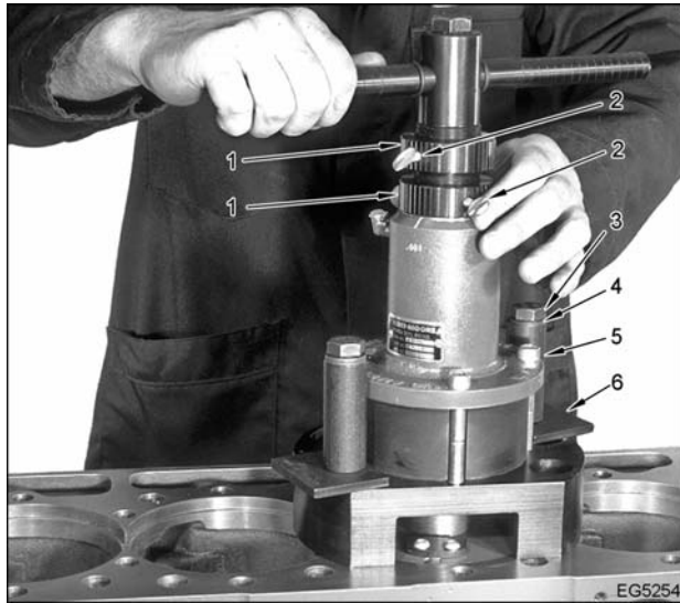
Figure 333 Positioning counterboring tool
