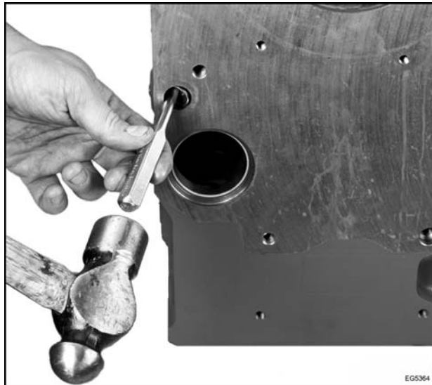
Figure 374 Removing crankcase plugs
