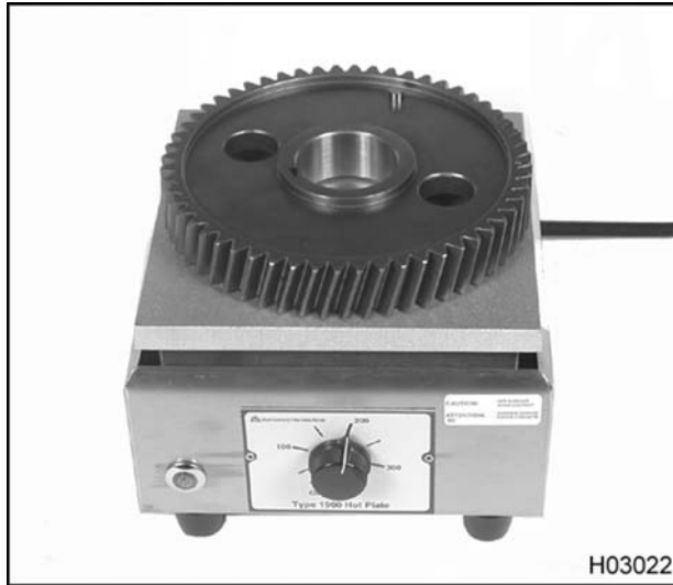
Figure 384 Heating the camshaft gear
