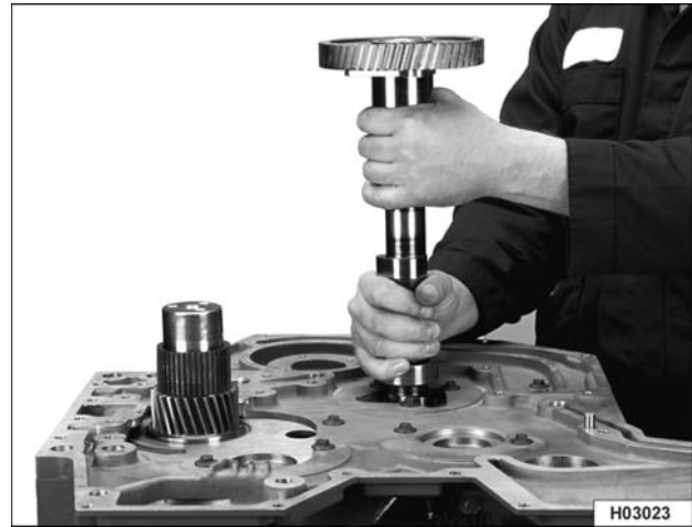
Figure 371 Removing the camshaft assembly
