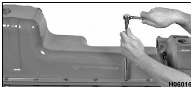
Figure 284 Removing the oil pan mounting bolts
