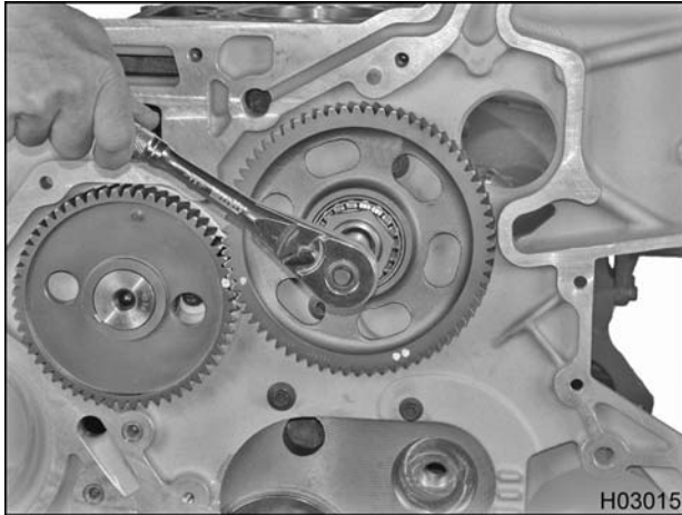
Figure 238 Removing the upper idler gear
