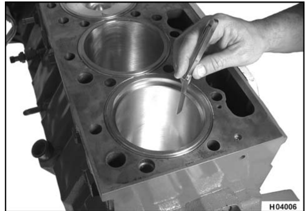
Figure 313 Checking piston ring end gap
