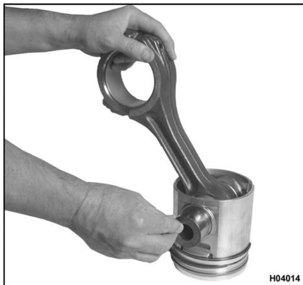
Figure 340 Installing piston pin
