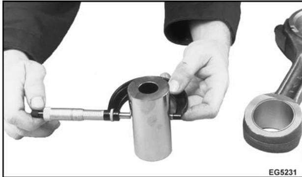
Figure 314 Measuring piston pin outside diameter
