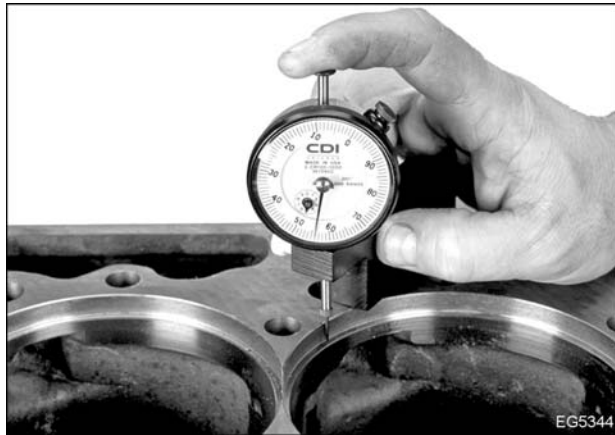
Figure 325 Checking counterbore depth with surface gauge
