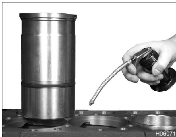
Figure 335 Lubrication of cylinder sleeve bore
