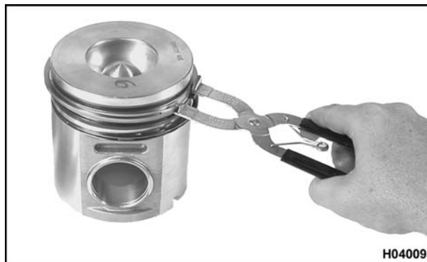
Figure 308 Removing piston rings (DT 466 piston shown)
