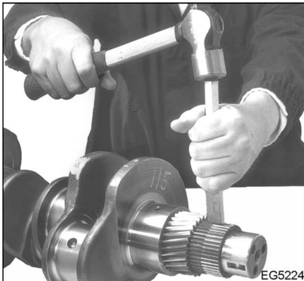
Figure 367 Removing oil pump drive spline
