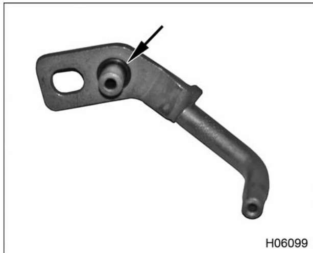
Figure 357 O-ring (underside) of new piston cooling tube
