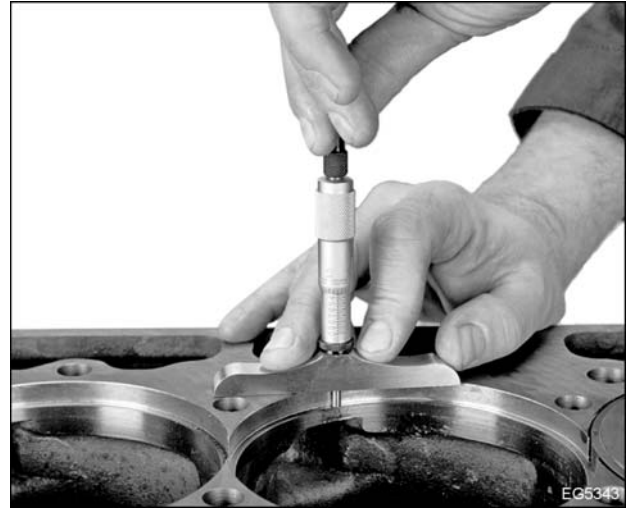
Figure 326 Checking counterbore depth with depth micrometer
