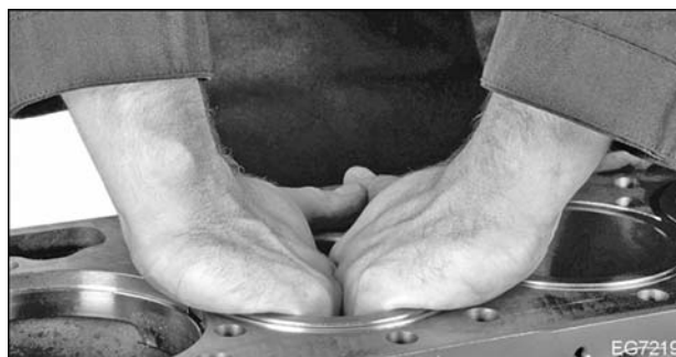
Figure 336 Installation of cylinder sleeve
