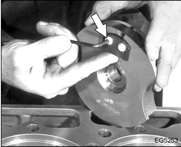
Figure 331 Setting tool bit
