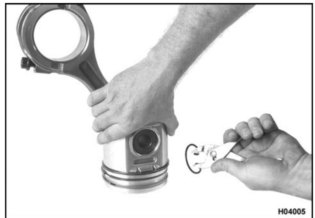
Figure 305 Removing piston pin retaining rings
