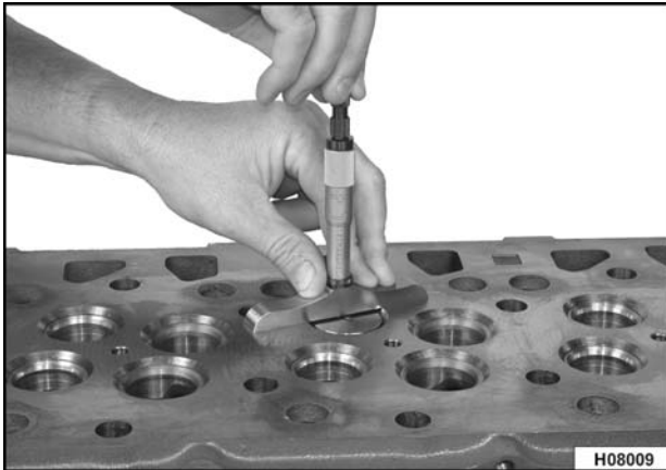
Figure 177 Checking valve recession
