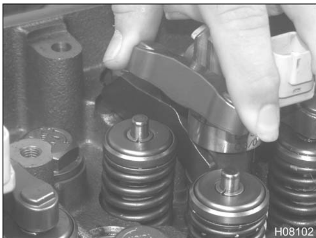
Figure 139 Removing the valve bridge
