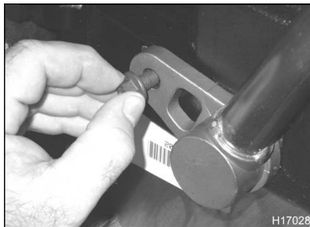
Figure 121 Installing the EGR return tube mounting bolt
