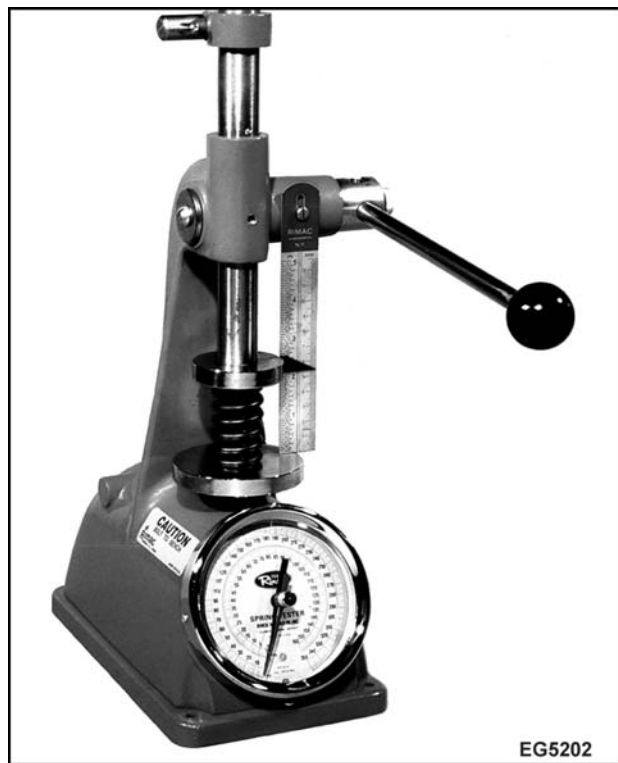
Figure 186 Measuring valve spring tension
