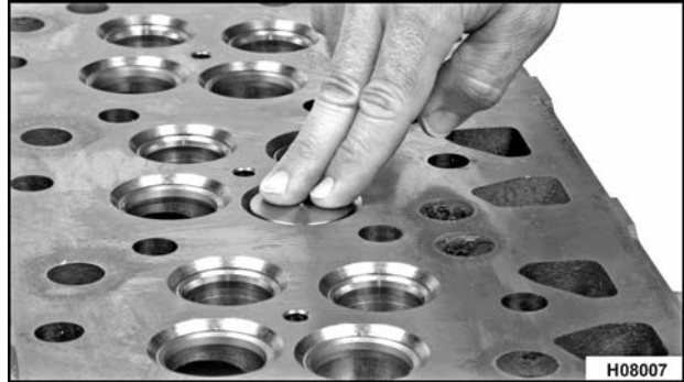
Figure 173 Turning valve on valve seat
