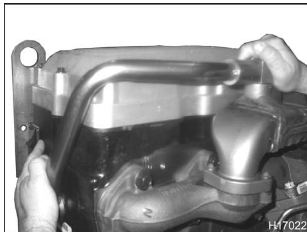
Figure 120 Installing the EGR cooler return tube
