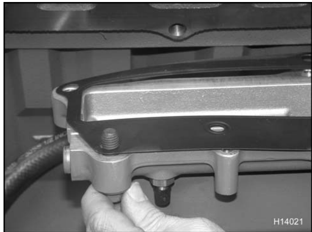
Figure 81 Aligning intake gasket to manifold
