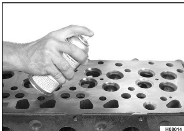
Figure 157 Spraying developer on cylinder head
