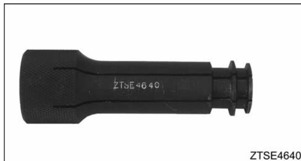
Figure 659 Valve seat remover (collet), ZTSE4640
