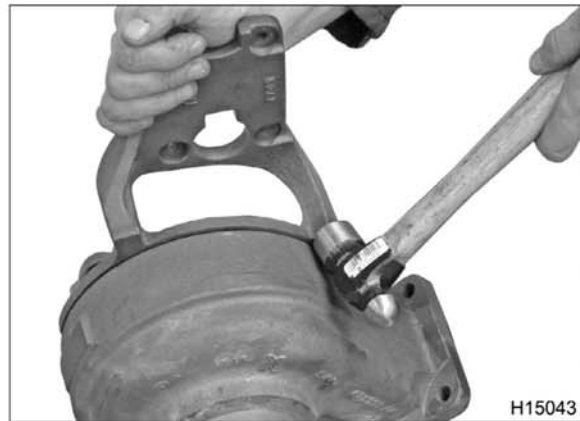
Figure 6 Removal of actuator flange
