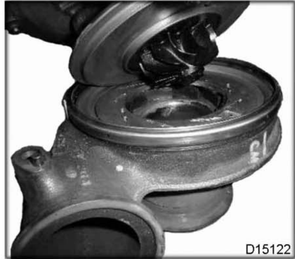
Figure 11 Center section onto the turbine housing
