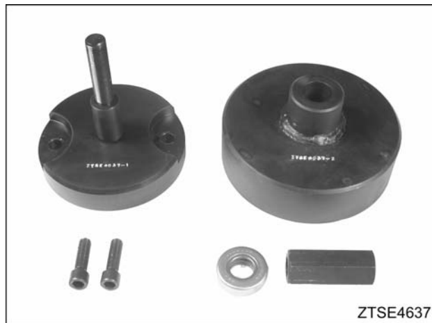
Figure 658 Rear seal installer, ZTSE4637
