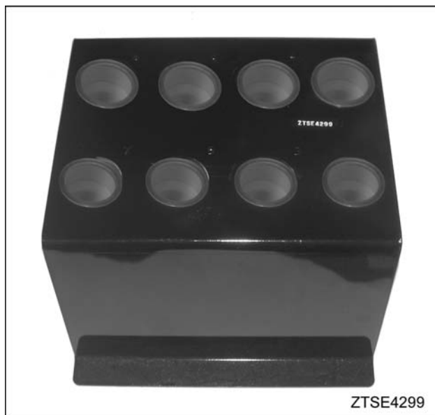
Figure 663 Injector rack – ZTSE4299B, Injector rack cups – ZTSE4645
