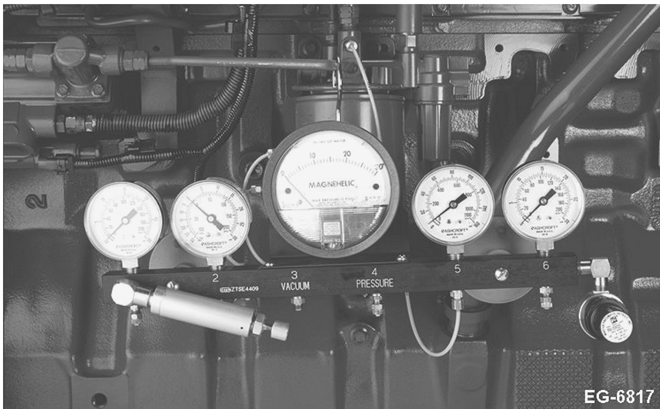
Figure 50 Measuring Fuel Pressure with Gauge Bar (PS94-831-3)
