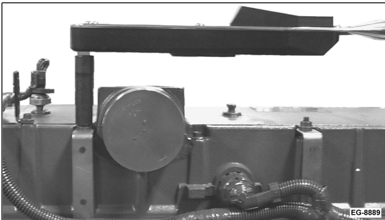
Figure 66 Torquing Valve Cover / Intake Manifold
