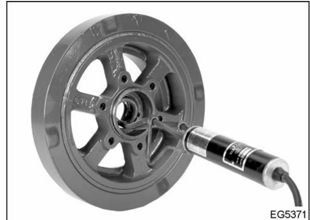
Figure 358 Heat vibration damper with Damper Heater
