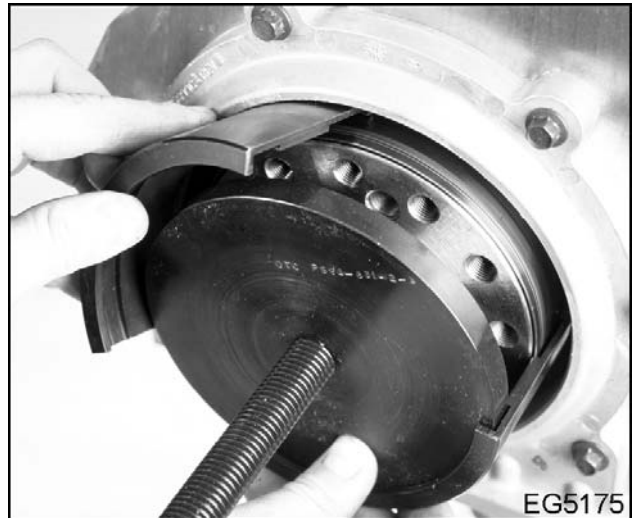
Figure 270 Assemble Wear Sleeve Removal Tool
