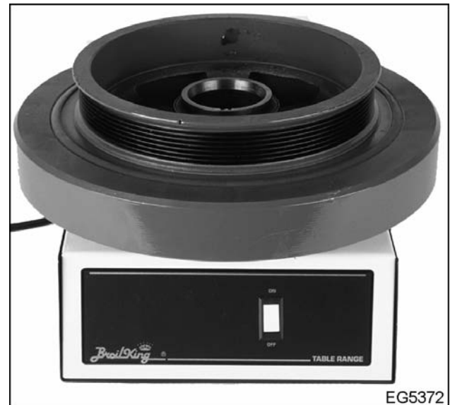
Figure 359 Heat vibration damper on hot plate
