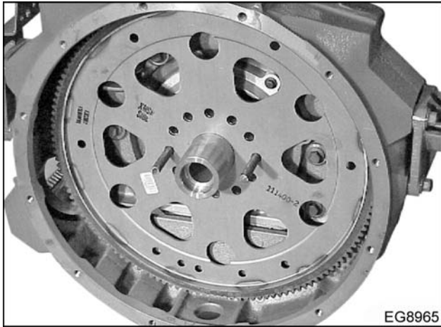
Figure 326 Install flywheel assembly
