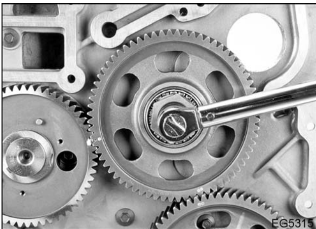
Figure 388 Install upper idler gear
