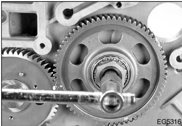
Figure 382 Remove upper idler gear
