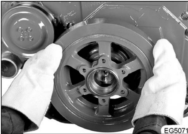
Figure 360 Install vibration damper
