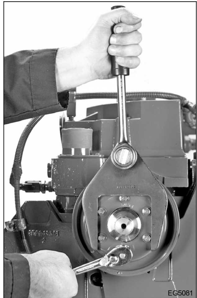
Figure 368 Remove fan drive hub pulley
