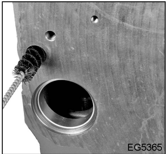
Figure 300 Clean crankcase galleries
