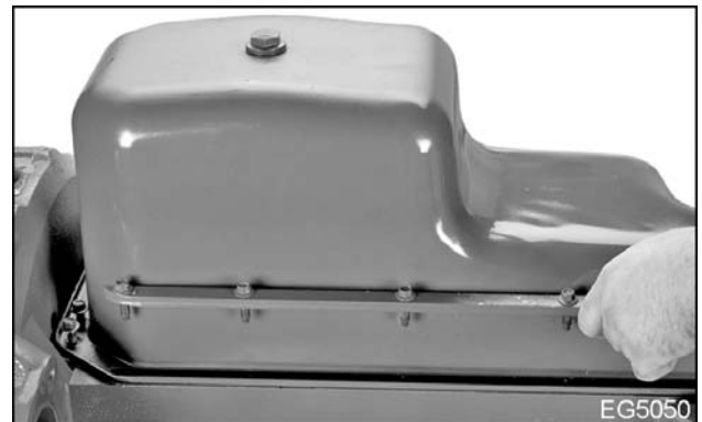
Figure 353 Install oil pan mounting bars
