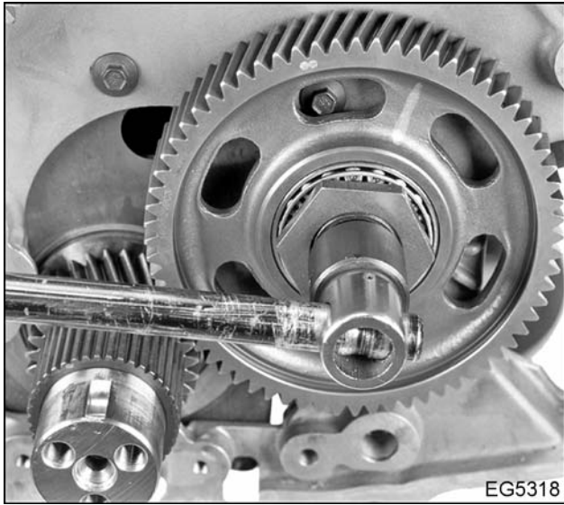
Figure 381 Remove lower idler gear
