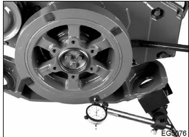
Figure 281 Measure vibration damper runout
