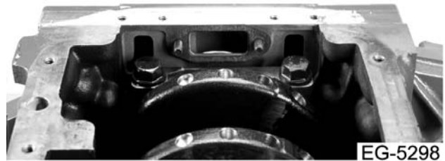
Figure 348 Install oil pickup tube gasket
