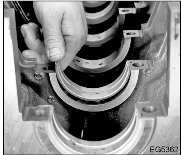
Figure 307 Install upper bearing inserts
