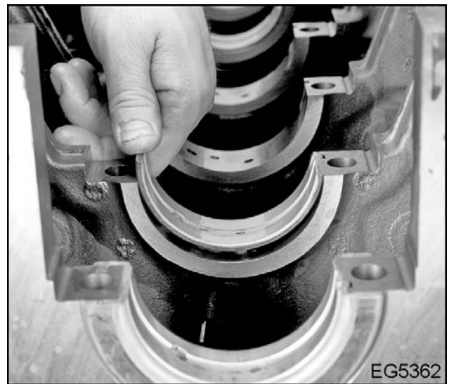
Figure 291 Remove upper main bearing shells
