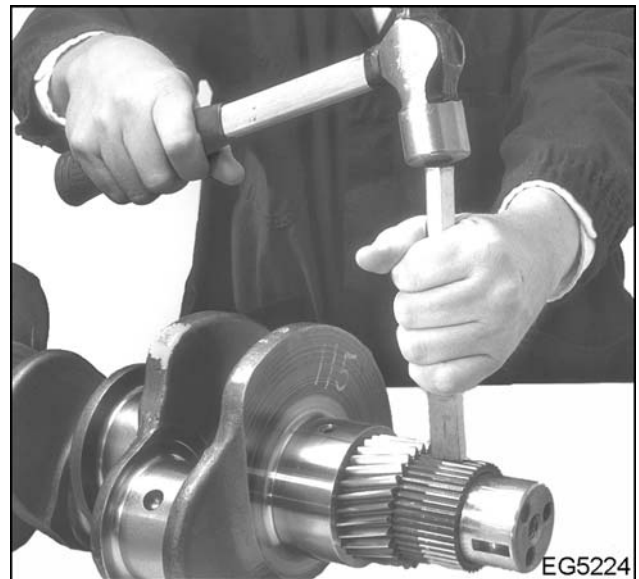
Figure 292 Remove oil pump drive spline
