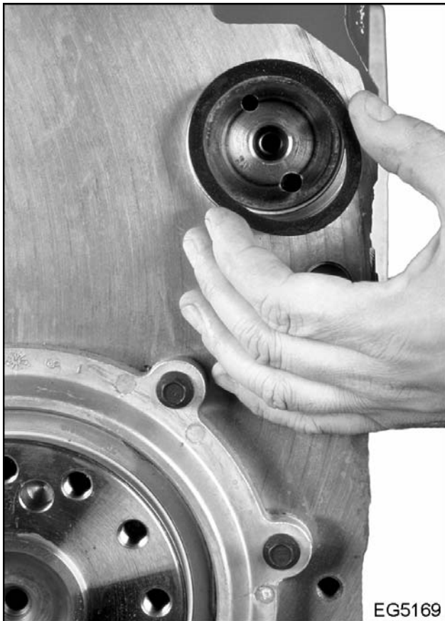
Figure 321 Install camshaft O-ring
