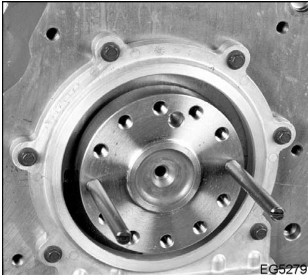
Figure 338 Install guide pins
