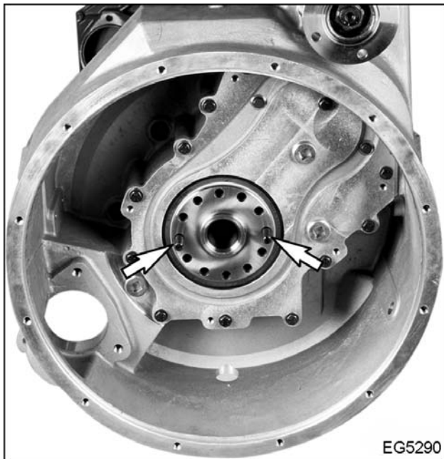
Figure 347 Install flywheel over guide pins
