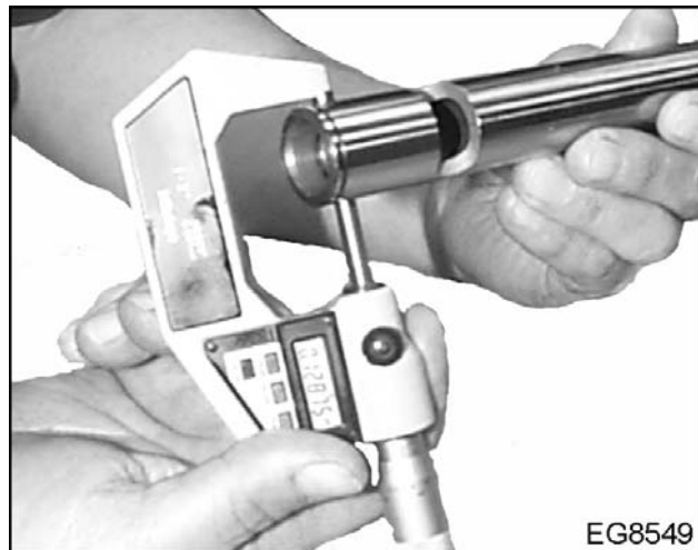
Figure 175 Measure contact and non-contact areas vertically
