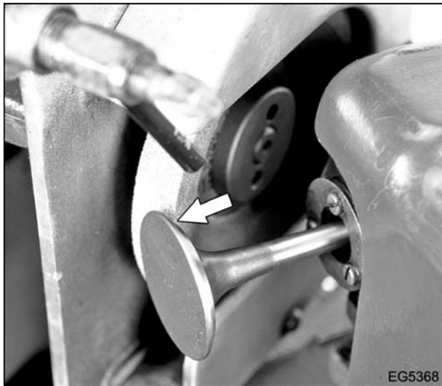
Figure 110 Grind valve face
