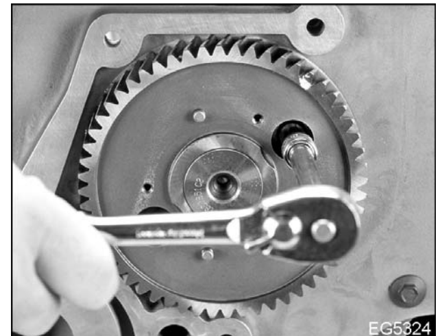
Figure 170 Remove camshaft gear thrust plate bolts
