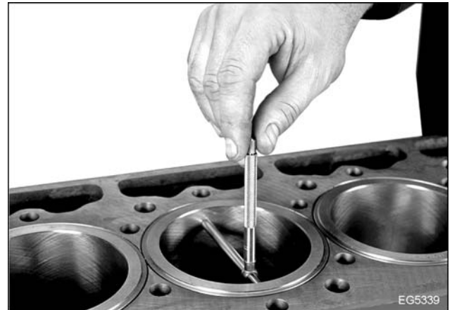
Figure 224 Measure cylinder sleeve inside diameter
