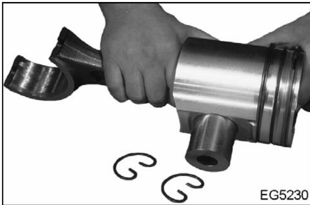
Figure 209 Remove piston pin
