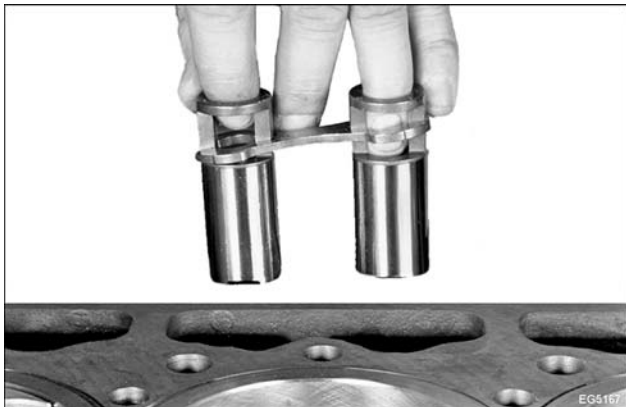
Figure 168 Remove roller tappet and guides
