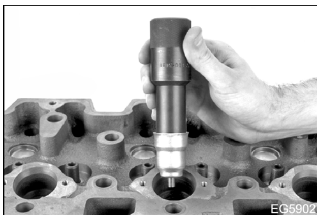
Figure 126 Insert fuel injector sleeve
