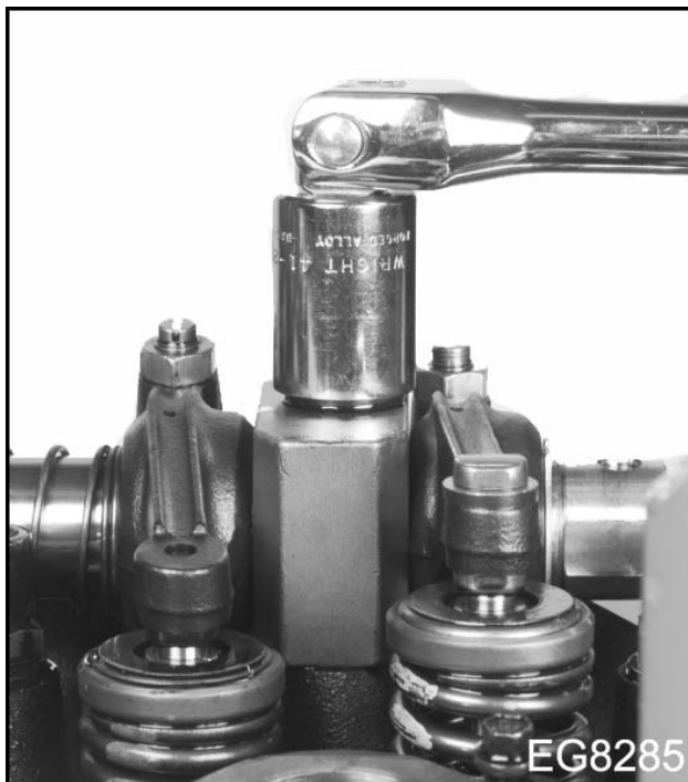
Figure 76 Remove valve lever assembly mounting bolts
