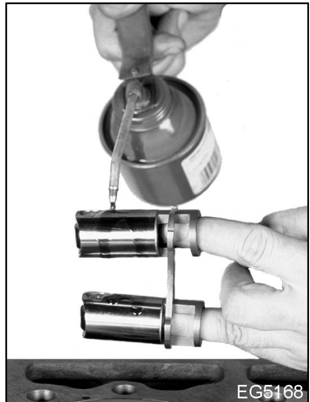
Figure 198 Lubricate roller tappets and guides
