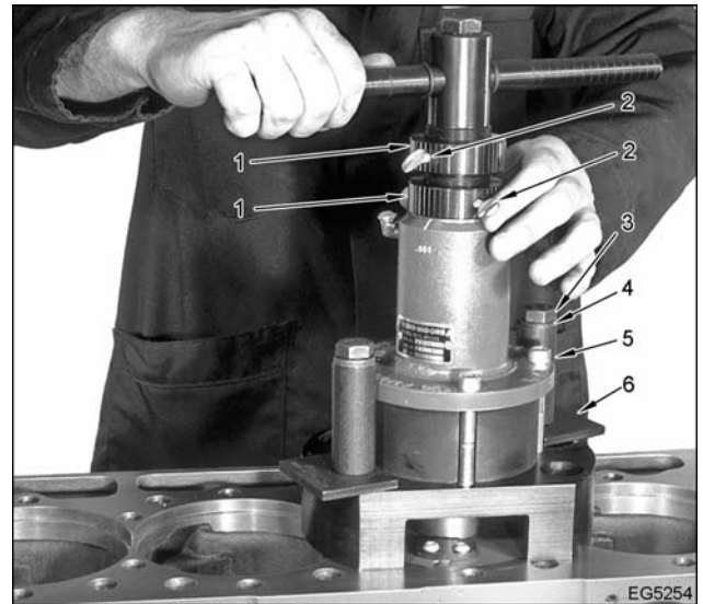
Figure 239 Position Counterbore Tool
