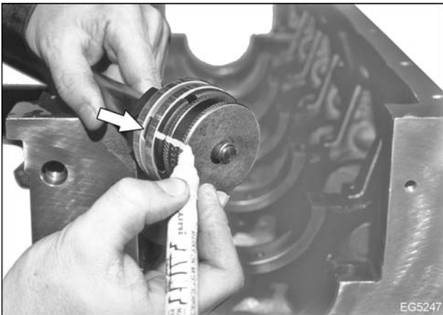
Figure 194 Mark oil hole location
