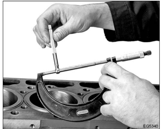
Figure 225 Measure cylinder sleeve inside diameter
