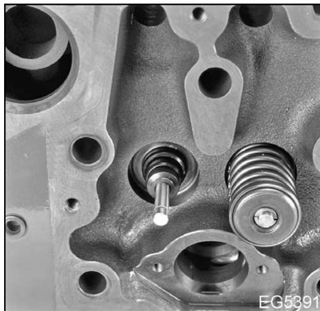
Figure 130 Install valve stem seal assembly
