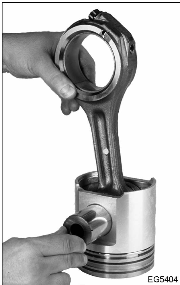
Figure 248 Insert piston pin
