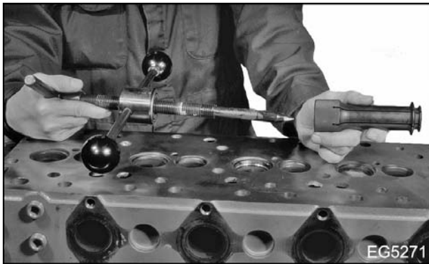
Figure 115 Assemble collet on tool
