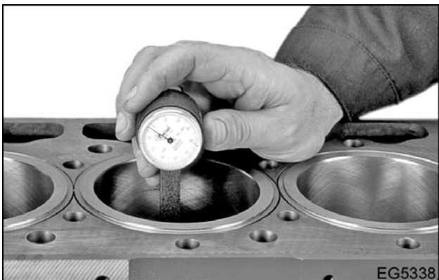
Figure 227 Measure cylinder sleeve lower diameter
