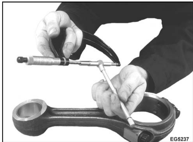
Figure 222 Measure connecting rod bearing bore taper
