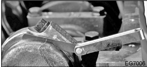
Figure 236 Measure connecting rod side clearance
