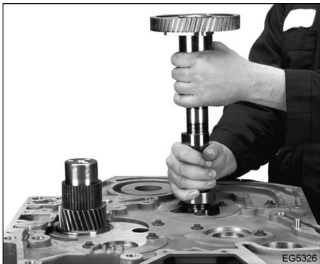
Figure 171 Remove camshaft and gear
