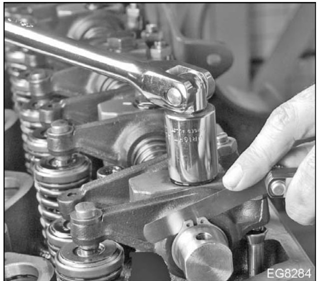
Figure 139 Tighten valve lever assembly mounting bolts
