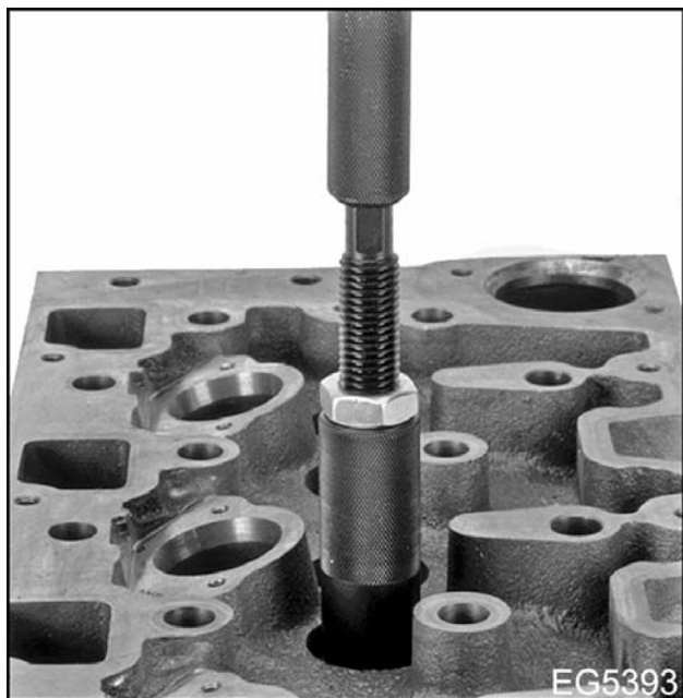
Figure 129 Install valve guide
