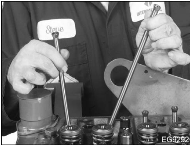
Figure 137 Install push rods
