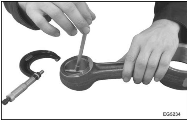
Figure 220 Measure connecting rod piston pin bore
