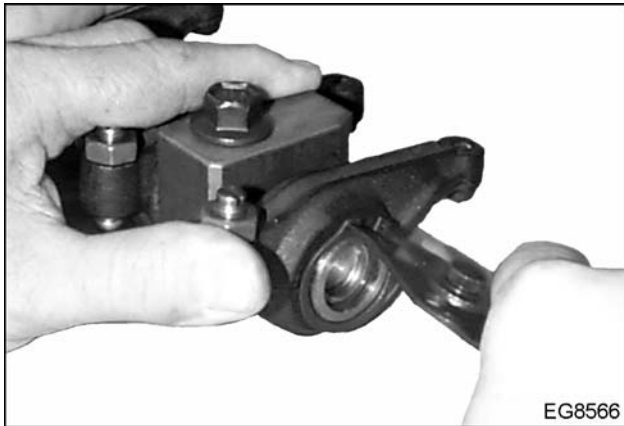
Figure 191 Install valve lever shaft retaining ring
