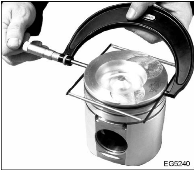
Figure 213 Measure piston diameter
