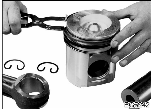
Figure 211 Remove piston rings
