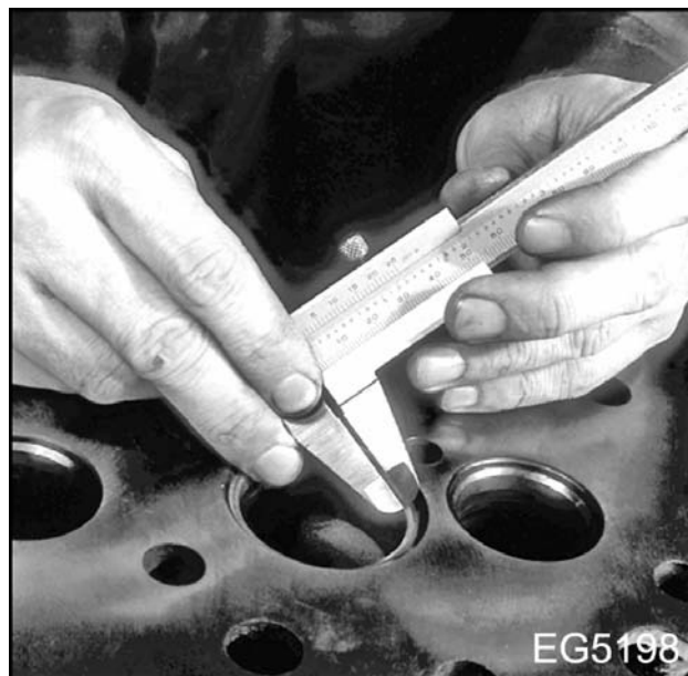
Figure 103 Measure valve seat width
