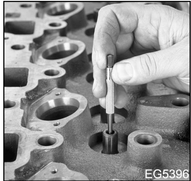
Figure 98 Measure valve guide with small hole gauge
