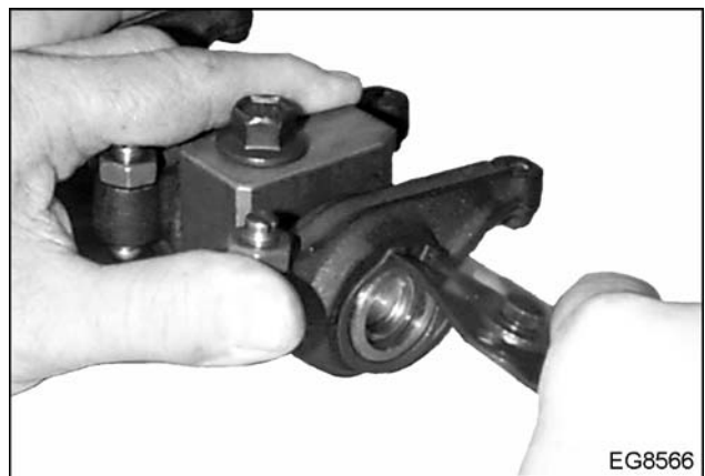
Figure 186 Remove valve lever retaining ring
