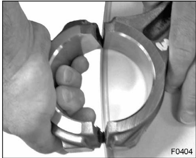
Figure 206 Split fractured connecting rod
