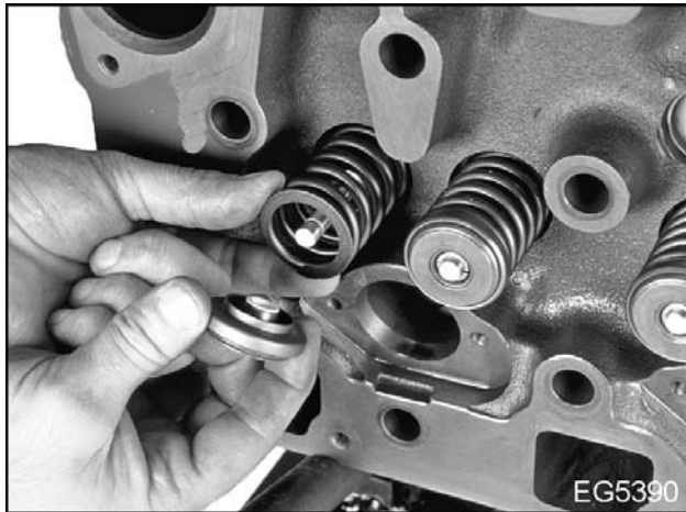
Figure 132 Install rotator assembly
