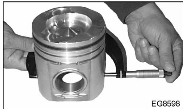
Figure 215 Measure piston skirt diameter
