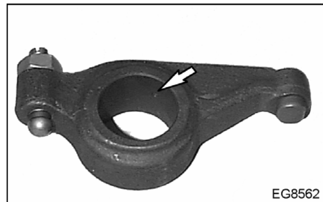
Figure 178 Inspect valve lever oil hole
