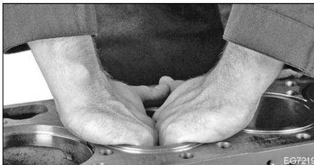
Figure 245 Install cylinder sleeve
