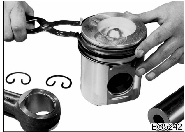
Figure 247 Install piston rings
