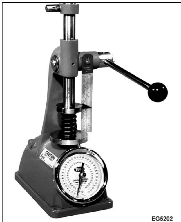
Figure 108 Measure valve spring tension
