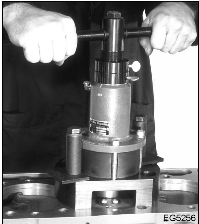
Figure 241 Cut cylinder sleeve counterbore
