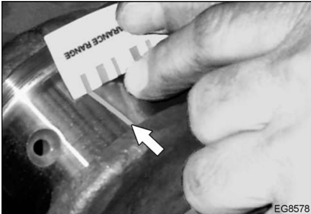
Figure 235 Measure flattened plastic material
