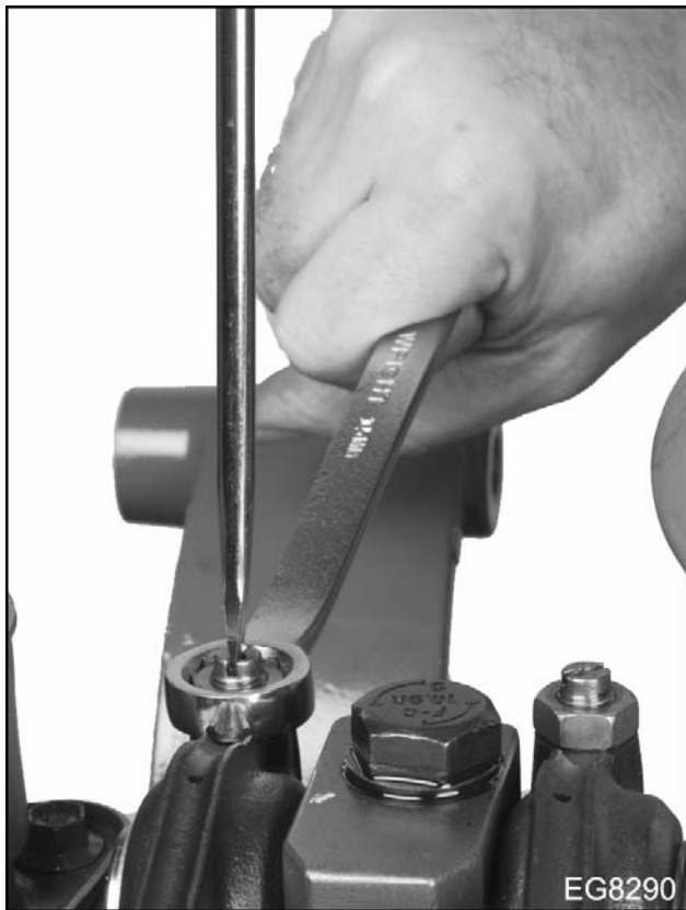
Figure 75 Loosen valve lever adjusting screw nuts
