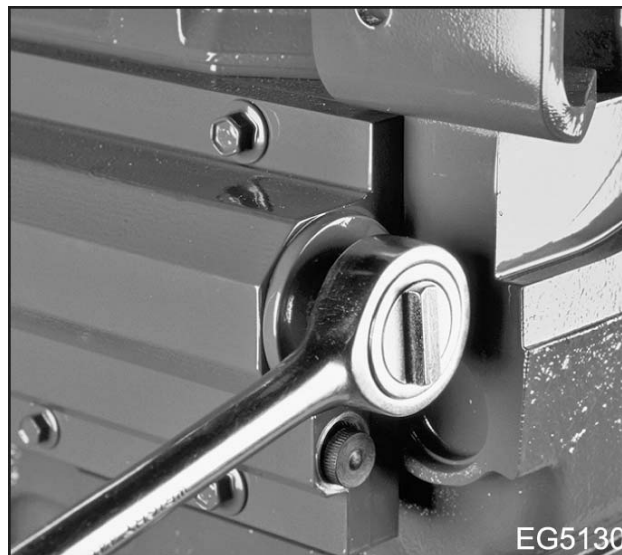
Figure 68 Remove supply manifold end plug
