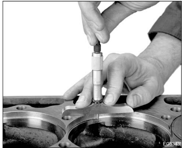
Figure 230 Measure cylinder sleeve counterbore depth
