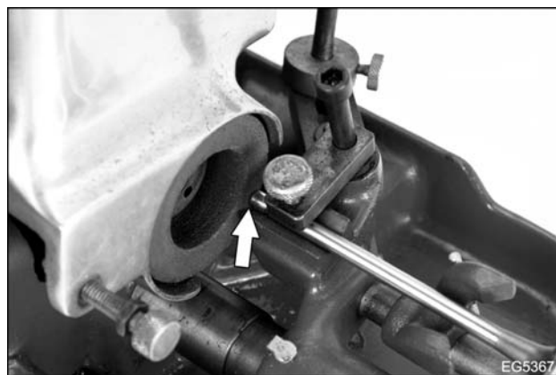
Figure 112 Insert valve stem in grinder
