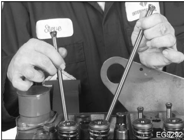
Figure 78 Remove push rods
