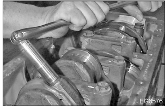
Figure 200 Remove connecting rod bolts
