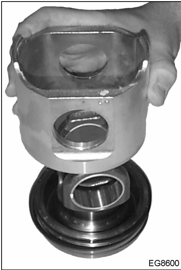
Figure 246 Assemble two-piece piston (parts are upside down for assembling)
