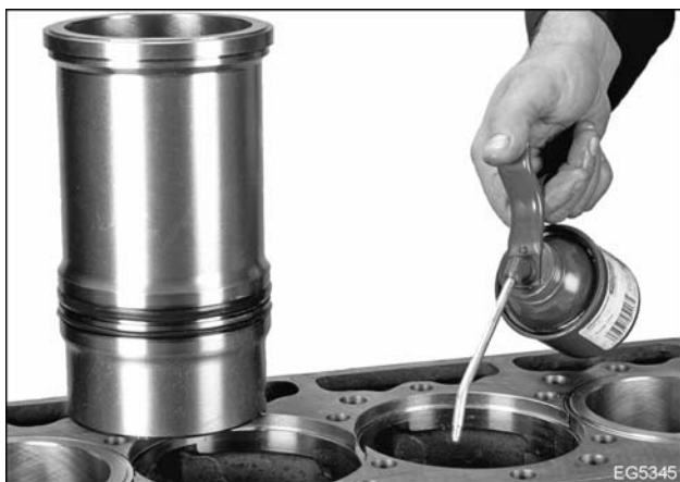
Figure 244 Lubricate cylinder sleeve bore
