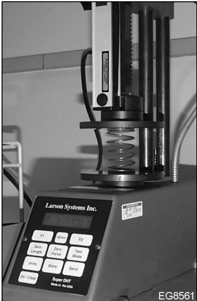
Figure 180 Measure shaft spring tension
