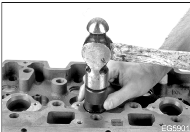
Figure 127 Install fuel injector sleeve
