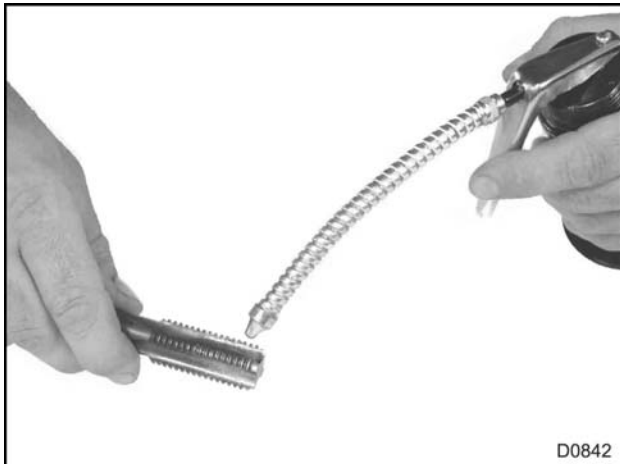
Figure 119 Lubricate thread tap
