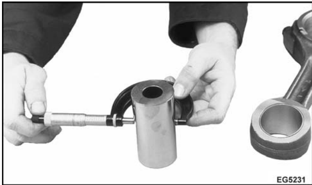
Figure 223 Measure piston pin outside diameter
