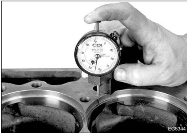
Figure 229 Measure cylinder sleeve counterbore depth
