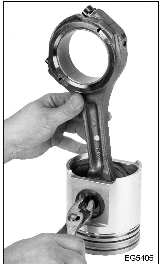
Figure 208 Remove piston pin retaining rings
