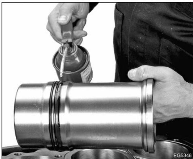
Figure 243 Lubricate cylinder sleeve and rings
