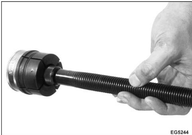
Figure 193 Install bushing on collet
