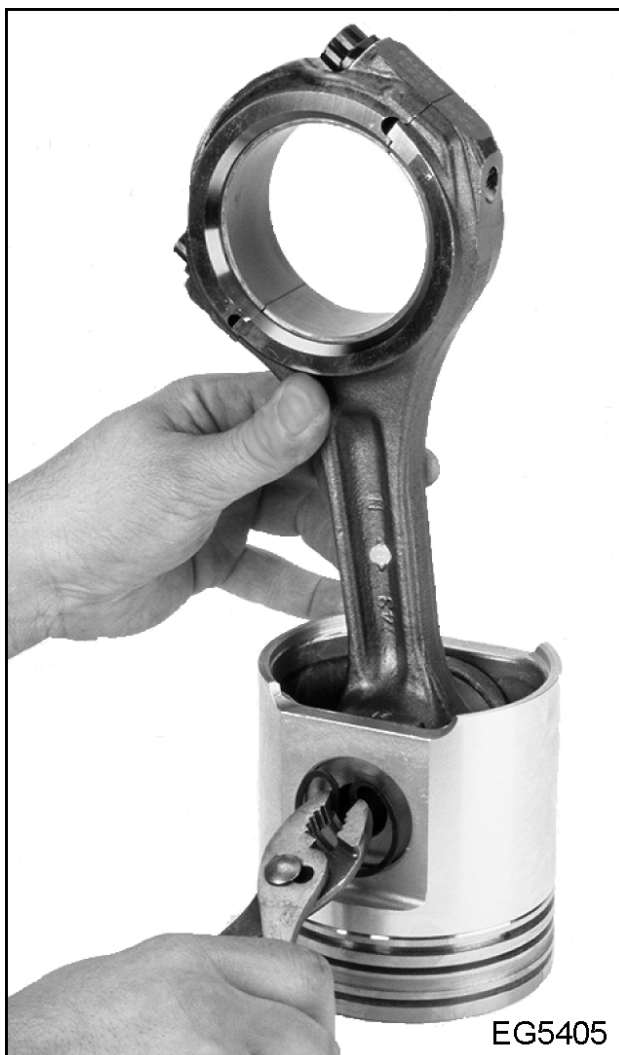
Figure 249 Install piston pin retaining ring
