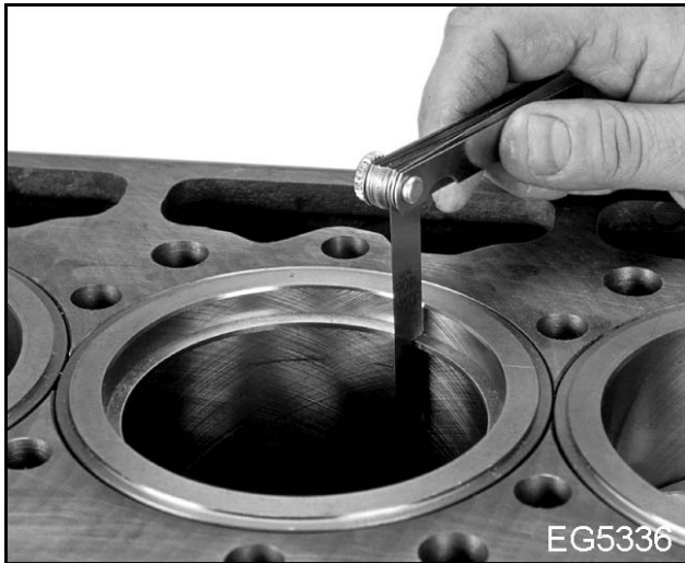
Figure 216 Measure ring gap
