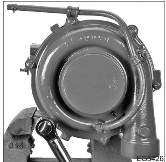
Figure 45 Install compressor housing
