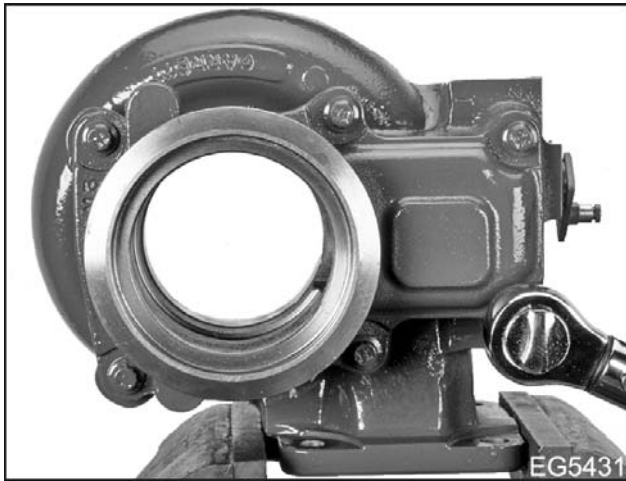
Figure 43 Install wastegate housing
