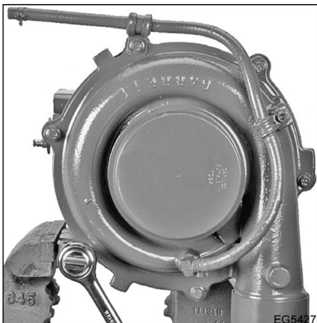
Figure 36 Remove compressor housing
