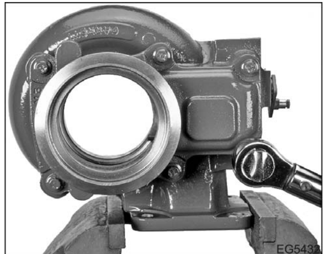
Figure 40 Remove wastegate housing
