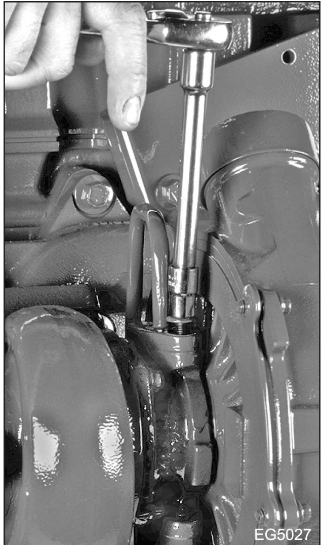
Figure 47 Install oil feed tube
